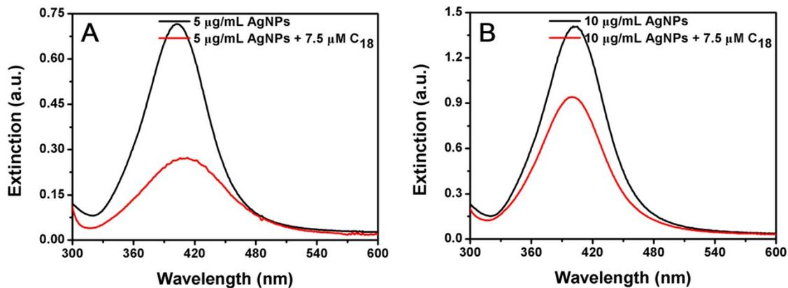
**Figure S4.** UV-vis spectra of 20 nm AgNPs with an initial concentration of (A) 5  $\mu\text{g/mL}$ ; and (B) 10  $\mu\text{g/mL}$  before and after incubated with 7.5  $\mu\text{M}$  of  $\text{C}_{18}$  DNA at 37  $^{\circ}\text{C}$  for 1.5 h. In (A) the spectrum red shifted indicating ripening, while in (B) the spectra blue shifted indicating etching of the AgNPs. Therefore, the critical concentration for ripening to take place is a function of the initial concentration of AgNPs.
