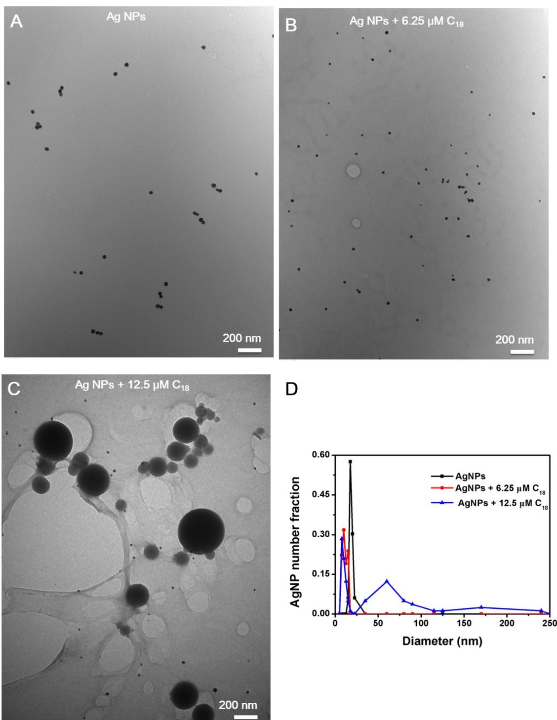
**Figure S1.** Wide-area TEM micrographs of 20 nm AgNPs incubated with different concentrations of C<sub>18</sub> DNA: (A) no DNA; (B) 6.25  $\mu\text{M}$  C<sub>18</sub> DNA; and (C) 12.5  $\mu\text{M}$  C<sub>18</sub> DNA for 1.5 h at 37 °C. (D) Histogram of the particle size distribution from the TEM data.
