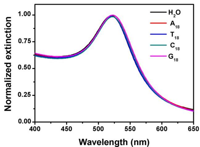
**Figure S7.** UV-vis spectra of citrate-capped gold nanoparticles (AuNPs) of 15 nm before and after adding 18-mer homo-DNAs of 25  $\mu$ M for 1.5 h at 37  $^{\circ}$ C. Negligible changes in the spectrum were observed for all these samples indicating that the AuNPs cannot be etched by these DNAs.
