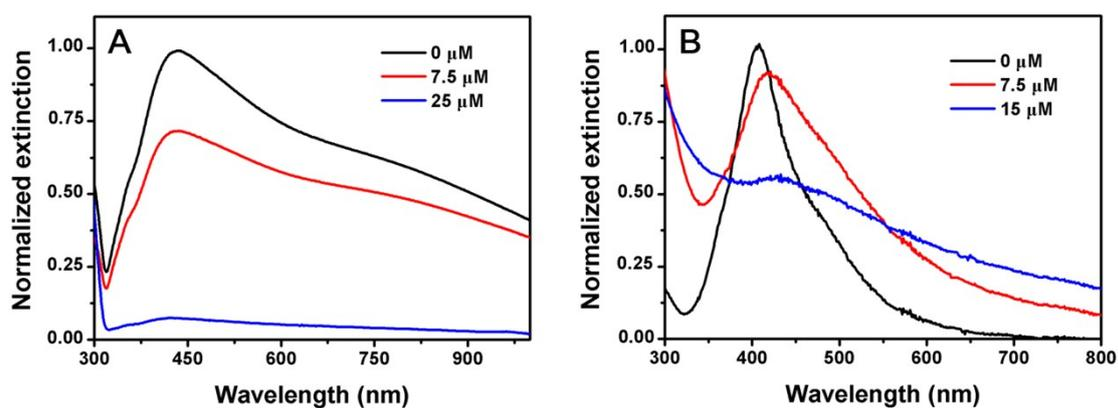
**Figure S6.** UV-vis spectra of (A) PVP- and (B) CTAB-capped AgNPs (20.25  $\mu\text{g/mL}$ ) mixed with different concentrations of C<sub>18</sub> DNA. In (A) the UV-vis peak dropped and blue shifted indicating etching, while in (B) the spectra red shifted indicating aggregation of the AgNPs.
