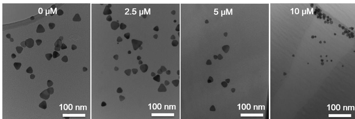
**Figure S8.** Wide-area TEM micrographs of Ag nanoplates before and after mixing with different concentrations of C<sub>18</sub> DNA. The increase of the C<sub>18</sub> DNA concentration caused an initial decrease in size of the triangular nanoplates and subsequent conversion to spherical morphology.
