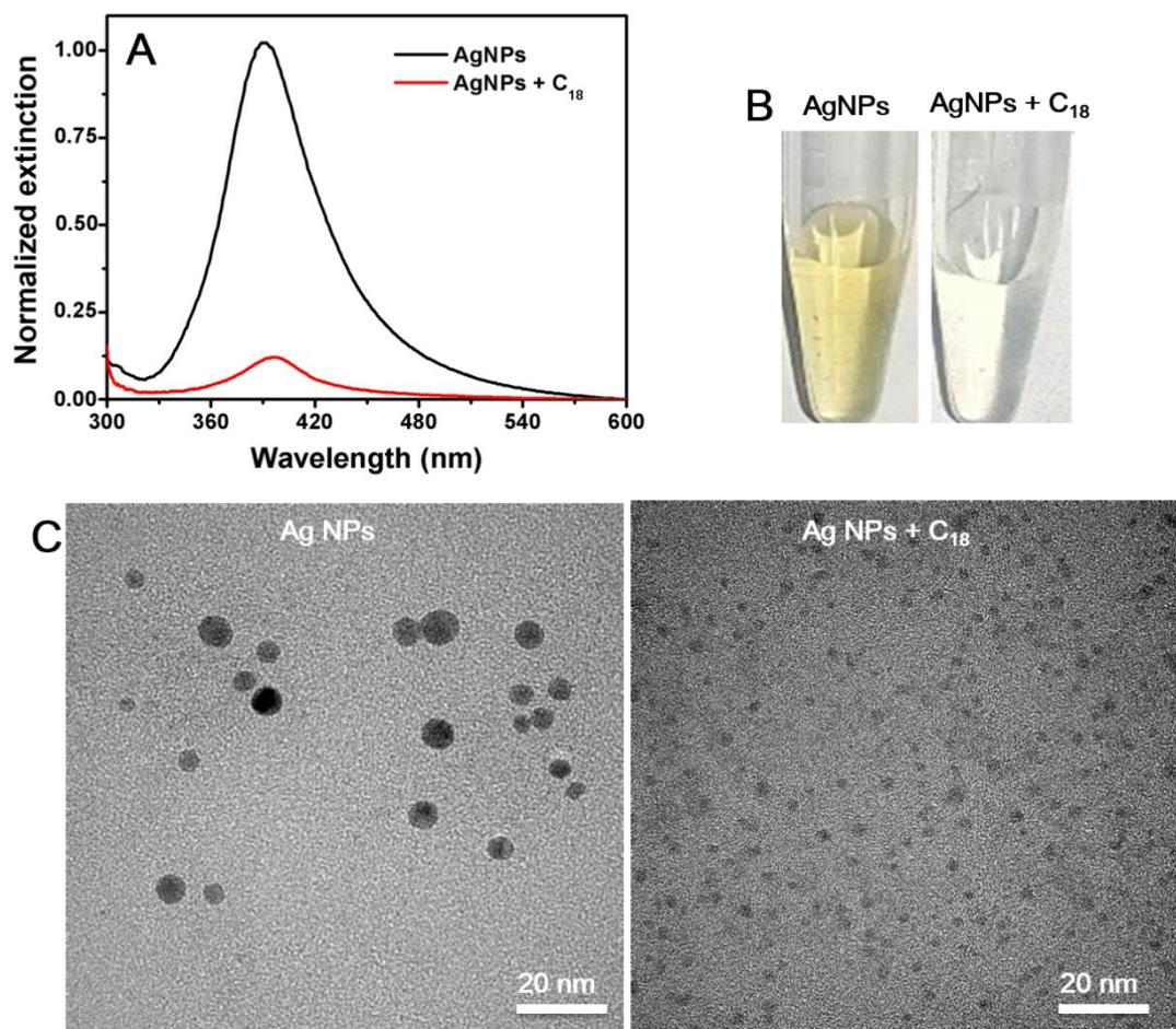
**Figure S5.** (A) UV-vis spectra and (B) photographs of home-made AgNPs (20.25  $\mu\text{g/mL}$ ) before and after incubated with 25  $\mu\text{M}$  C<sub>18</sub> DNA. The disappearance of the yellow color and the drop of the plasmonic peak intensity were indications of etching. (C) TEM micrographs of the AgNPs before and after mixing with 25  $\mu\text{M}$  C<sub>18</sub> DNA.
