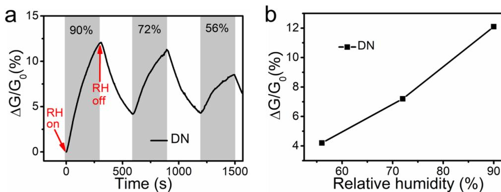
**Figure S5.** a) Real-time response of the unmodified DN hydrogel to different RH levels ranging from 90% to 56%. b) Plot of the quantitative response of the DN hydrogel sensor versus RH.
