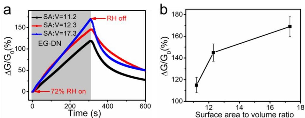
**Figure S8.** Investigation of the effect of surface-area-to-volume ratio (SA:V) on the sensitivity. a) Dynamic responses of the three EG-DN sensors with the SA:V of 11.2, 12.3 and 17.3, respectively, to 72% RH. b) Plot of the quantitative response to 72% RH versus the SA:V of the EG-DN organohydrogels. The cuboid-shaped EG-DN slices with the SA:V of 11.2, 12.3 and 17.3 have the dimensions of 2 cm × 6 cm × 0.2 cm, 1 cm × 6 cm × 0.2 cm, 0.5 cm × 6 cm × 0.2 cm, respectively.
