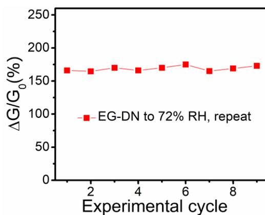
**Figure S9.** Plot of the quantitative responses of the EG-DN sensor to 72% RH versus experimental cycle.
