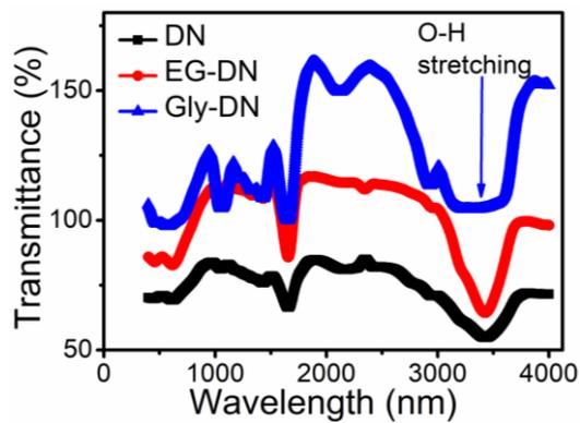
**Figure S4.** Fourier transform infrared (FTIR) spectra of the DN hydrogel, EG-DN and Gly-DN organohydrogels, respectively.
