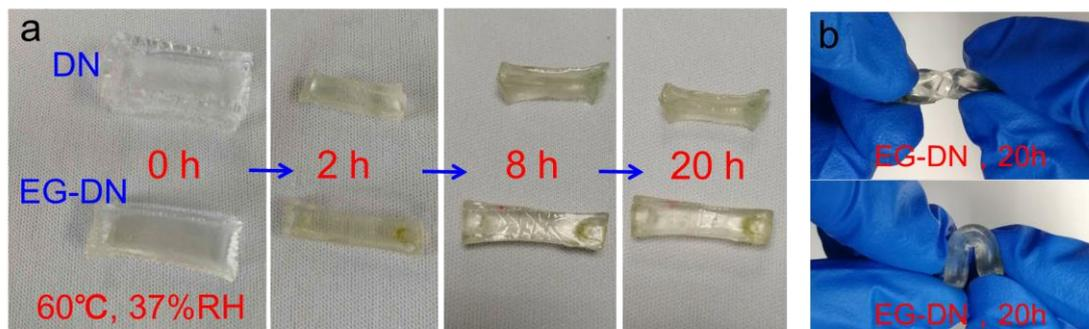
**Figure S1.** a) Photographs of the DN hydrogel (above) and EG-DN organohydrogel (below) placed at 60 °C and 37% relative humidity (RH) for 0, 2, 8 and 20 h, respectively. b) Digital images showing that the EG-DN organohydrogel stored at 60 °C and 37% RH for 20 h can still be twisted for 360° (above) and bent for 155° (below). In contrast, the DN hydrogel became dried at 20 h and therefore could not withstand such mechanical deformations.
