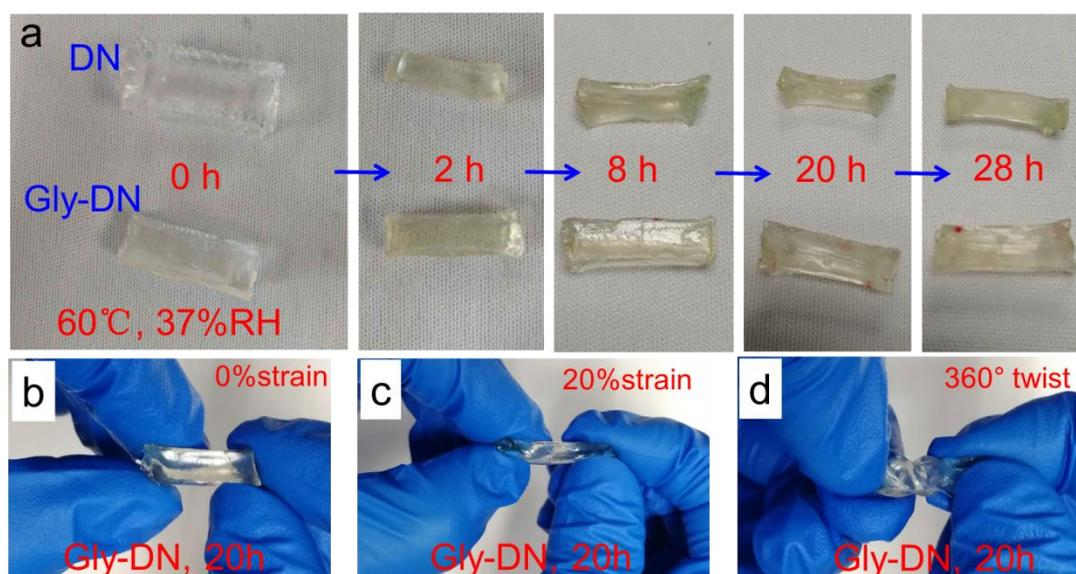
**Figure S2.** a) Photographs of the DN hydrogel (above) and Gly-DN organohydrogel (below) stored at 60 °C and 37% RH for 0, 2, 8, 20 and 28 h, respectively. b-d) Photographs showing that the Gly-DN organohydrogel stored at 60 °C and 37% RH for 50 h can still be stretched for 20% strain (b-c) and twisted for 360° (d).
