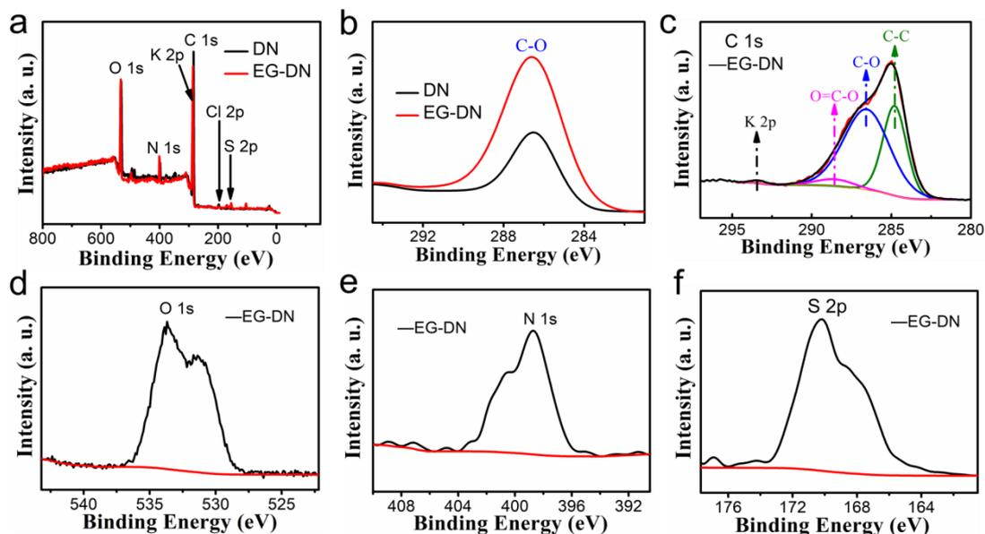
**Figure S3.** a) X-ray photoelectron spectroscopy (XPS) spectra of the DN hydrogel and EG-DN organohydrogels. b) Analysis of the C-O bond in the C 1s XPS spectra of the DN hydrogel and EG-DN organohydrogels. c) C 1s XPS spectra of the EG-DN organohydrogel. d), e) and f) O 1s, N 1s and S 2p XPS spectra of the EG-DN organohydrogel, respectively.
