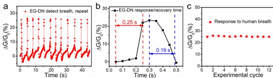
**Figure S6.** a) Dynamic response of the EG-DN sensor to human respiration for twelve repeated cycles. b) Analyses of the response and recovery time of the EG-DN sensor in the respiration monitoring. c) Plot of the response variation of the EG-DN sensor versus experimental cycle.
