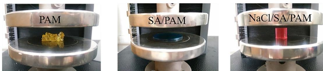
**Figure S10** When compressed with 98% of their original heights, the PAM gel was fractured completely, while SA/PAM gel could not be restored to its original state though without fracture. In contrast, NaCl/SA/PAM hydrogel recovered to its original shape immediately after release of the loading even at 98% strain.
