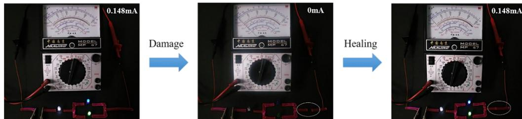
**Figure S3** The photographs of the healing process for ionic hydrogels in series-parallel as self-healable electronic interconnects with LEDs. The LEDs could work and the multimeter shows the same value of current to initial stage after the two cut pieces are pushed together at room temperature and spontaneously self-adhesive under ambient conditions without any external stimulus, indicating the good healing properties of the ionic hydrogels for electronic circuits.
