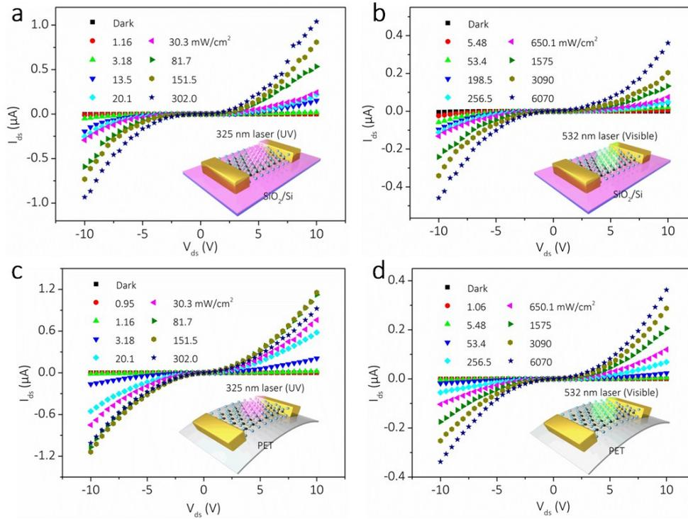
Figure S4. (a-b) I-V curves of MoS<sub>2</sub>/SiO<sub>2</sub>/Si PD under UV and VIS illumination, respectively. (c-d) I-V curves of MoS<sub>2</sub>/PET PD under UV and VIS illumination, respectively.
