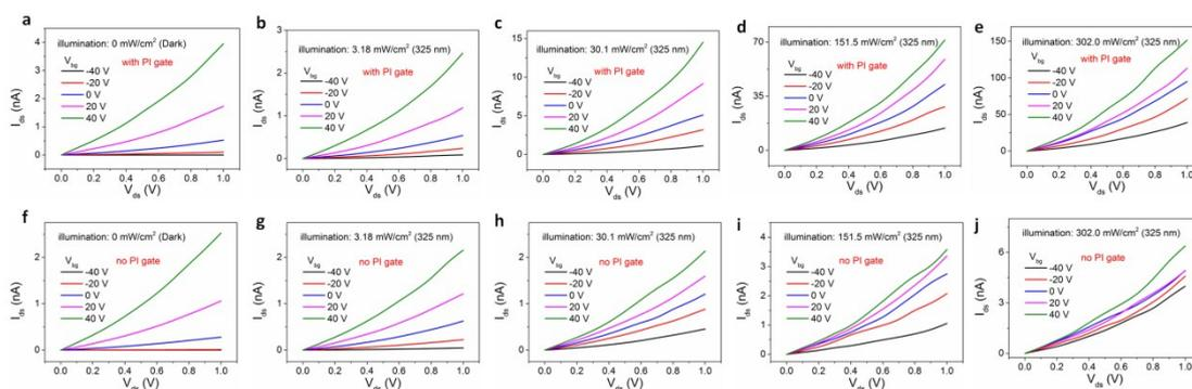
Figure S7.  $I_{ds}$ - $V_{ds}$  output characteristics of monolayer MoS<sub>2</sub> FET (a-e) with PI gate and (f-j) without PI gate in dark and different UV optical power intensity.
