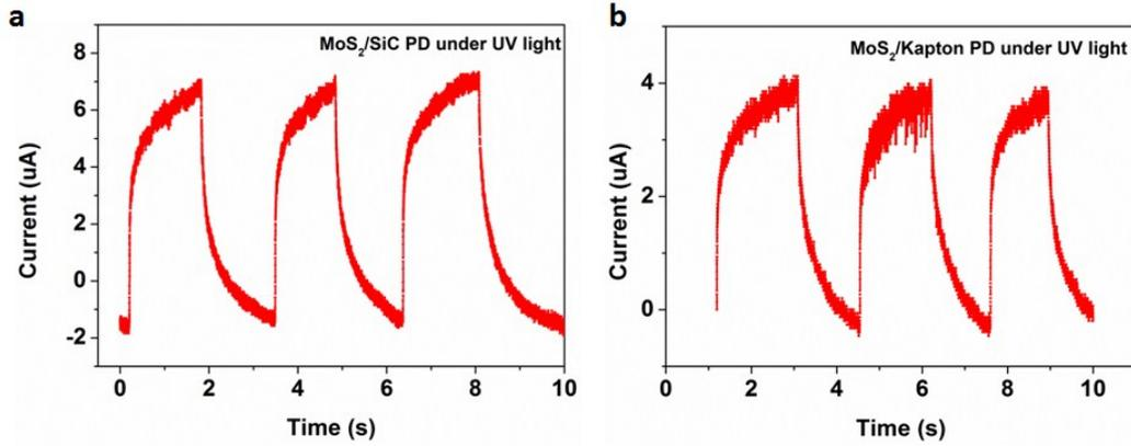
Figure S8. The transient response of (a) MoS<sub>2</sub>/SiC PD and (b) MoS<sub>2</sub>/Kapton PD.
