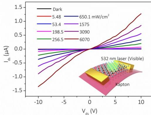
Figure S5. I-V curves of MoS<sub>2</sub>/Kapton PD under VIS (532 nm laser) illumination.
