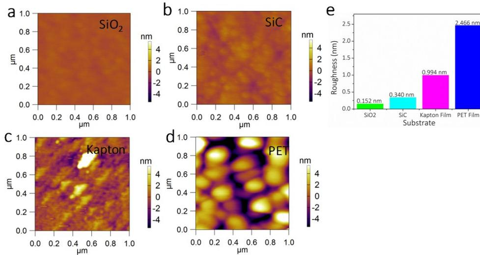
Figure S2. (a-d) Surface morphologies of SiO<sub>2</sub>/Si, SiC, Kapton and PET, respectively. (e) Surface roughness of four substrates.
