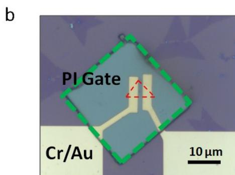
Figure S6. (a) The construction processes of MoS<sub>2</sub>-FET with a layer of PI coating. (b) Optical microscope image of MoS<sub>2</sub>-FET with PI gate.
