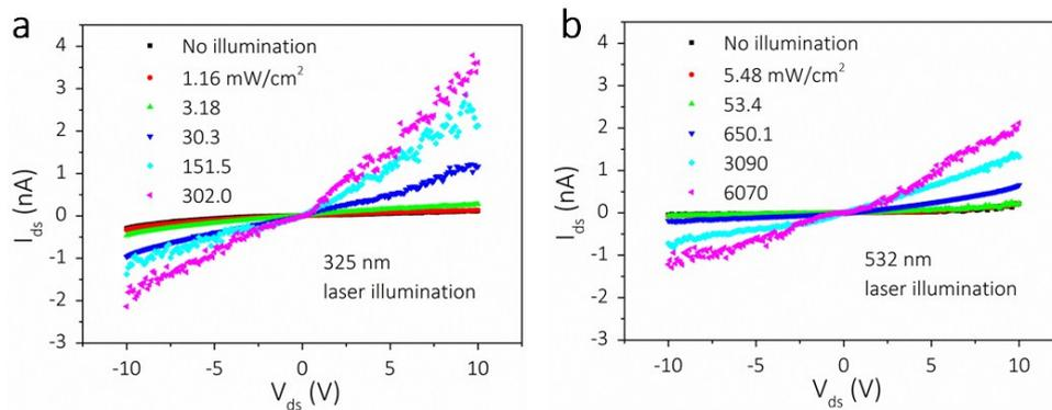
Figure S3. (a) In-plane current of undoped-SiC substrate itself under UV illumination. (b) In-plane current of undoped-SiC substrate itself under VIS illumination.
