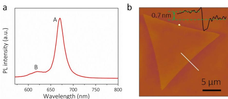
Figure S1. (a) Typical PL spectrum of monolayer MoS<sub>2</sub>. (b) AFM morphology measurement of triangle MoS<sub>2</sub> flake. The thickness is ~0.7 nm.
