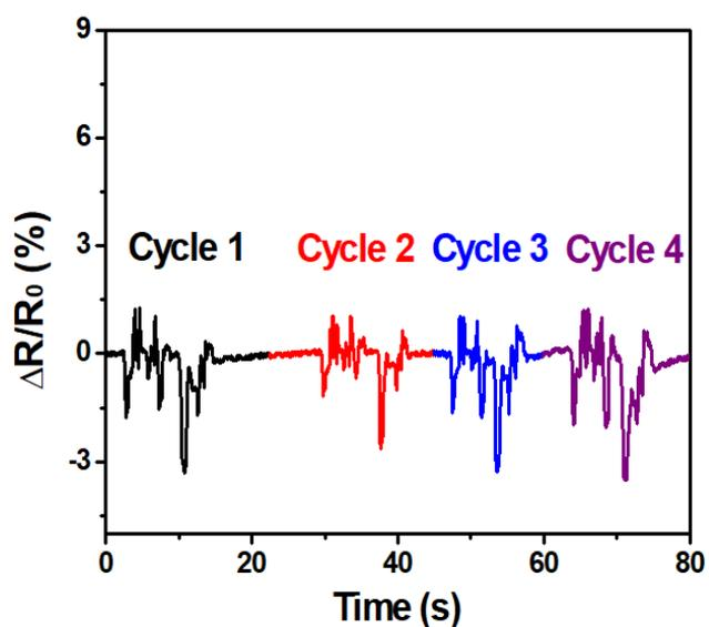
**Figure S13.** Resistive change of LM-hydrogel (10 vol%) for repeated cycles of writing letters “A”, “B”, “C” and “D”.
