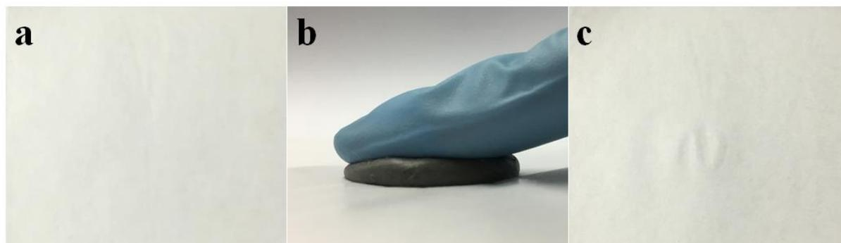
**Figure S21.** Photo of leaking test for LM-hydrogel (10 vol%) a) A piece of clean paper. b) Pressed LM-hydrogel on paper. c) The paper was only slightly wetted by the hydrogel without leaking of liquid metal.
