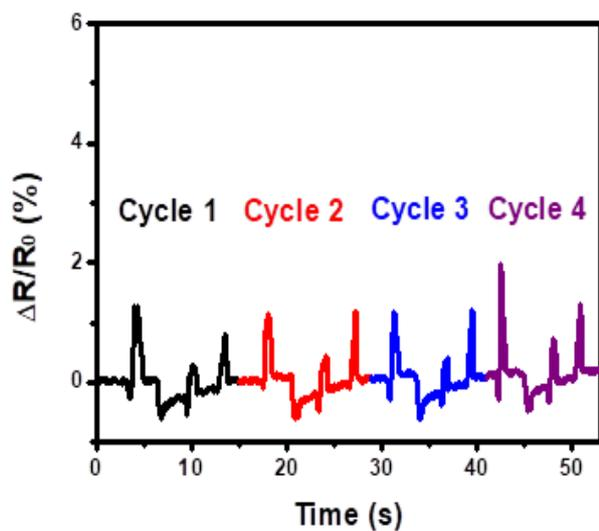
**Figure S12.** Resistive change for repeated cycles of continuous movement on LM-hydrogel (10 vol%) surface in **Figure 4g**.
