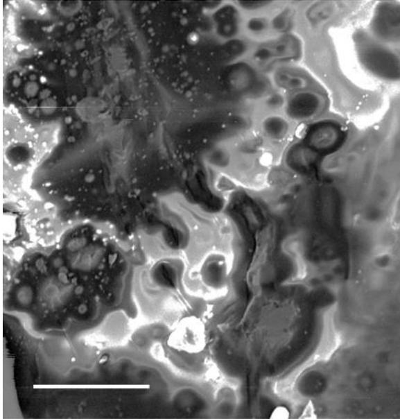
**Figure S3.** Cross-sectional SEM images for hydrogels with 20 vol% liquid metals. Heavy aggregation was observed in the matrix. Scale bar: 25  $\mu\text{m}$ .
