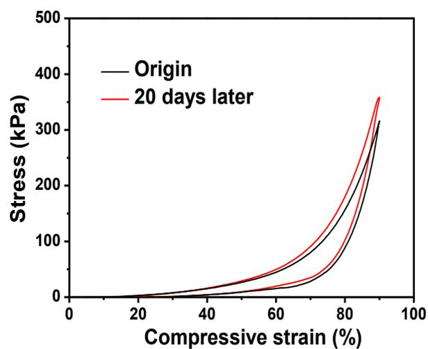
**Figure S20.** Compressive test for LM-hydrogel (10 vol%) sealed in PVDF films for 20 days. No obvious change was observed after 20 days of dehydration in PVDF films, indicating that the PVDF-sealing strategy was an effective method to protect LM-hydrogel from dehydration. Curve marked with origin was the hydrogel without dehydration.
