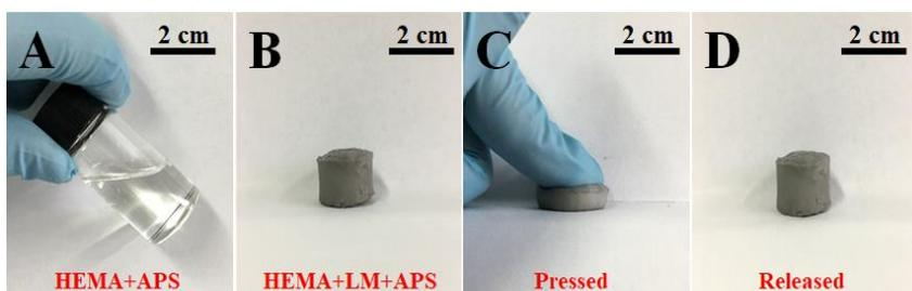
**Figure S2.** Synthesis of LM-HEMA hydrogel (A) without LM. No gelation was observed without liquid metal. B) The cylinder LM-HEMA hydrogel (10 vol%) was prepared by adding LM to initiate the gelation. Photos of C) pressed and D) released LM- HEMA gel (10 vol%).
