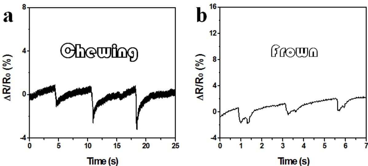
**Figure S18.** Resistive change from pristine hydrogels of (a) chewing and (b) frown. Hydrogel without liquid metals exhibited weaker signals or lost the detailed information of the motion. Experimental setup was the same as LM-hydrogel as shown in Figure S16.
