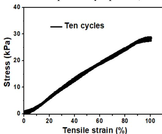
**Figure S7.** The cyclic tensile curves of LM-hydrogel (10 vol%) at strain of 100% for ten cycles.
