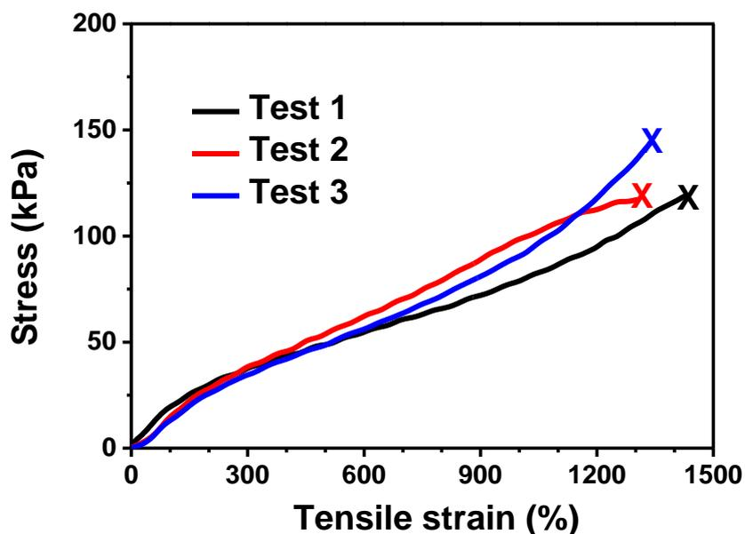
**Figure S5.** The tensile mechanical curves of LM (eutectic gallium indium, melting point: 10 °C)-hydrogel (10 vol%).
