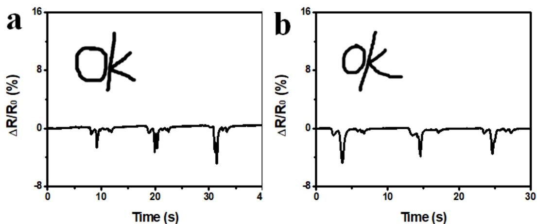
**Figure S15.** (a-b) The resistive responses of pristine hydrogels to the words "OK" written by two different researchers. Pristine gels lost the ability to discern personal writings.
