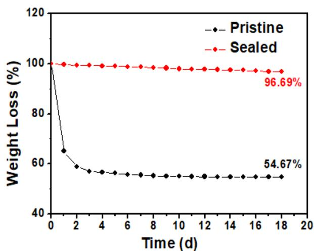
**Figure S19.** Time-dependent mass changes of LM-hydrogel (10 vol%) with (sealed) or without (pristine) PVDF sealing.
