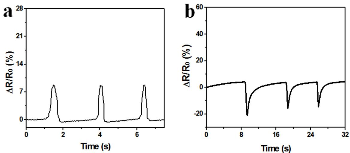
**Figure S17.** Resistive change of forefinger bending with pristine hydrogel attached outside (a) and inside (b). Pristine hydrogels showed comparable signals as LM-hydrogels under large deformation. Experimental setup was the same as LM-hydrogel as shown in Figure 6a- 6b.
