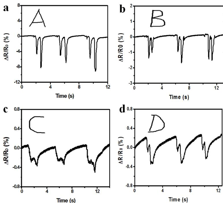
**Figure S14.** Resistive change of pristine hydrogel pad when writing A, B, C and D; each letter was written for three times to show the repeatability. Compared with LM-hydrogels, peaks from pristine hydrogels are weaker and do not show subtle changes of each letter.
