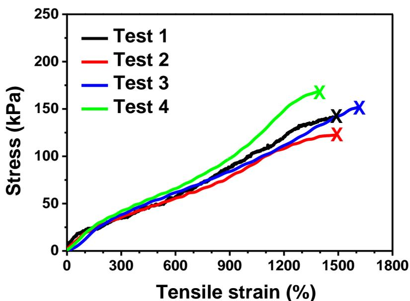
**Figure S6.** The tensile mechanical curves from three independent LM-hydrogels (10 vol%) and the curve previously reported (black curve of test 1) in **Figure 2c**.
