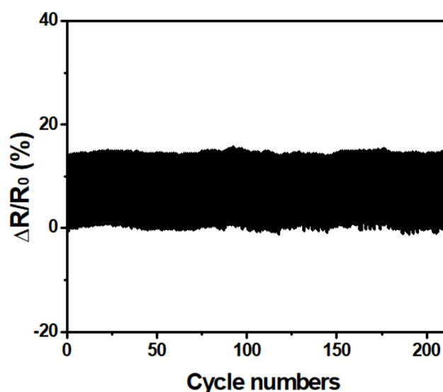
**Figure S10.** Resistance cycles sensing of 10 vol% LM-hydrogel over 200 times, each cycle applied by tensile strain to 30%. No obvious change of signals was exhibited after more than 200 cycles of tensile deformation, confirming the good electrical stability.
