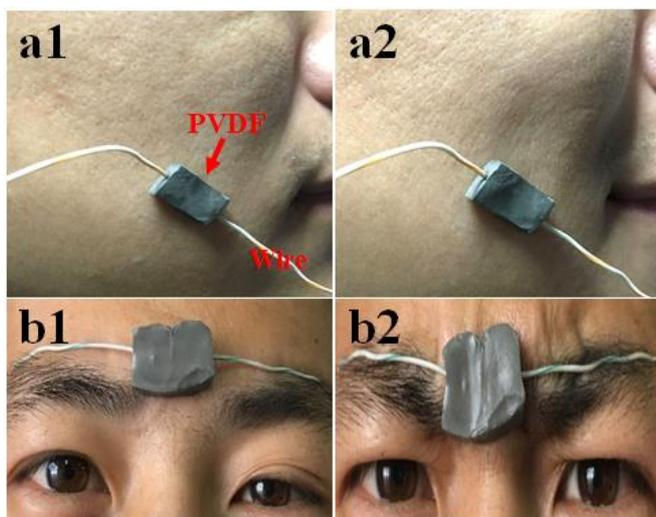
**Figure S16.** Experimental setup for hydrogels to detect bodily motion from human face (a) Chewing and (b) Frown. The electrodes were copper wires fixing by double-side tape to adhere to skin.
