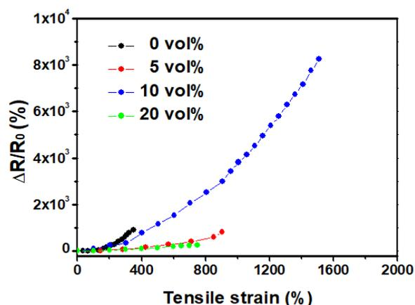
**Figure S8.** The strain-resistive change curves for tensile strain. The LM-hydrogel is conductive all the time until its breaking.
