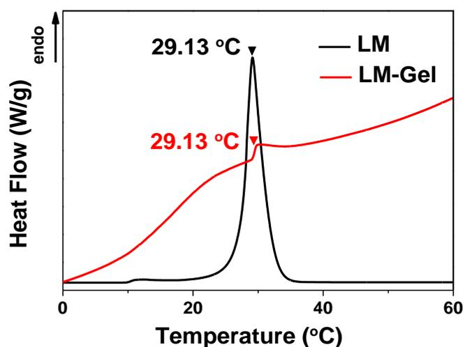
**Figure S1.** The differential scanning calorimetry (DSC) curves of liquid metal and LM-hydrogel to determine the melting points of liquid metal in LM-hydrogel (10 vol%). It indicated that the melting point of LM had no obvious shifting after gelation.
