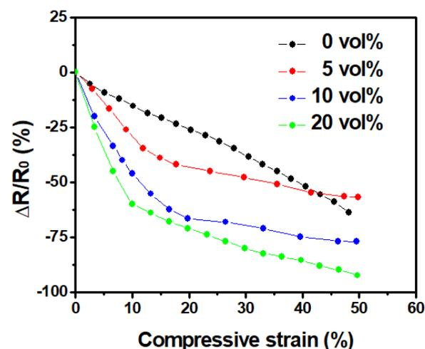
**Figure S9.** The strain-resistive change curves for compressive strain.
