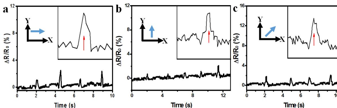
**Figure S11.** Resistive change of pristine hydrogel in response to object motion on its surface along (a) x direction, (b) y direction and (c) 45° angel along x direction; Each movement in Figure 4a – c was repeated for three times and insets are detailed response for one movement.
