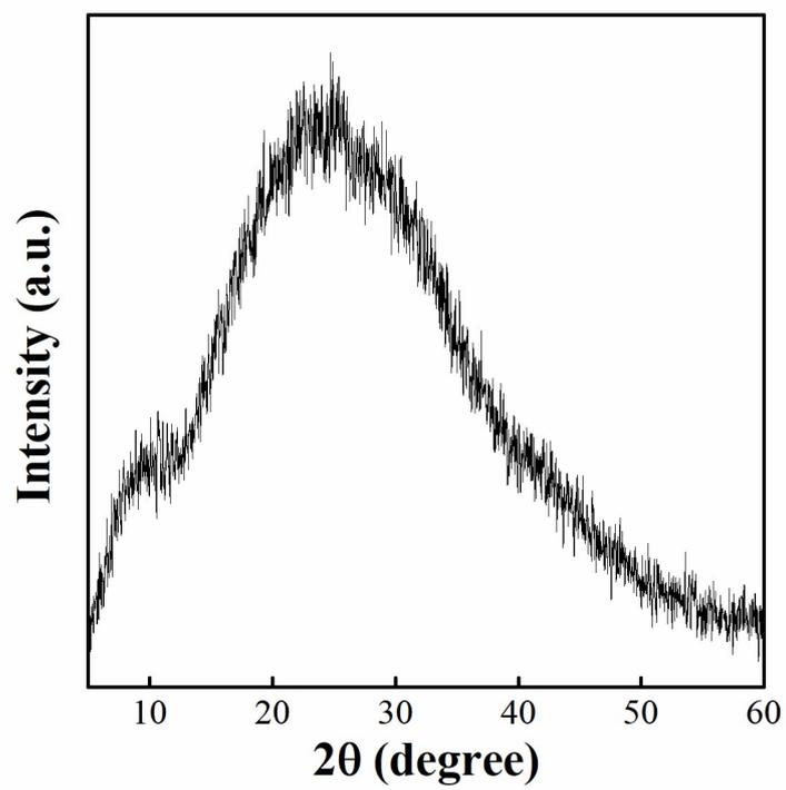
**Figure S1.** XRD pattern of the CDs
