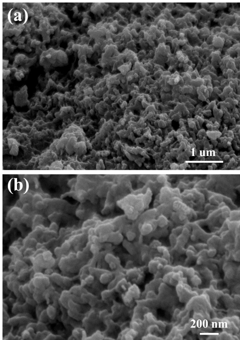
**Fig. S1** SEM images (a, b) of the bulk polyaniline particle aggregates, which were prepared by direct polymerization of aniline without any template.
