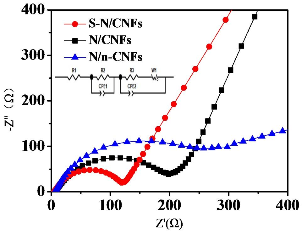
**Fig. S8** Electrochemical impedance spectra (EIS) of N/S-HCNFs, N-HCNFs and N-n-HCNFs
