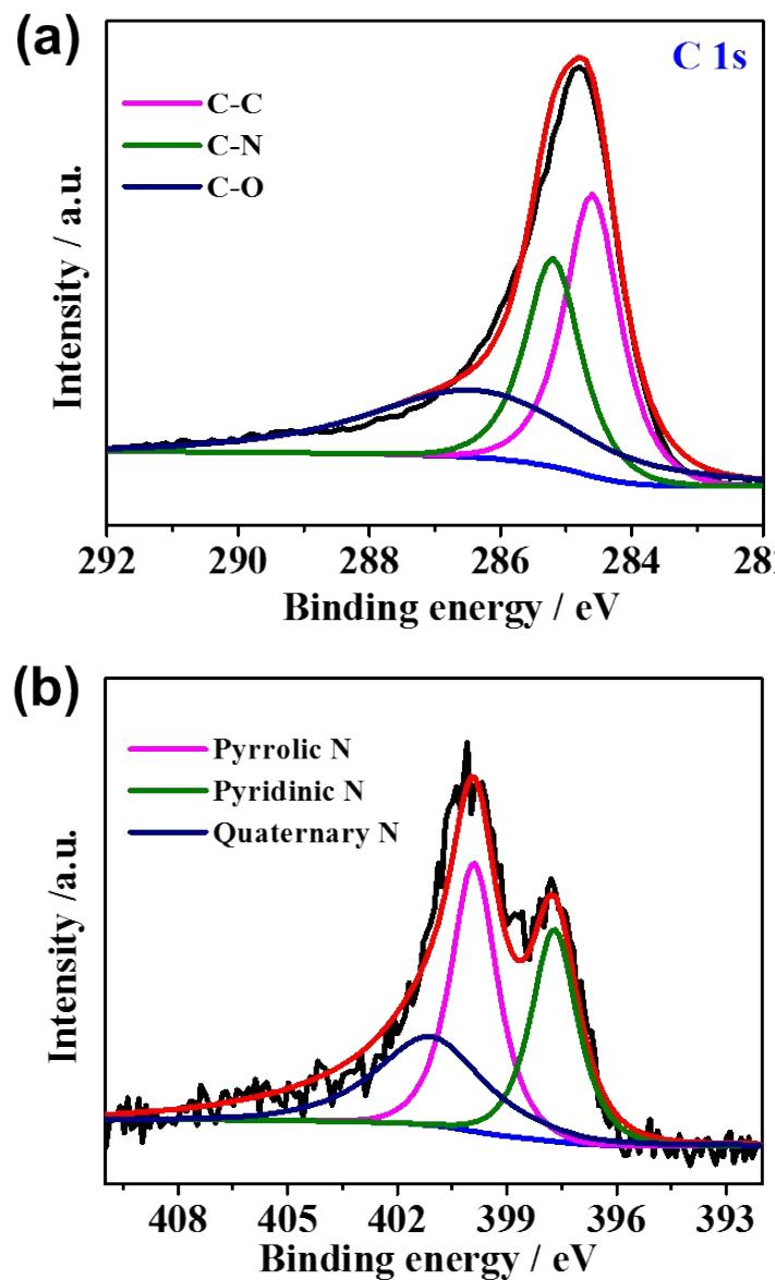
**Fig. S4** High-resolution XPS spectra of C1s (a) and N1s (b) in N-HCNFs.
