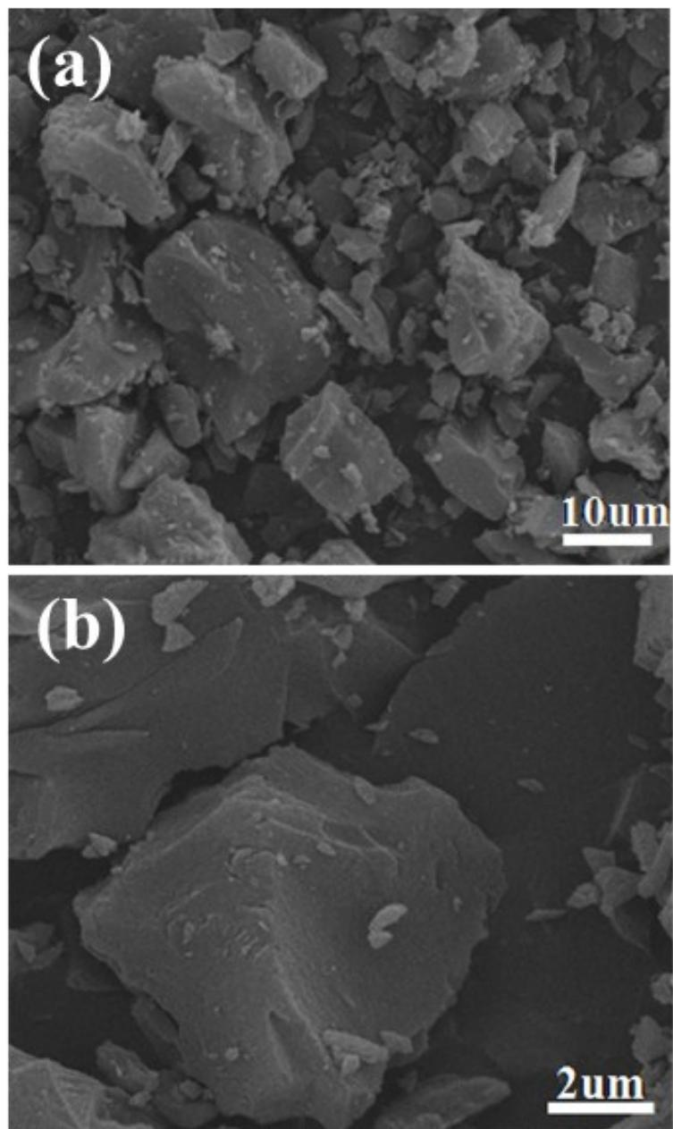
**Fig. S3** SEM images (a, b) of the AC cathode.
