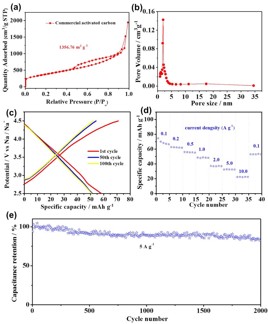
**Fig. S9** Nitrogen adsorption-desorption isotherms (a) and pore size distribution (b) of commercial AC. Electrochemical properties of the AC electrode in a Na half-cell between 2.5 and 4.5 V vs.  $\text{Na}/\text{Na}^+$ . (c) Charging/discharging curves of the AC electrode at 1st, 50th and 100th at  $0.1 \text{ A g}^{-1}$ . (d) Specific capacities at different current densities. (e) Cycling performance at  $5 \text{ A g}^{-1}$ .
