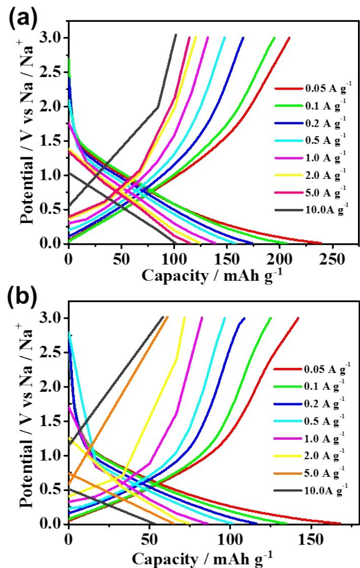
**Fig. S5** Charge and discharge curves of as-synthesized N-HCNFs (a) and N-n-HCNFs (b) at different current densities.
