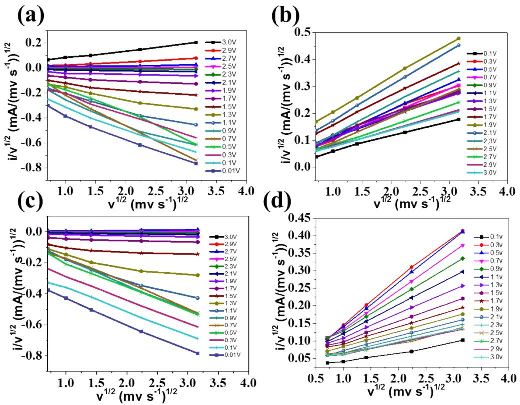
**Fig. S7** The plots of  $i/v^{1/2}$  vs  $v^{1/2}$  used for calculating constants  $a_1$  and  $a_2$  for the cathodic process. of N/S-HCNFs (a) and N-HCNFs (c). The plots of  $i/v^{1/2}$  vs  $v^{1/2}$  used for calculating constants  $a_1$  and  $a_2$  for the anodic process of N/S-HCNFs (b) and N-HCNFS (d).
