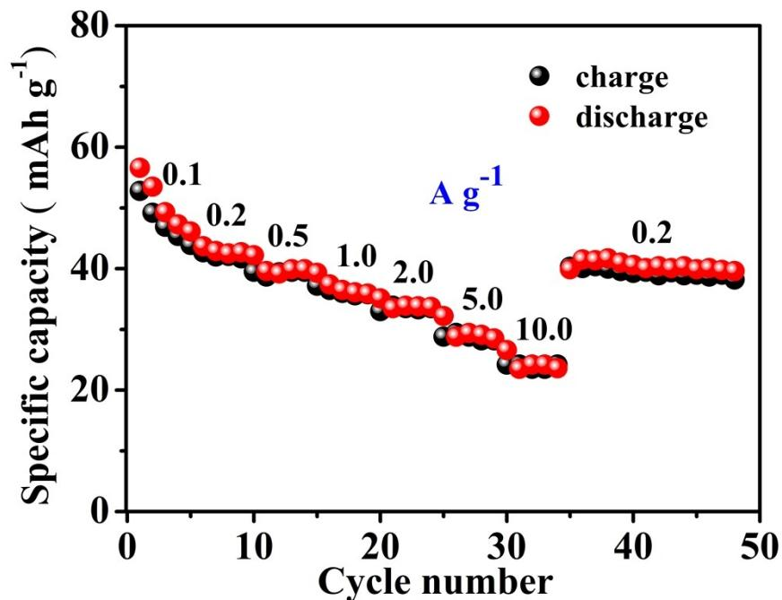
**Fig. S10** Rate performance of the as-assembled NIC at different current densities based on the total mass of S-N/CNTs and AC.
