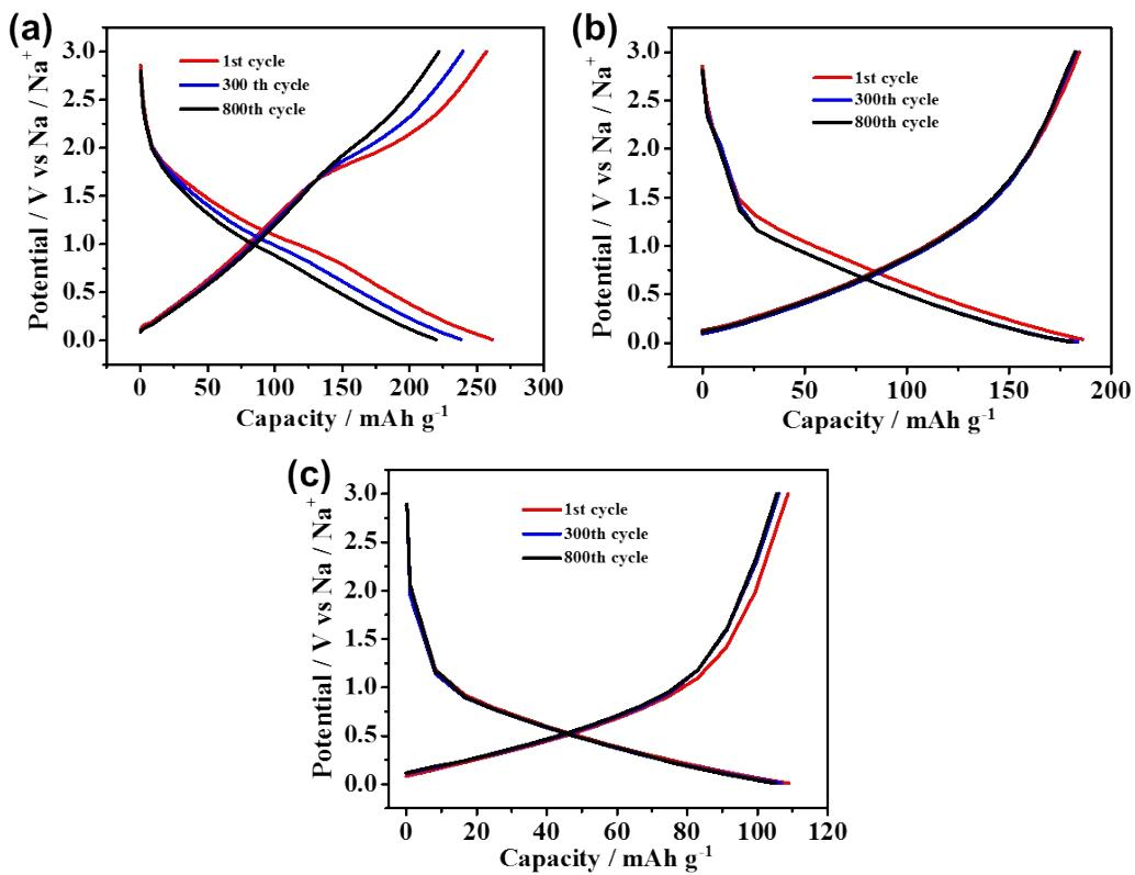
**Fig. S6** Charge and discharge curves of as-synthesized N/S-HCNFs (a), N-HCNFs (b) and N-n-HCNFs (c) at 1st, 300th and 800th at  $0.5 \text{ A g}^{-1}$ .
