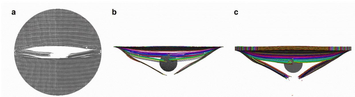
**Figure S6:** Splitting failure for Bouligand film with  $\gamma=0^\circ$ : (a) top view and (b) side view of the first layer, and (c) side view of the entire structure splitting. Different colors represent individual CNC fibers and the grey spheres are the projectiles.
