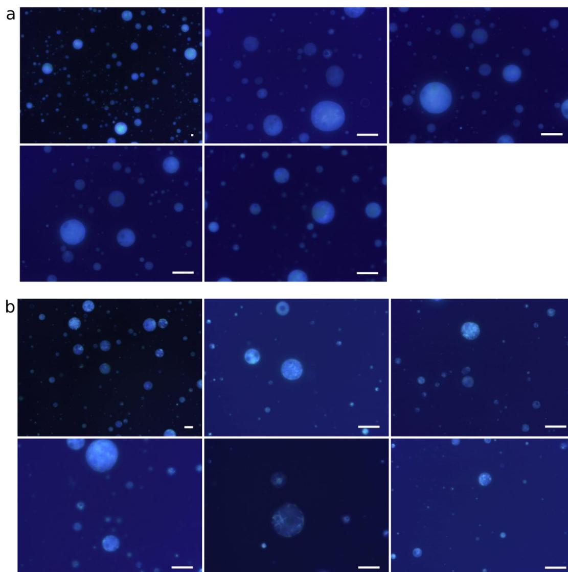
**Figure S10:** Formation of fibers in water-in-oil emulsions of **CP1** (2% w/w); a) dissolved in water and b) diluted in HEPES (30 mM) at pH 8. Scale bar is 10 μm.
