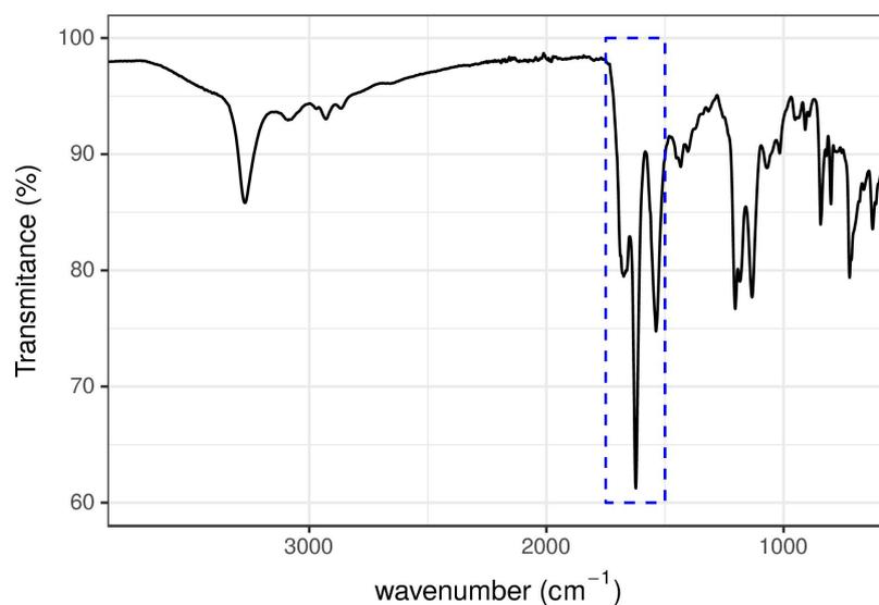
**Figure S2:** IR-ATR of a freeze-dried sample of **CP1** (2 % w/w) after alkalization with NaOH (0.1 M). Base was added until a gel was obtained. The dashed blue box indicates the presence of intense peaks of the amides I and II at  $1623$  and  $1538 \text{ cm}^{-1}$  respectively.
