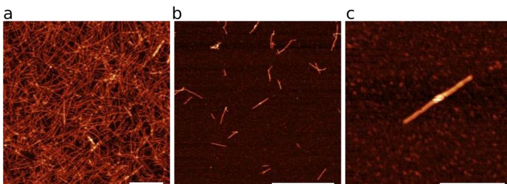
**Figure S7:** AFM images of CP1 (0.2 % w/w) at pH *ca* 8 obtained by dilution of the gel: a) High density of nanotubes; b) low density; c) single nanotube. Persistence length was estimated from the later. Scale bars are 1  $\mu\text{m}$  (a), 500 nm (b and c)
