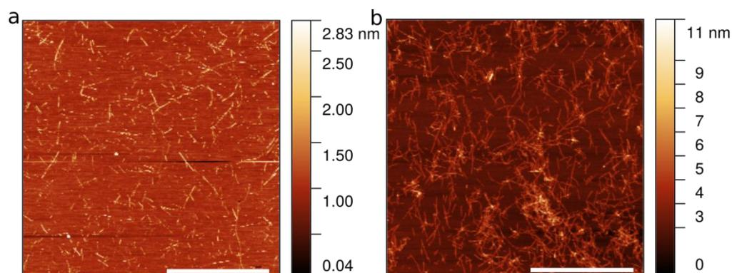
**Figure S6:** AFM images of **CP1** (0.2 % w/w) solutions at different pH deposited on mica surface: a) after dissolving in water (pH ~ 4) b) upon alkalinization (pH ~ 8). Scale bar is 4 μm.
