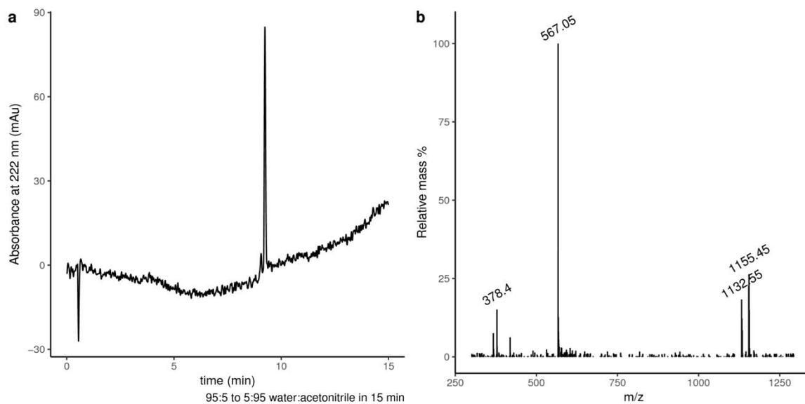
**Figure S13:** a) Chromatogram of CP1 after purification; b) MS spectra from the main peak.
