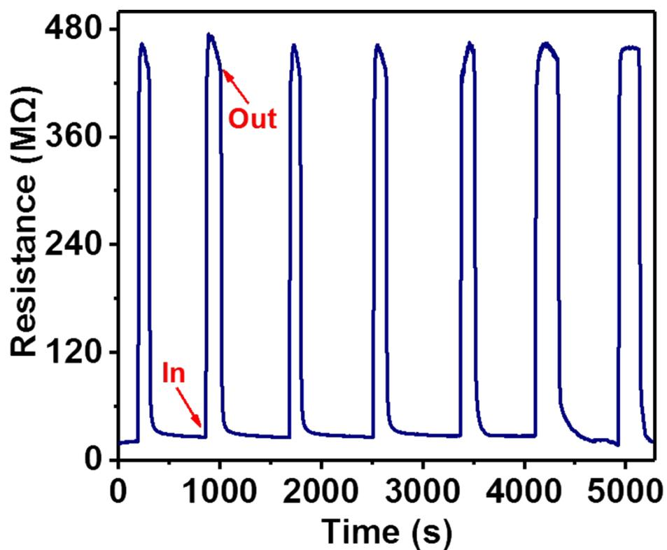
**Fig. S5** The reproducibility of the ZnO-BP sensor upon seven cycles to 100 ppb  $\text{NO}_2$  at 160 °C.
