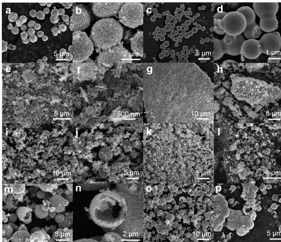
**Fig. S7** SEM images of (a) and (b) ZnO hollow spheres; (c) and (d) ZnO-1; (e) and (f) ZnO-2; (g) and (h) ZnO-3; (i) and (j) ZnO-4; (k) and (l) ZnO-5; (m) and (n) ZnO-6; (o) and (p) ZnO-7.
