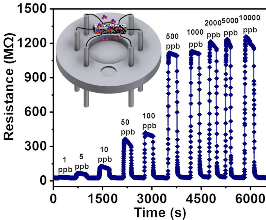
Fig. S3 Dynamic response-recovery curves of ZnO-BP sensor to different NO<sub>2</sub> concentrations at 160 °C.
