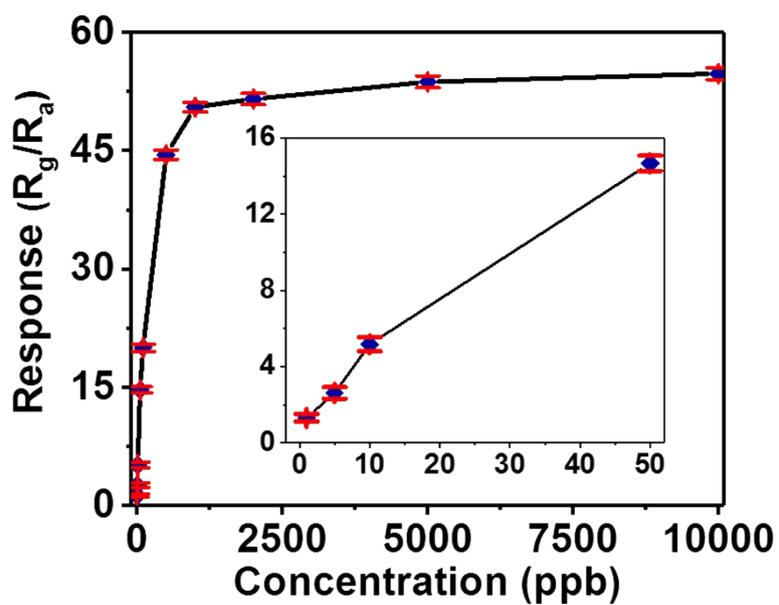
**Fig. S4** Response of ZnO-BP sensor as a function of  $\text{NO}_2$  concentrations (1-10000 ppb) at 160 °C, the inset shows the response at low  $\text{NO}_2$  concentrations (1-50 ppb).
