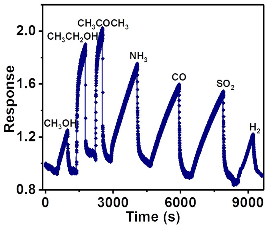
**Fig. S6** Dynamic response curves of the sensor based on ZnO-BP to 1 ppm various gases (CH<sub>3</sub>OH, CH<sub>3</sub>CH<sub>2</sub>OH, CH<sub>3</sub>COCH<sub>3</sub>, NH<sub>3</sub>, CO, SO<sub>2</sub>, and H<sub>2</sub>) at 160 °C.
