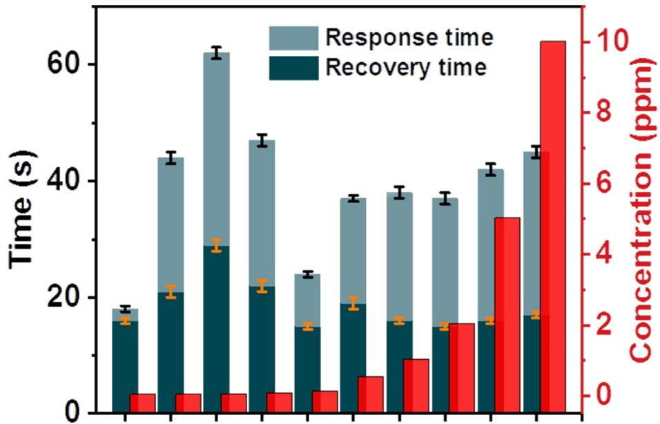
Fig. S2 Response and recovery time of the ZnO-BP gas sensor to different concentrations NO<sub>2</sub> at 160 °C.
