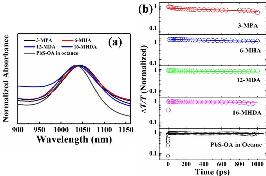
**Fig. S4** (a) Absorption spectra of PbS QD films capped by different MAA ligands and PbS QDs capped by OA in Octane. (b) TA time decay curves of PbS QD films capped by different MAA ligands and PbS QDs capped by OA in Octane solutions. TA signal intensities were normalized at 5 ps. The solid lines are the fitting results.
