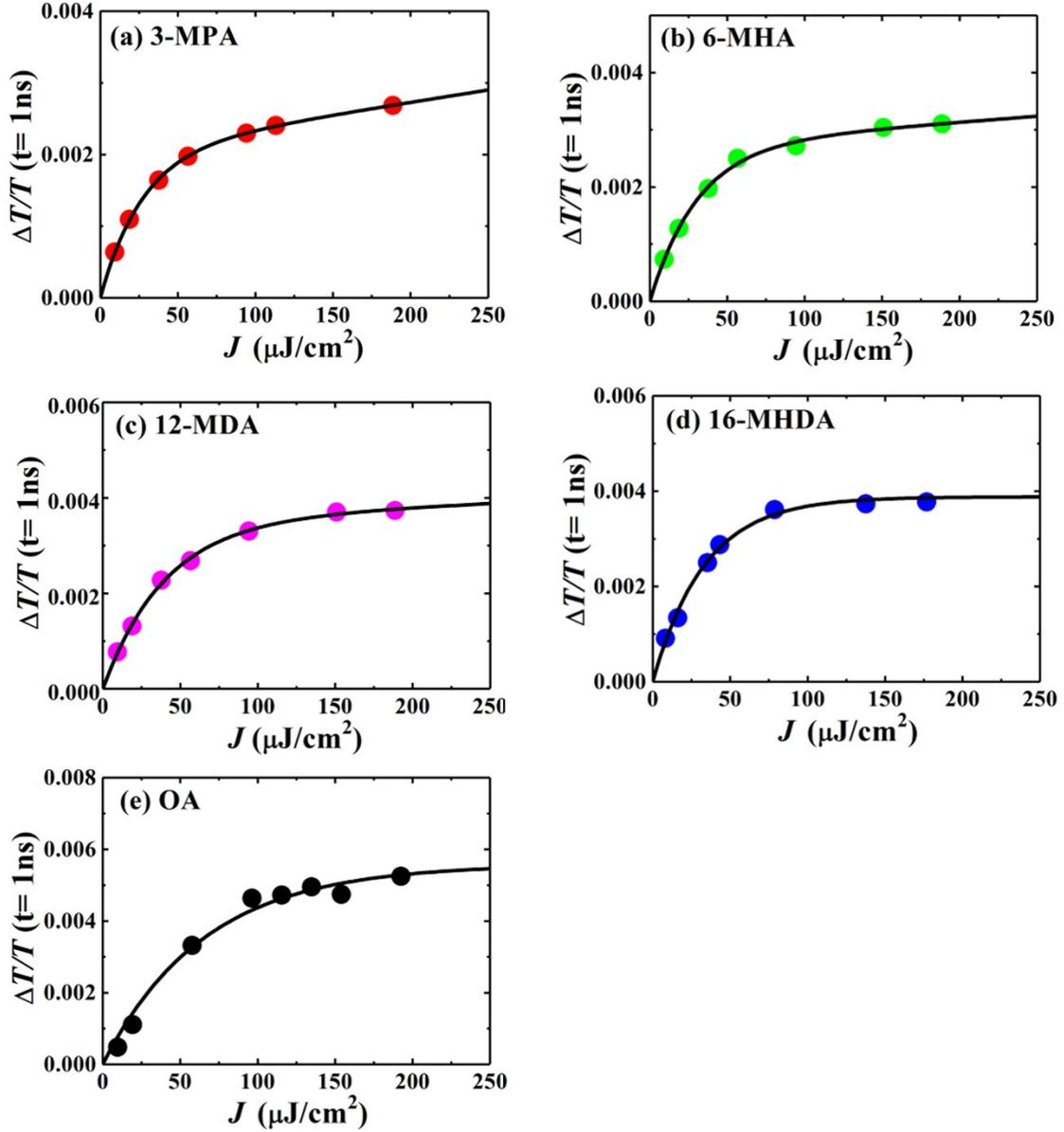
**Fig. S6** TA signals of (a) 3-MPA, (b) 6-MHA, (c) 12-MDA and (d) 16-MHDA treated films and (e) OA-capped-PbS QDs in octane (isolated QDs) vs the excitation fluence ( $J$ ) at delay time of 1 ns. The solid curves are the fitting results.
