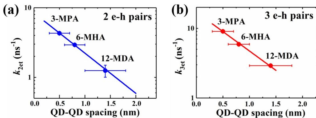
**Fig. S8** Correlation between QD-QD spacing and charge transfer rate constants  $k_{2et}$  and  $k_{3et}$  of 2 *e-h* pairs (a) and 3 *e-h* pairs (b) for MAA ligands treated films. A single exponential decay fitting (dotted line) indicates that the carrier transfer occurs via tunneling of charge through a potential barrier.
