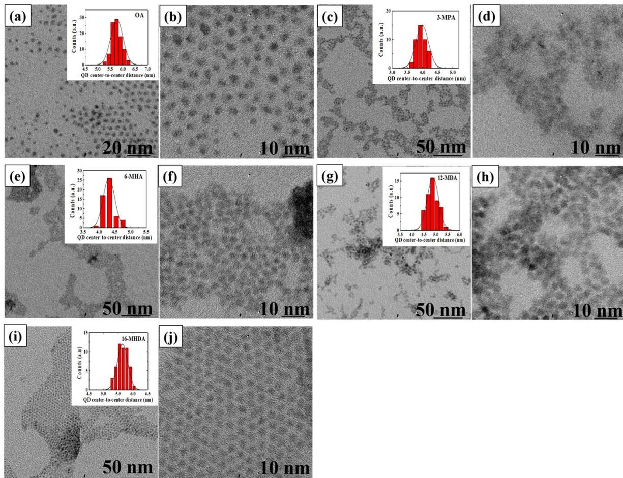
**Fig. S2** TEM images of chemically treated PbS QD films with different ligands: (a, b) OA; (c, d) 3-MPA; (e, f) 6-MHA; (g, h) 12-MDA and (i, j) 16-MHDA. The inset Figures are the histograms of the QD center-to-center distances.
