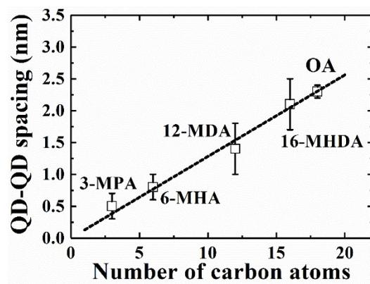
**Fig. S3** The linear relationship between the QD-QD interparticle spacing and the number of carbon atoms of capping ligands.
