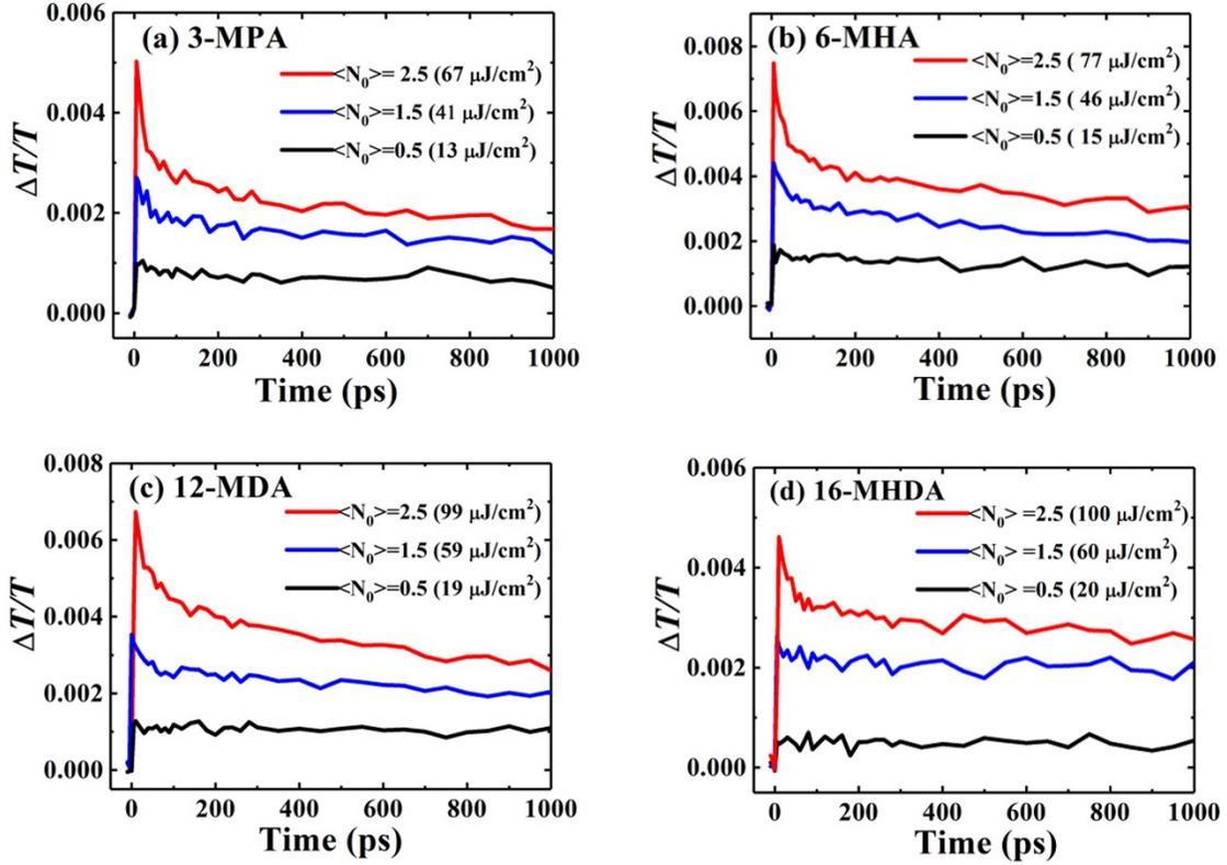
**Fig. S7** Excitation-fluences dependent of TA curves of (a) 3-MPA, (b) 6-MHA, 12-MDA and 16-MHDA treated films. Average number of  $e-h$  pair per QD:  $\langle N_0 \rangle = J_p \sigma$ , <sup>5, 6</sup> where  $J_p$  and  $\sigma$  is photon fluence and absorption cross section, respectively.
