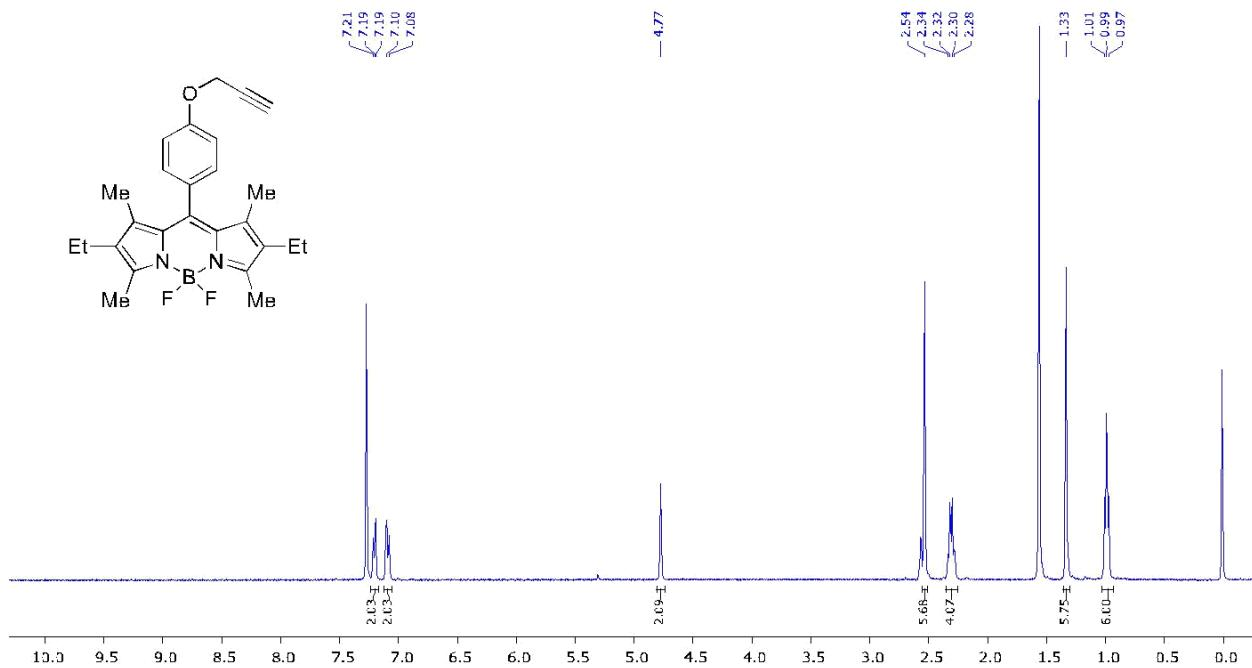
**Figure 1:**  $^1\text{H}$  NMR of BODIPY **1** in  $\text{CDCl}_3$  (400 MHz)
