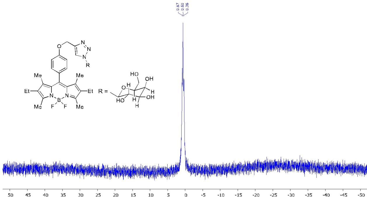
**Figure 25:**  $^{11}\text{B}$  NMR of BODIPY **4c** in  $\text{CDCl}_3$  (128 MHz)
