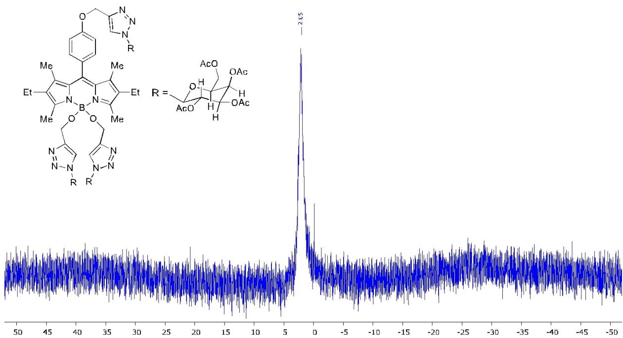
**Figure 22:**  $^{11}\text{B}$  NMR of BODIPY **3b** in  $\text{CDCl}_3$  (128 MHz)
