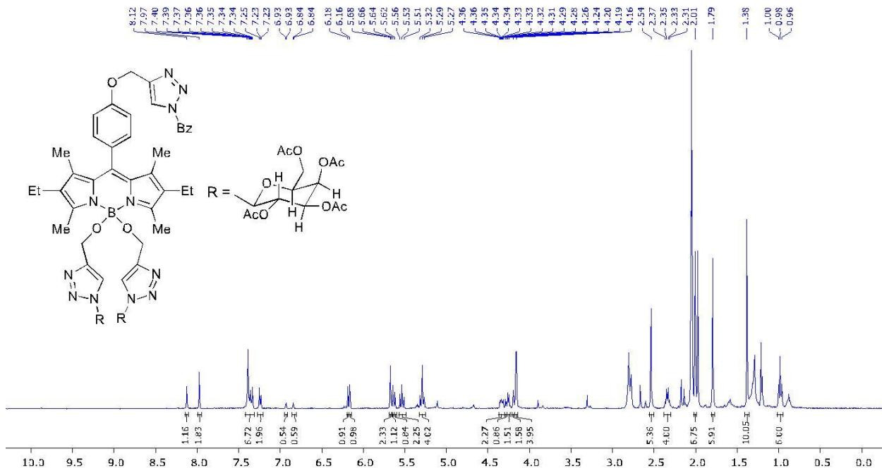
**Figure 17:**  $^1\text{H}$  NMR of BODIPY **6a** in acetone (400 MHz)
