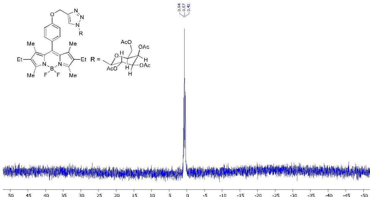
**Figure 24:**  $^{11}\text{B}$  NMR of BODIPY **4b** in  $\text{CDCl}_3$  (128 MHz)
