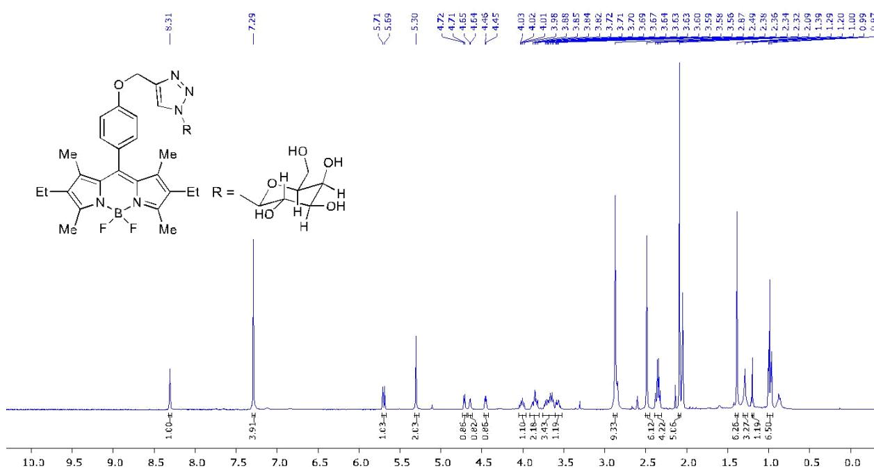
**Figure 13:**  $^1\text{H}$  NMR of BODIPY **4c** in acetone (400 MHz)
