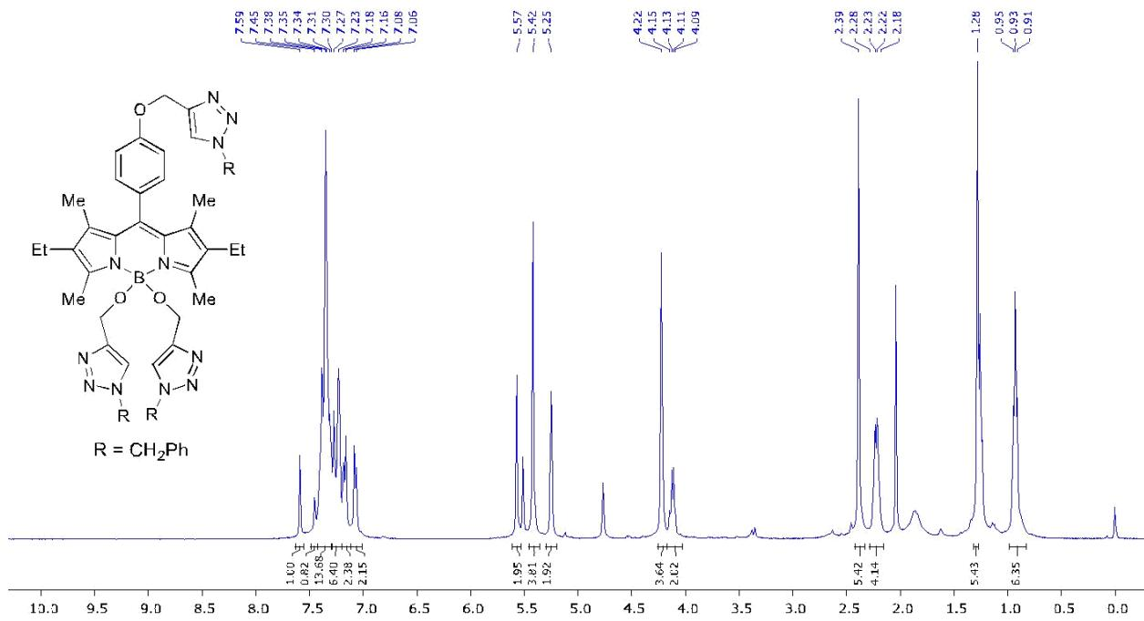
**Figure 5:**  $^1\text{H}$  NMR of BODIPY **3a** in  $\text{CDCl}_3$  (400 MHz)
