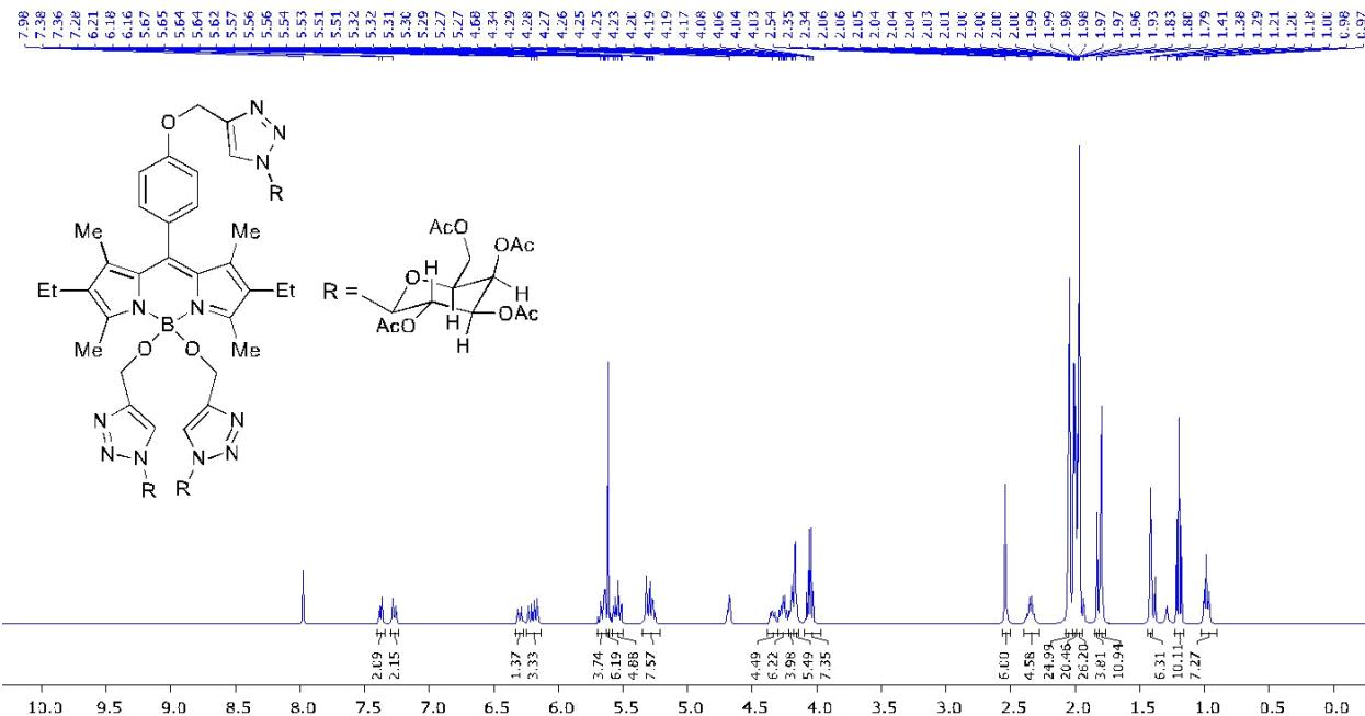
Figure 7:  $^1\text{H}$  NMR of BODIPY 3b in acetone (400 MHz)
