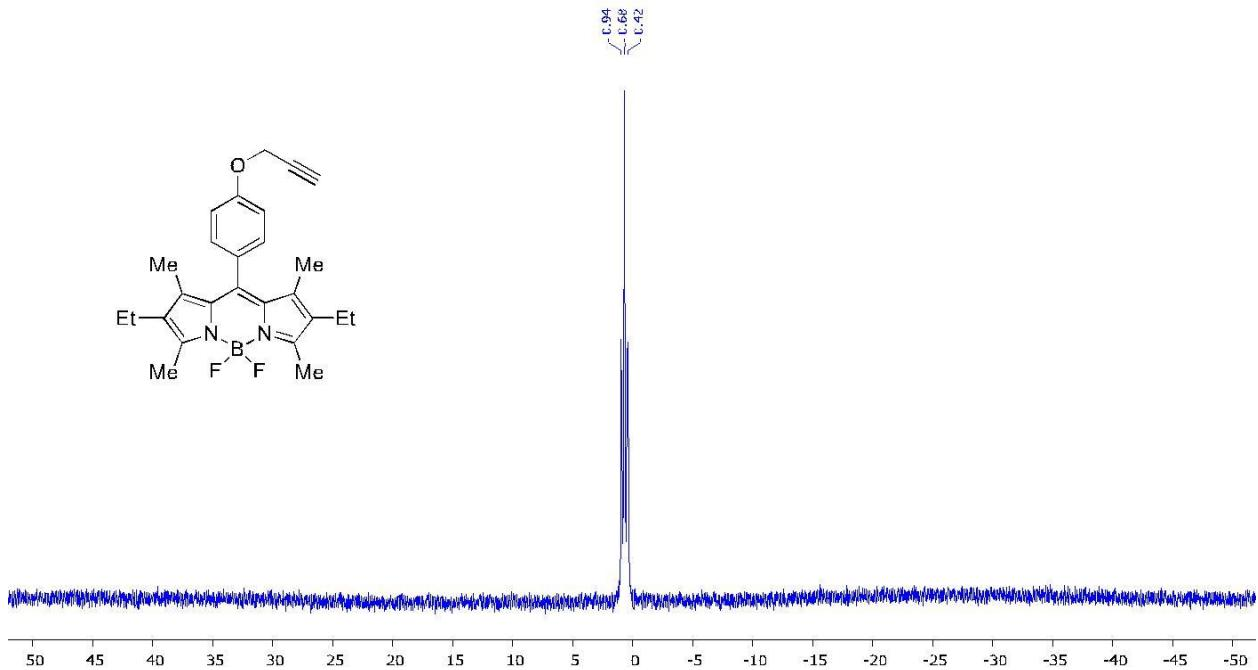
**Figure 19:**  $^{11}\text{B}$  NMR of BODIPY **1** in  $\text{CDCl}_3$  (128 MHz)
