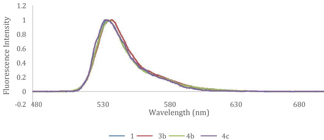
**Figure 29:** Normalized fluorescence emission spectra of selected BODIPYs **1**, **3b**, **4b** and **4c** in DMSO at room temperature.
