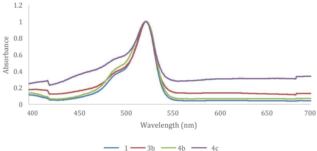
**Figure 28:** Normalized UV-Vis spectra of selected BODIPYs **1**, **3b**, **4b** and **4c** in DMSO at room temperature.
