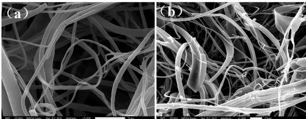
Figure S6 (a) SEM image of PGMA-*b*-PS (BCP-3) fibers, and the solution concentration and rotation speed were 0.3 g/ml and 2000 r/min, respectively; (b) SEM image of PGMA-*b*-PS (BCP-3) fibers, and the solution concentration and rotation speed were 0.4 g/ml and 2000 r/min, respectively.
