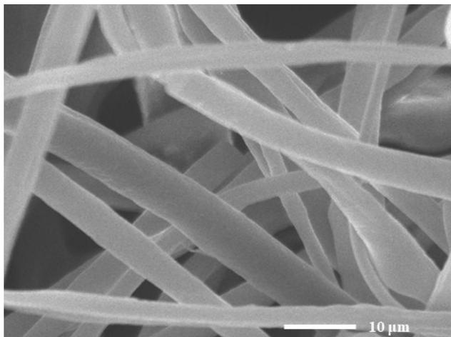
Figure S8 SEM image of PGMA-*b*-PS fibers formed by BCP-6, and the solution concentration and rotation speed were 0.3 g/ml and 1500 r/min, respectively. The contents of glycerin and methanol were 40 ml and 410 ml, respectively.
