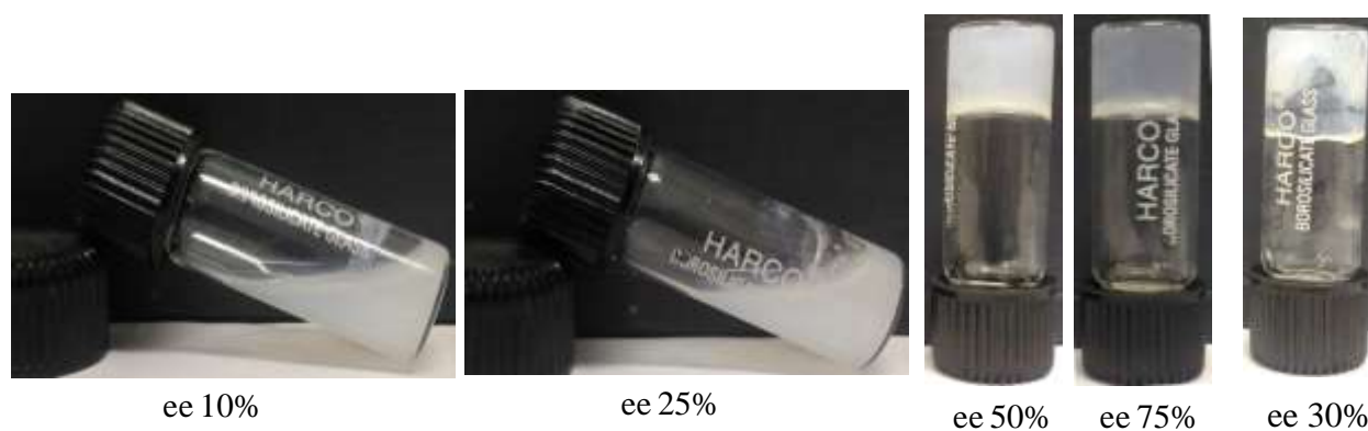
Figure S7. Digital images of the precipitates and hydrogels formed by histidine and Zn^{2+} ions with varying ee % of D -histidine. Partial gel formed upon addition of Zn^{2+} ions to a 30% ee solution of D -histidine.
