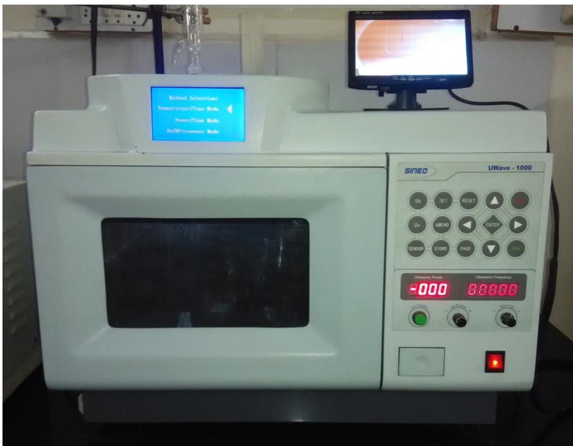
Figure S1. Digital photograph of SINEO UWave-1000 microwave synthesizer used in the study.
