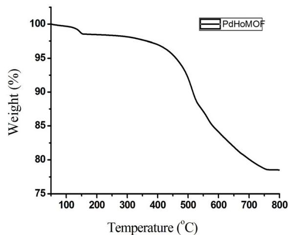
**Fig. S4** The TG curve of **PdHoMOF**.
