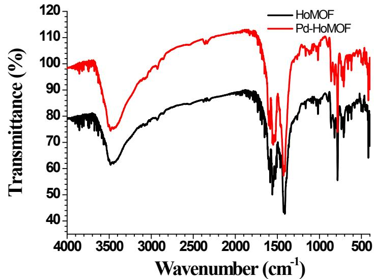
**Fig. S1** The IR spectra of **HoMOF** and **Pd-HoMOF**.
