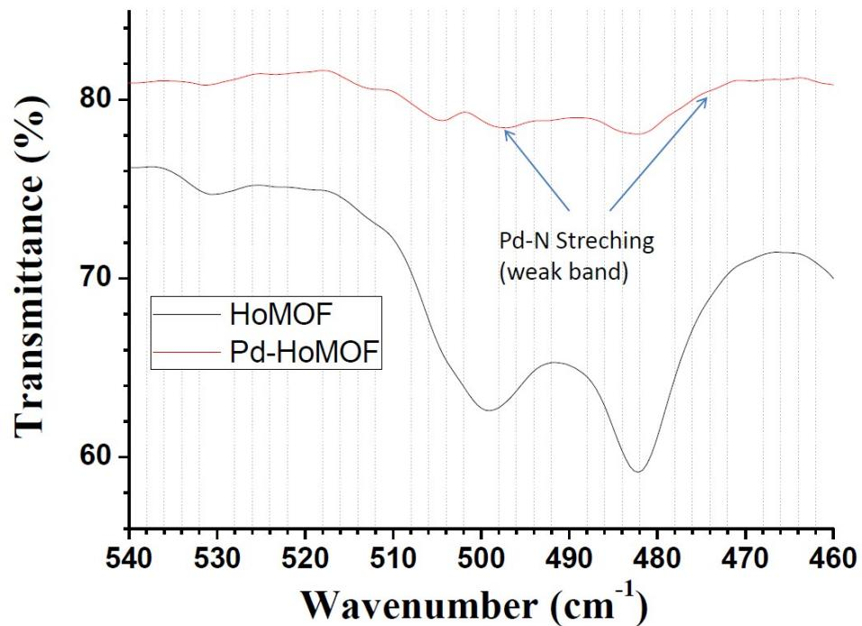
Fig. S2 IR spectra of **HoMOF** (black) and **Pd-HoMOF** (red) demonstrating the two weak Pd–N stretching observed for **Pd-HoMOF**.
