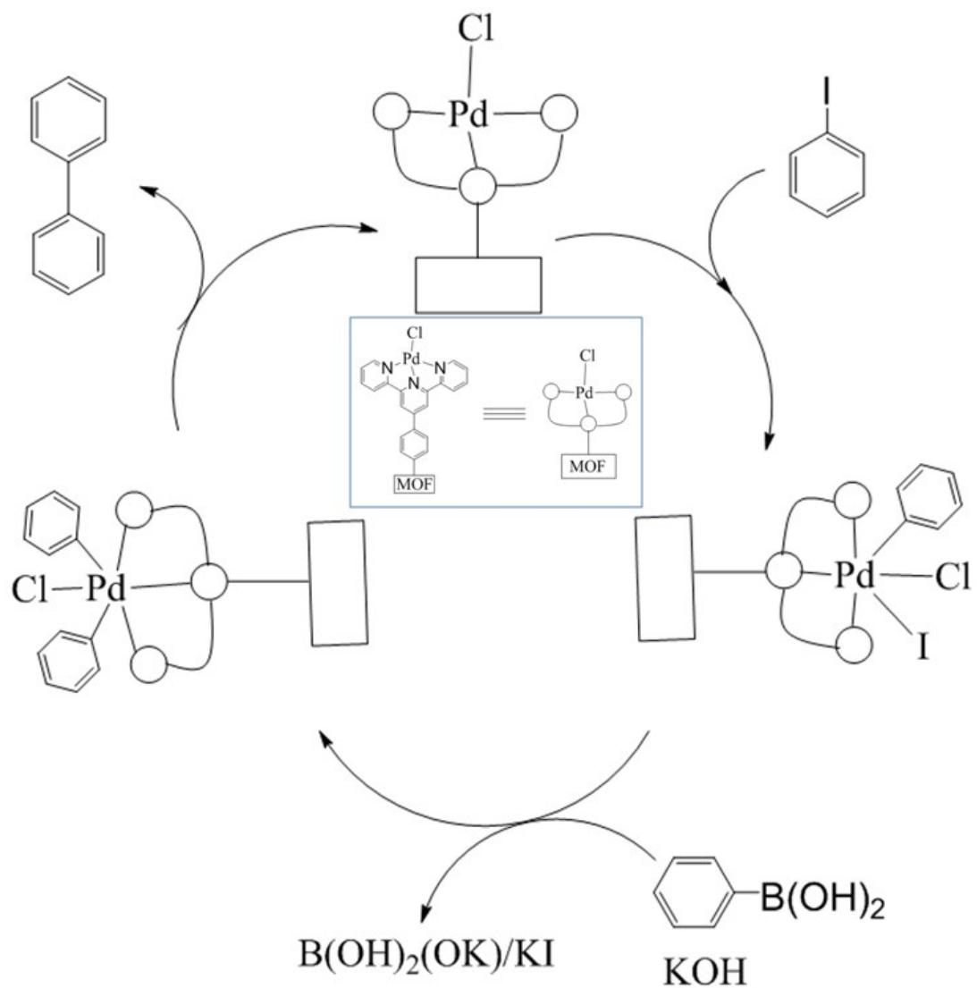
Scheme S1 An illustrative sketch of proposed mechanism of the Suzuki–Miyaura reaction of iodobenzene in the presence of Pd-HoMOF catalyst.
