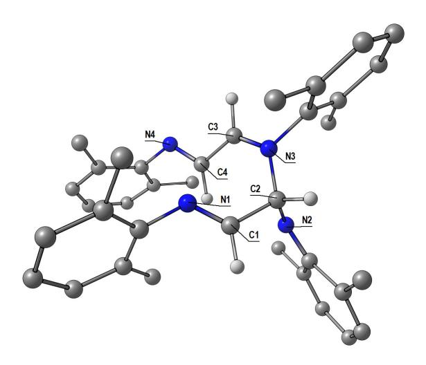
**Figure SI-4**. DFT-optimized geometry of [WCl<sub>5</sub>{N(Ar)C(CHNXyl)NXylCHCHNXyl}] $^+$  (C-PCM/ $_{\odot}$ B97X calculations) and spin density surface (isovalue = 0.01 a.u.). Hydrogen atoms on the Xyl moieties are omitted for clarity. Colour map: W, orange; Cl, green; N, blue; C, grey; H, white; spin density surface: yellow tones. Selected computed lengths (Å): C1-N1 1.265, C2-N2 1.256, C2-N3 1.464, C3-N3 1.291, C4-N4 1.271, C1-C2 1.491, C3-C4 1.471, W-Cl (average) 2.294, W---N2 4.307.
