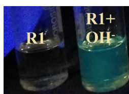
Fig. S7 Fluorometric response of R1 with the addition of 2 equiv. of TBAOH
