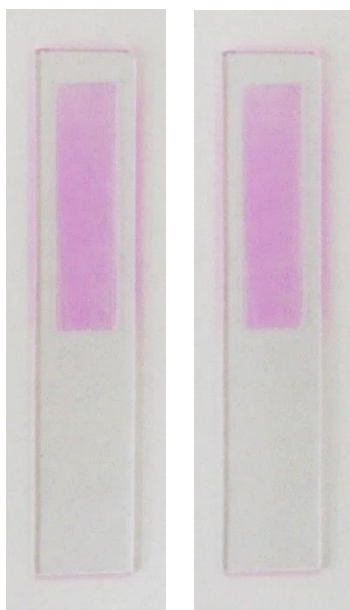
Fig. S17 Photographs of the 1a/PVA film on the glass slide (a) before and (b) after washing with methanol.
