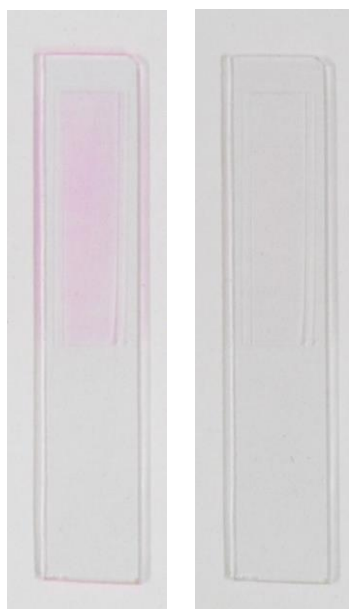
Fig. S19 Photographs of the 1b/PVA film on a glass slide (a) before and (b) after washing with methanol.
