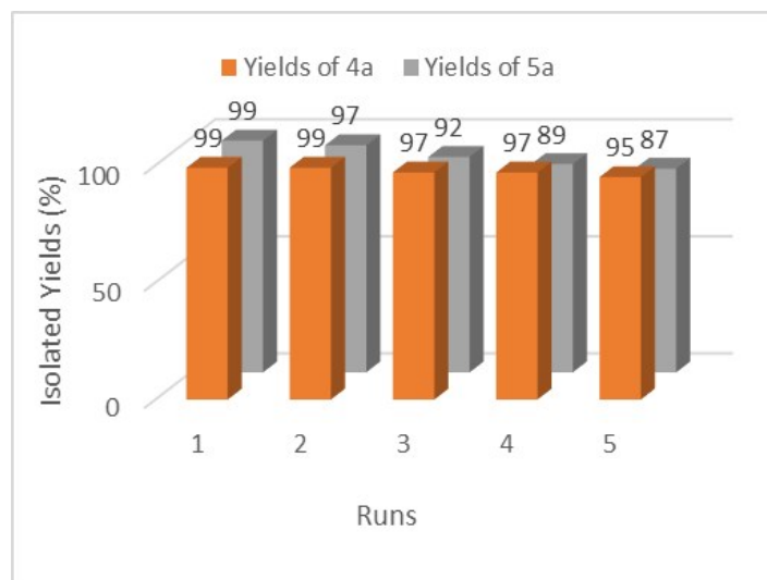
Fig. 6 Reusability of the GO/ZnO nanocomposite ( 1 ) for the synthesis of 4a and 5a .
