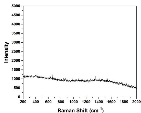
Fig. S7 Raman spectrum of the pPLLA electrospun nanofiber membrane after dipping into 1 mM AgNO<sub>3</sub> solution for 24 h. 0.1 mM 4-ATP solution was dropped on the sample and left to dry.
