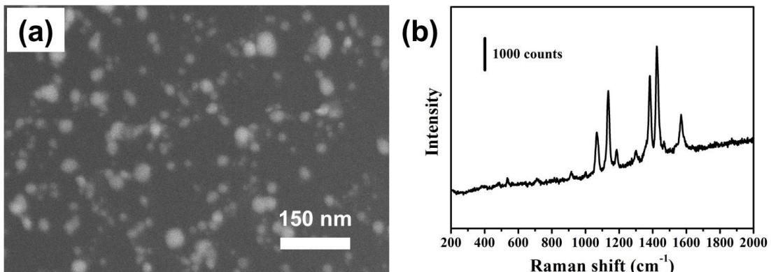
Fig. S4 (a) SEM image of Ag NPs assembled on plasma treated PLLA 2D thin film; (b) SERS spectrum of 0.1 mM 4-ATP molecules collected on the corresponding Ag NPs decorated thin film. The 2D thin film was spin-coated from PLLA solution. The plasma treatment and the assembly procedure are the same as the ones of pPLLA-Ag NPs nanofiber membrane.
