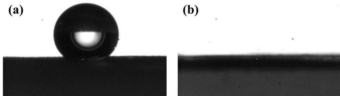
Fig. S2 The wetting behavior of the PLLA electrospun membrane before (a) and after (b) the plasma treatment.
