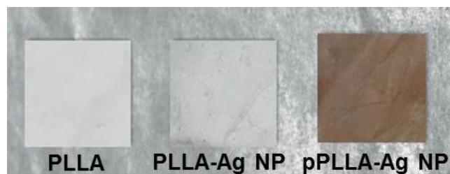
Fig. S3 Photographs of the pristine PLLA electrospun membrane (left), the pristine PLLA electrospun membrane after immersion in Ag NP solution (center) and the pPLLA electrospun membrane after immersion in Ag NP solution (right).
