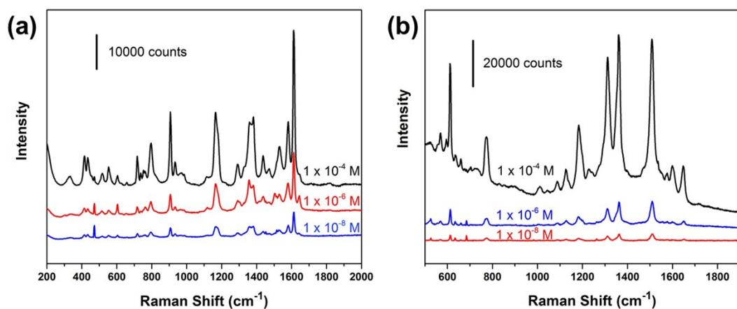
Fig. S5 SERS spectra of different concentrations of crystal violet (a) and rhodamine 6G (b) on the pPLLA-Ag NPs nanofibers.
