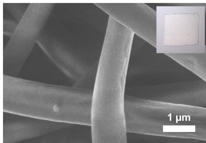
Fig. S6 SEM image and photograph (inset) of the pPLLA electrospun nanofiber membrane after immersion in negative-charged citrate-protected Ag NPs solution.
