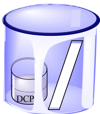
Fig. S21 Setup for the vapour phase recognition of DCP via 2@\text{SiO}_2@\text{Al} strips.
