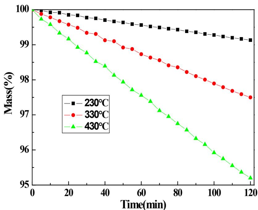
Fig. S1 Isothermal gravimetric analyses of 1-ethoxycarbonylmethyl-3-methylimidazolium tetrafluoroborate at various temperatures, N<sub>2</sub>-atmosphere.
