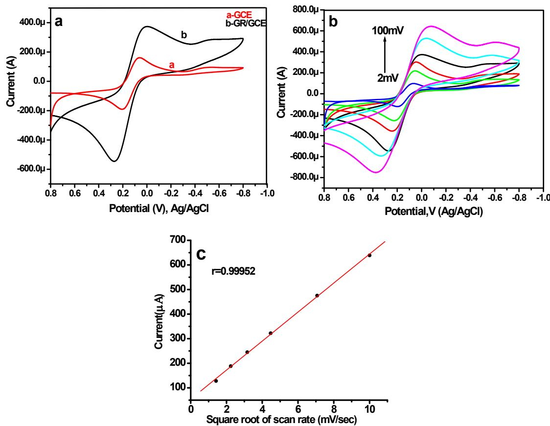
**Figure S3:** a) CV curves of GCE and GR/GCE in 0.1M KCl containing 5mM  $[\text{Fe}(\text{CN})_6]^{4-/\text{3}-}$  at 50 m  $\text{Vs}^{-1}$
