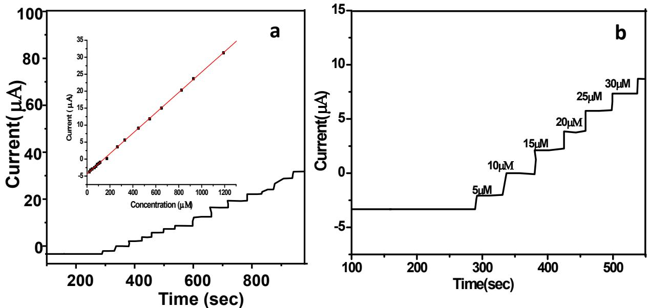
**Figure S4:** a) Amperometric responses of GR/GCE to successive addition of AA into PBS buffer. (Inset: linear curves of oxidation current versus concentration ) b) magnified portion of the amperometric response curve.
