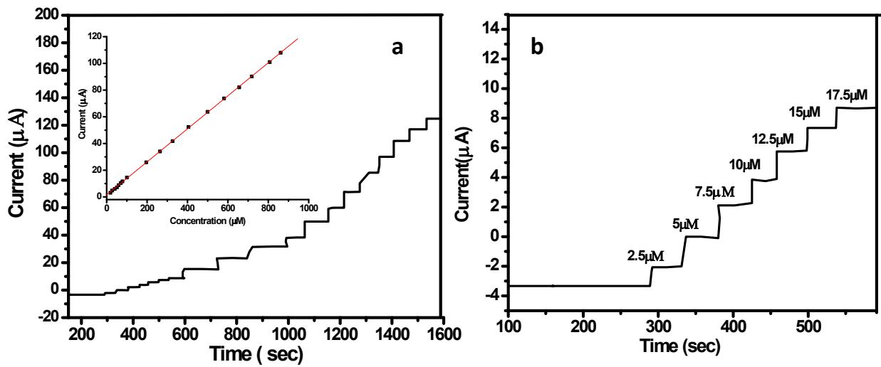
**Figure S5:** a) Amperometric responses of GR/GCE to successive addition of DA into PBS buffer (inset: linear curves of oxidation current versus concentration) b) magnified portion of the amperometric response curve.
