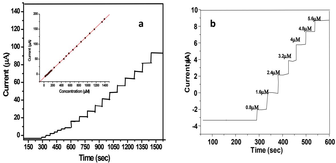
**Figure S6:** a) Amperometric responses of GR/GCE to successive addition of UA into PBS buffer (inset: linear curves of oxidation current versus concentration) b) magnified portion of the amperometric response curve.
