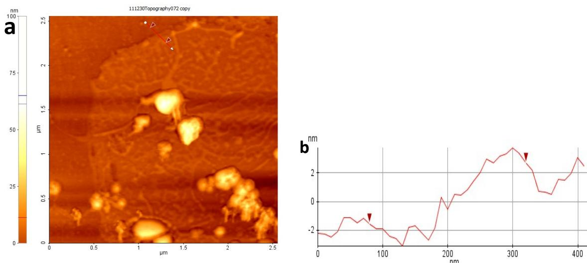
**Figure S1.** a) AFM image of GR. b) Thickness profile of the GR sheet (red scanning line)
