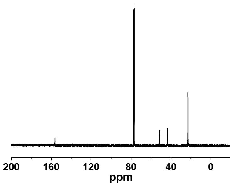
**Fig. S22** <sup>13</sup>C NMR spectra of methyl isopropyl carbamate.
