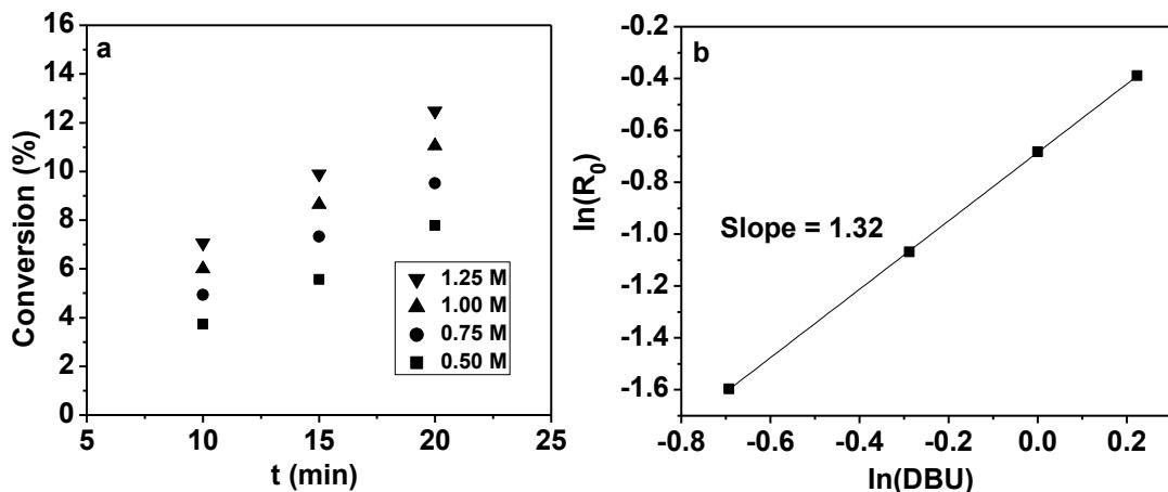
**Fig. S6** The relationship between the initial reaction rate ( $R_0$ ) and the initial concentrations of DBU. Reaction conditions: DBU (0.50-1.25 M), DMC (3.0 M), ethanol (1.0 M), CO<sub>2</sub> pressure (1.0 MPa), 100 °C.
