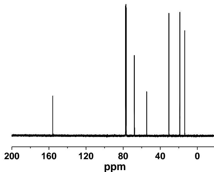
**Fig. S10** <sup>13</sup>C NMR spectra of butyl methyl carbonate.
