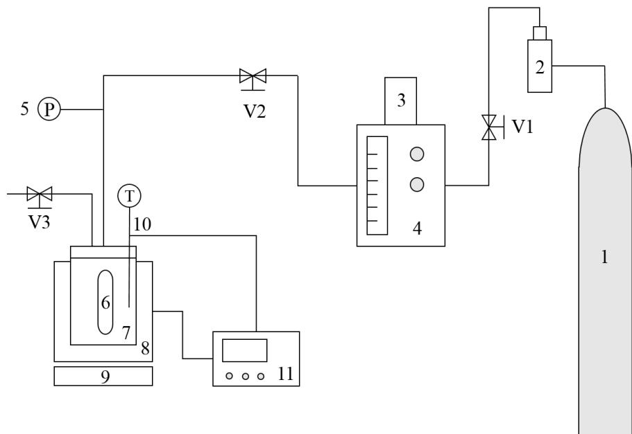
**Fig. S1** Apparatus for phase behavior. 1. CO<sub>2</sub> gas cylinder, 2. Drying tower, 3. Cold trap, 4. High-pressure metering pump, 5. Pressure sensor, 6. View window, 7. Reacting vessel, 8. Heating jacket, 9. Magnetic stirrer, 10. Thermocouple, 11. Temperature sensor. V1, V2 and V3: valve.
