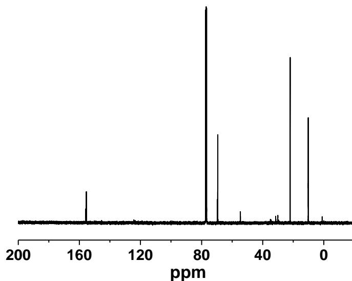
**Fig. S8** <sup>13</sup>C NMR spectra of propyl methyl carbonate.
