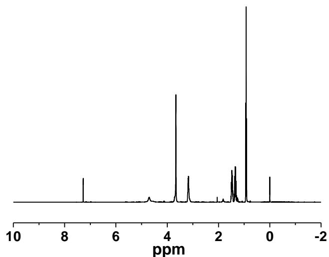
**Fig. S23** <sup>1</sup>H NMR spectra of methyl butyl carbamate.
