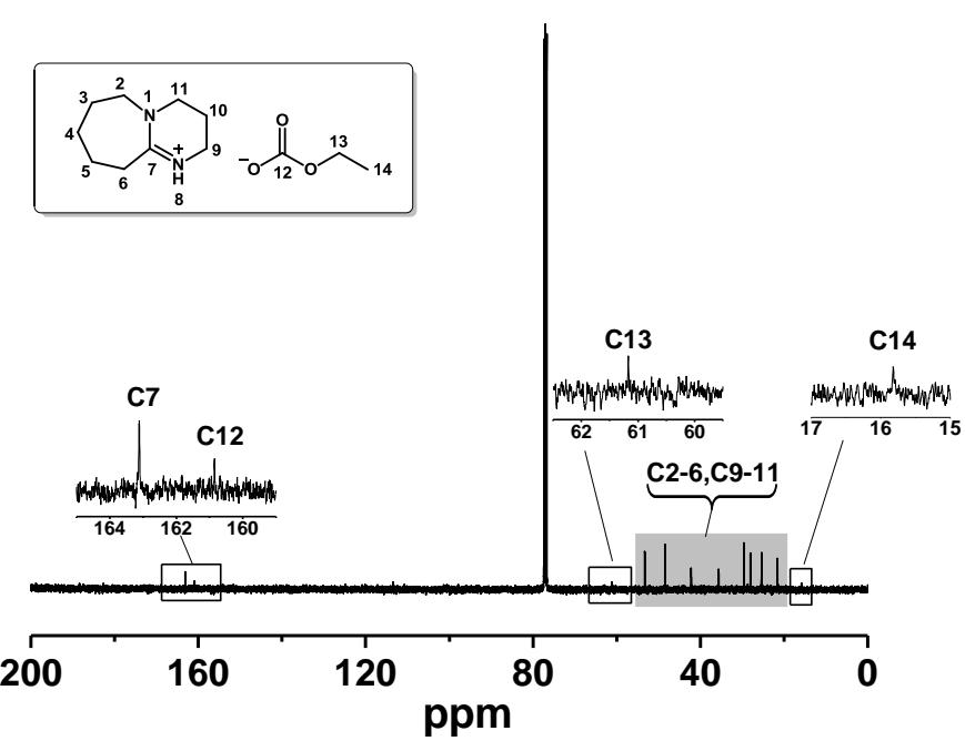
**Fig. S5**  $^{13}\text{C}$  NMR ( $\text{CDCl}_3$  as a solvent) spectra of  $[\text{DBUH}][\text{O}(\text{CO})\text{OCH}_2\text{CH}_3]$ .
