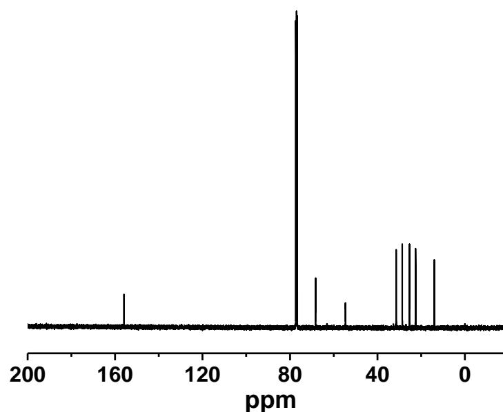
**Fig. S12** <sup>13</sup>C NMR spectra of hexyl methyl carbonate.
