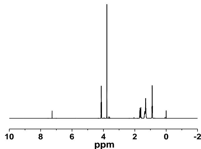
**Fig. S11** <sup>1</sup>H NMR spectra of hexyl methyl carbonate.
