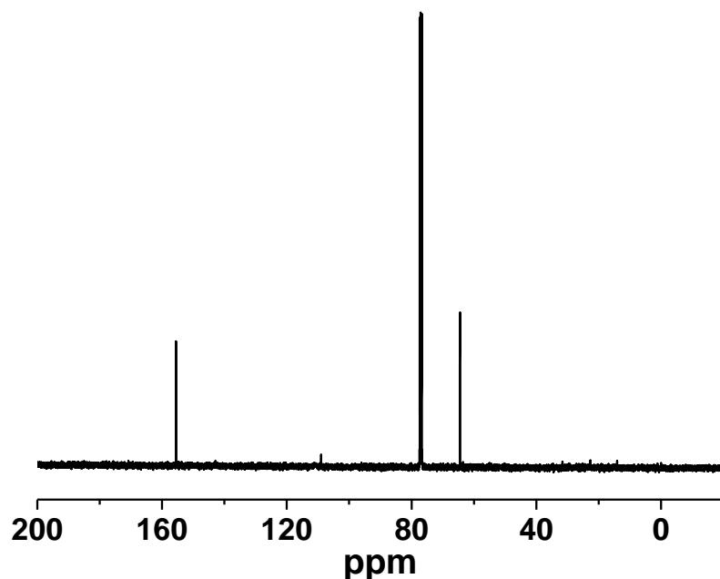
**Fig. S16** <sup>13</sup>C NMR spectra of 1,3-dioxolan-2-one.
