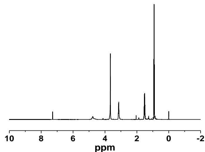
**Fig. S19** <sup>1</sup>H NMR spectra of methyl propyl carbamate.
