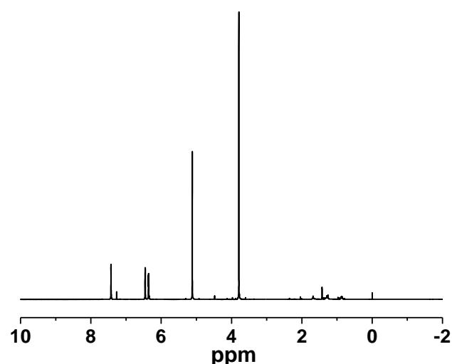
**Fig. S17**  $^1\text{H}$  NMR spectra of furan-2-ylmethyl methyl carbonate.
