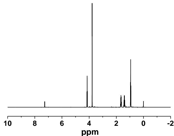
**Fig. S9** <sup>1</sup>H NMR spectra of butyl methyl carbonate.
