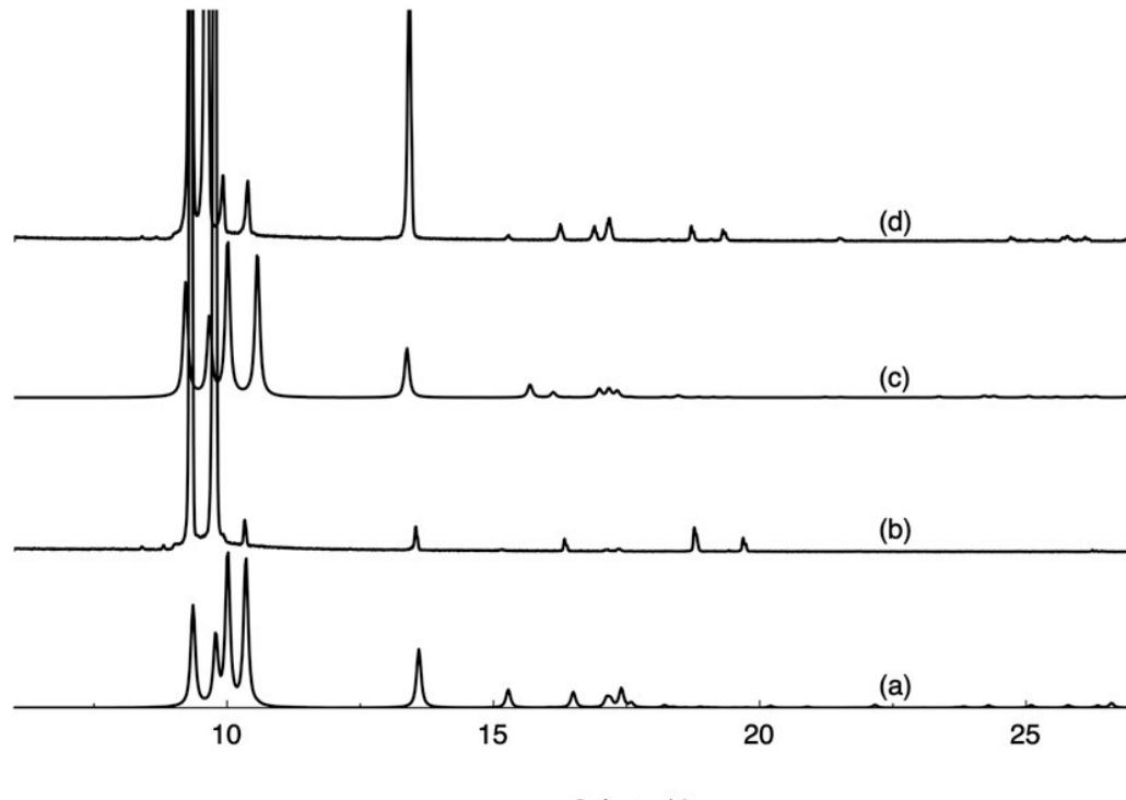
**Figure S1:** Comparison of the simulated (a)  $(1-2H)_2\text{-}[Re_6S_8(CN)^6]$  and (c)  $(1-2H)_2\text{-}[Re_6Se_8(CN)^6]$ , and recorded PXRD patterns for (b)  $(1-2H)_2\text{-}[Re_6S_8(CN)^6]$  (b)  $(1-2H)_2\text{-}[Re_6Se_8(CN)^6]$ , (d). Discrepancies in intensity between the observed and simulated patterns are due to preferential orientations of the microcrystalline powders.
