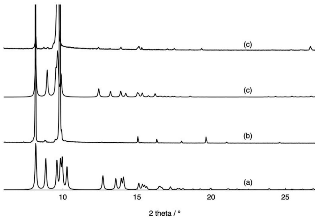
**Figure S2:** Comparison of the simulated (a)  $(2-2H)_2\text{-}[Re_6S_8(CN)^6]$  and (c)  $(2-2H)_2\text{-}[Re_6Se_8(CN)^6]$  and recorded PXRD patterns for (b)  $(2-2H)_2\text{-}[Re_6S_8(CN)^6]$  (b) and  $(2-2H)_2\text{-}[Re_6Se_8(CN)^6]$  (d). Discrepancies in intensity between the observed and simulated patterns are due to preferential orientations of the microcrystalline powders.
