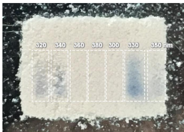
Fig. S5 Photoresponse range of ZnLCl upon irradiation of UV light at characteristic wavelength (nm). Every spot was irradiated for 1 min.
