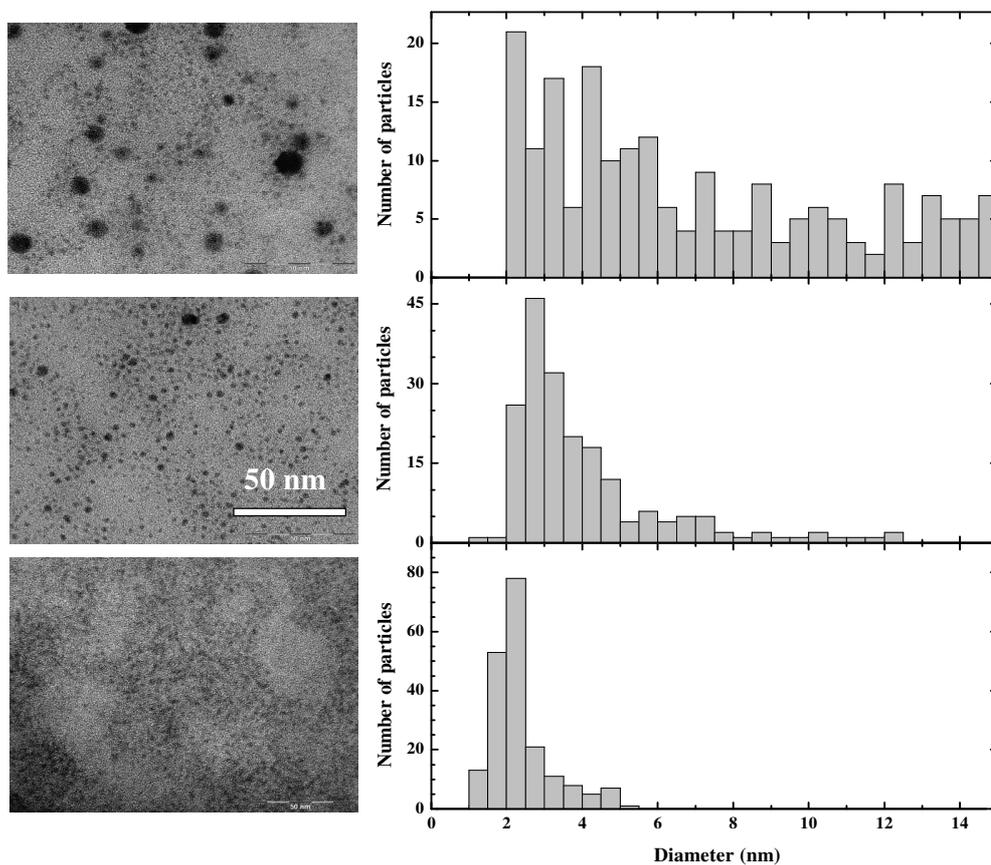
**Figure S2.** TEM micrographs and size distribution of silver nanoparticles obtained by total  $\gamma$ -reduction of ethanolic solutions containing  $5 \times 10^{-5}$  M calix[8]arene **5** and different concentrations of  $\text{AgClO}_4$ : **(top)**  $1 \times 10^{-3}$  M (dose 1440 Gy), **(middle)**  $7.5 \times 10^{-4}$  M (dose 1080 Gy), **(bottom)**  $5 \times 10^{-4}$  M (dose 720 Gy). The scale is the same for the three micrographs.
