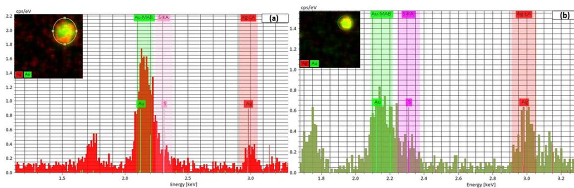
**Figure S7.** EDX spectra of gold-silver nanoparticles obtained by total  $\gamma$ -reduction (dose 1440 Gy) of ethanolic solutions containing  $5 \times 10^{-5}$  M calix[8]arene **5**,  $2.5 \times 10^{-4}$  M H<sub>2</sub>SO<sub>4</sub> and  $2.5 \times 10^{-4}$  M AgBF<sub>4</sub>
