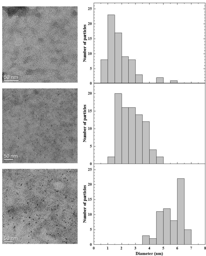
**Figure S3.** TEM micrographs and size distribution of silver nanoparticles obtained by total  $\gamma$ -reduction (dose 720 Gy) of ethanolic solutions containing  $5 \times 10^{-5}$  M calix[8]arene 5 and  $5 \times 10^{-4}$  M silver salt : **(top)**  $\text{AgPF}_6$ , **(middle)**  $\text{AgOTf}$ , **(bottom)**  $\text{AgBF}_4$ .
