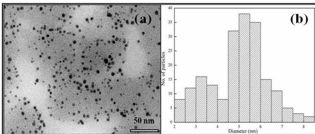
**Figure S4.** (a) TEM micrographs and (b) size distribution of gold nanoparticles obtained by total  $\gamma$ -reduction (dose 2160 Gy) of ethanolic solutions containing  $5 \times 10^{-5}$  M calix[8]arene **5** and  $5 \times 10^{-4}$  M  $\text{HAuCl}_4$ .
