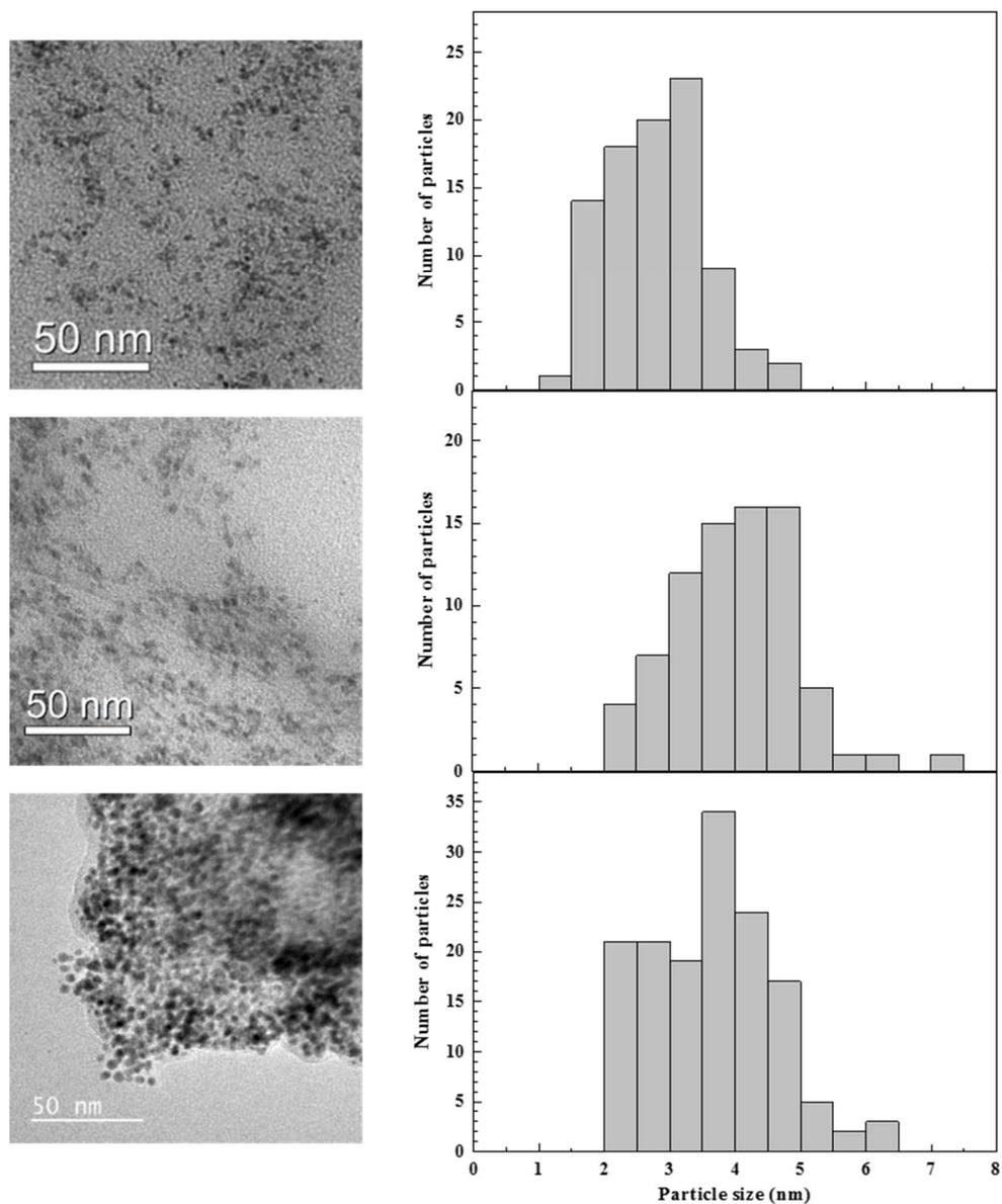
**Figure S5.** TEM micrographs and size distribution of gold-silver nanoparticles obtained by total  $\gamma$ -reduction (dose 1440 Gy) of ethanolic solutions containing  $5 \times 10^{-5}$  M calix[8]arene **5**,  $2.5 \times 10^{-4}$  M H<sub>2</sub>AuCl<sub>4</sub> and  $2.5 \times 10^{-4}$  M silver salt: **(top)** AgPF<sub>6</sub>, **(middle)** AgOTf, **(bottom)** AgClO<sub>4</sub>.
