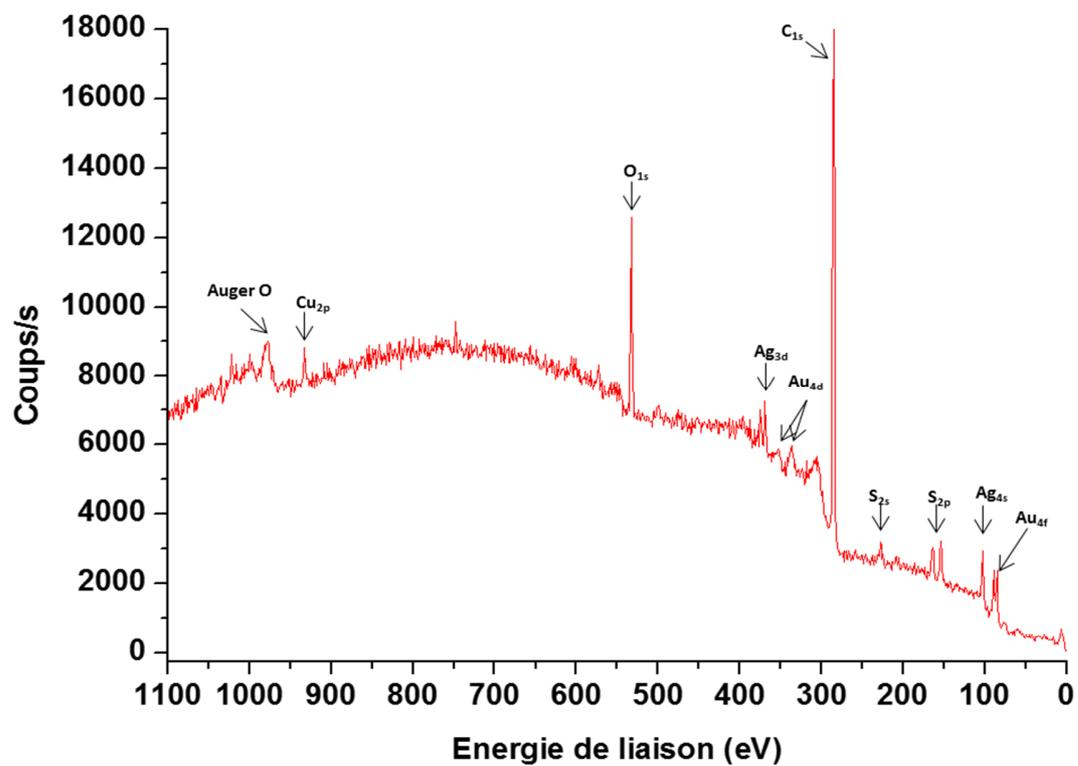
**Figure S6.** XPS spectrum of gold-silver nanoparticles obtained by total  $\gamma$ -reduction (dose 1440 Gy) of ethanolic solutions containing  $5 \times 10^{-5}$  M calix[8]arene **5**,  $2.5 \times 10^{-4}$  M H<sub>2</sub>AuCl<sub>4</sub> and  $2.5 \times 10^{-4}$  M AgClO<sub>4</sub>
