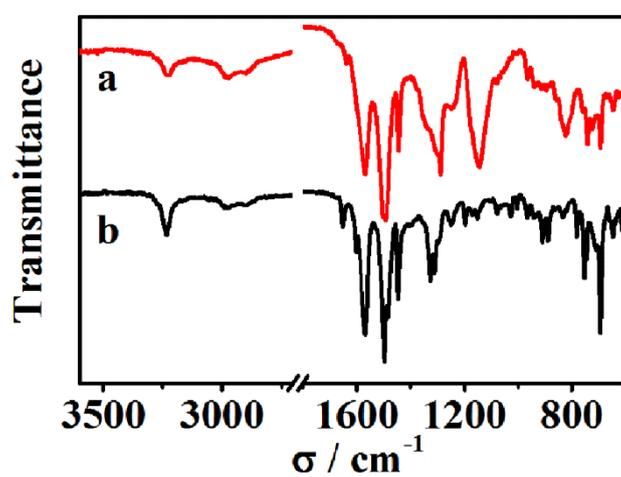
Fig.S5 FT-IR spectra of PANI synthesized in the presence (a) or absence (b) of Fc.
