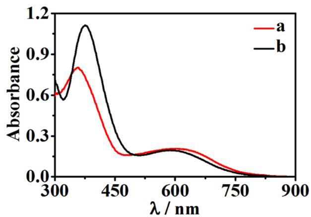
Fig.S6 Absorption spectra of PANI synthesized in the presence (a) or absence (b) of Fc.
