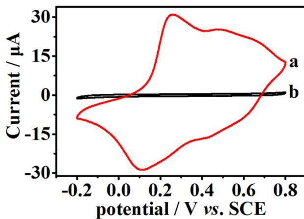
Fig.S7 Cyclic voltammogram of (b) the bare GCE or (a) in the presence of a PANI film.
