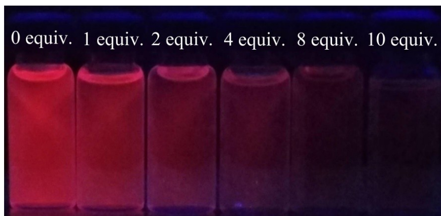
Fig. S10 Fluorescence of I 1 /16 without and with C 70 in CHCl 3 under irradiation (365 nm).
