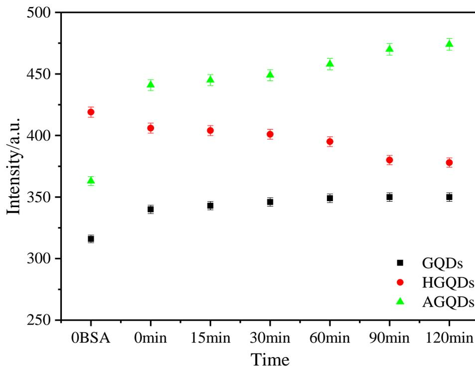
Fig.S5 Fluorescence spectra intensity changes of three kinds of composite probes of graphene quantum dots with BSA in different incubation time.
