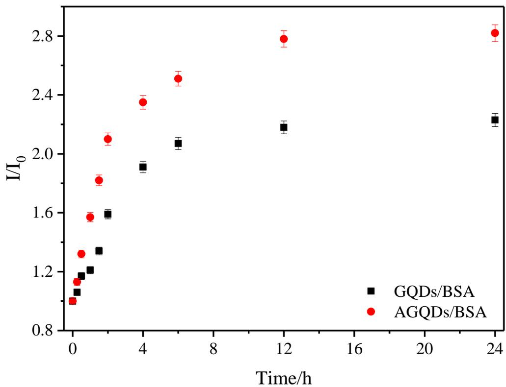
Fig.S6 Fluorescence spectra intensity changes of GQDs/BSA and A GQDs/BSA in different incubation time when detecting trypsin
