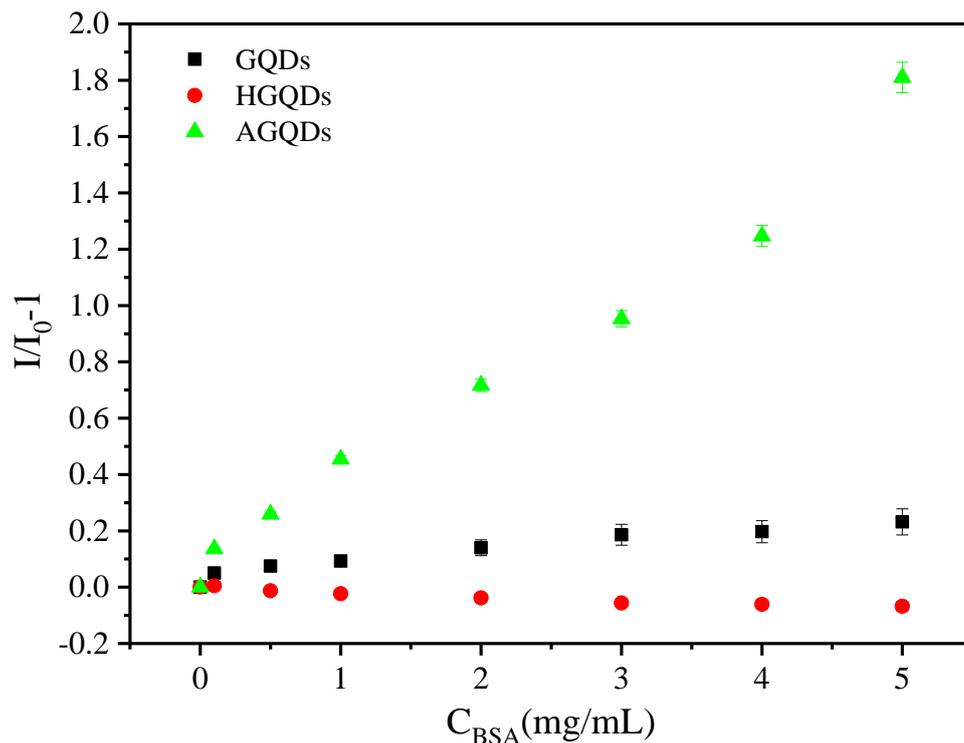
Fig.S4 Fluorescence spectra intensity changes of three kinds of graphene quantum dots in the presence of different BSA concentration.
