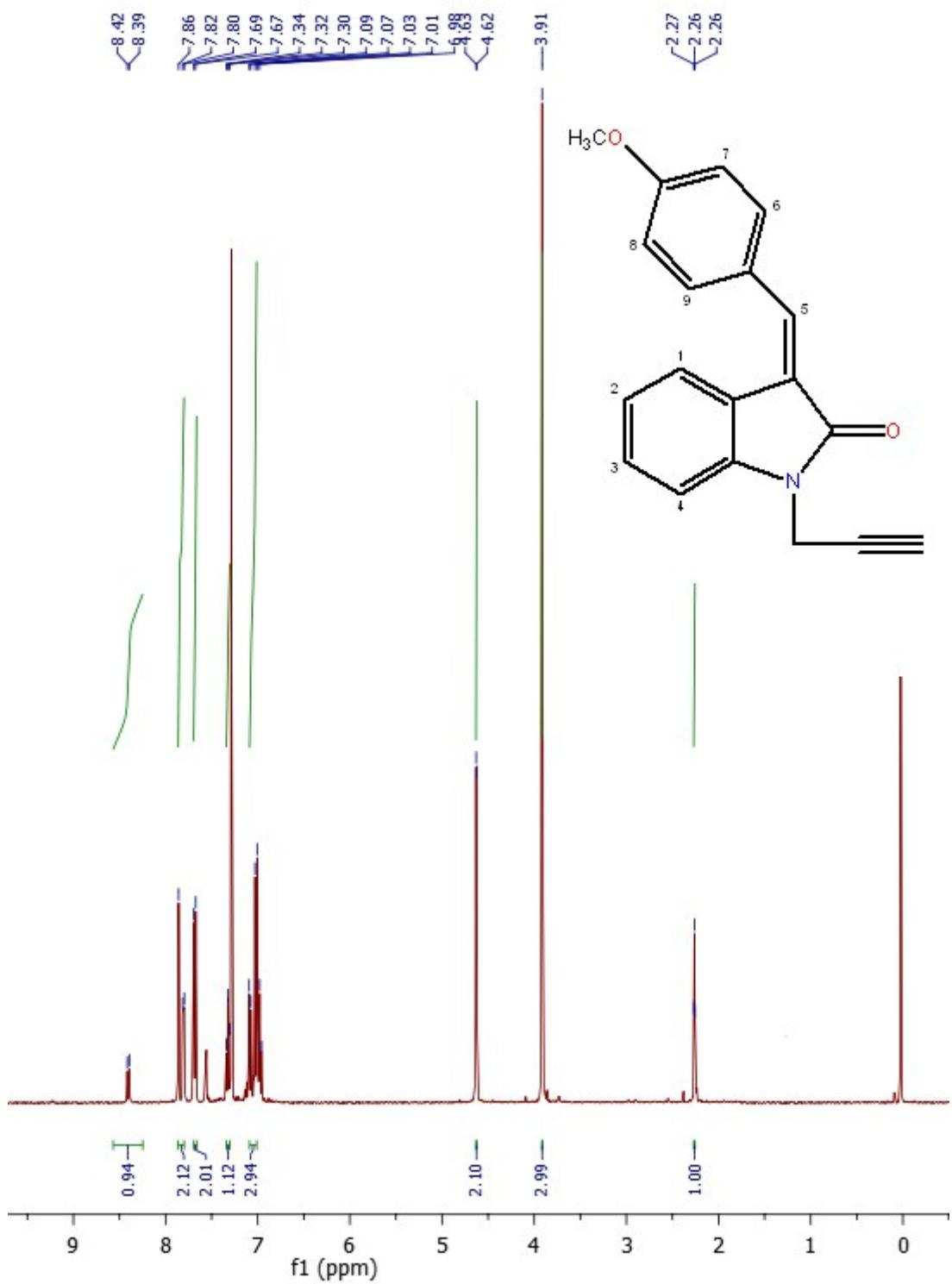
Fig. S9. <sup>1</sup>H NMR Spectra of Compound 4e
