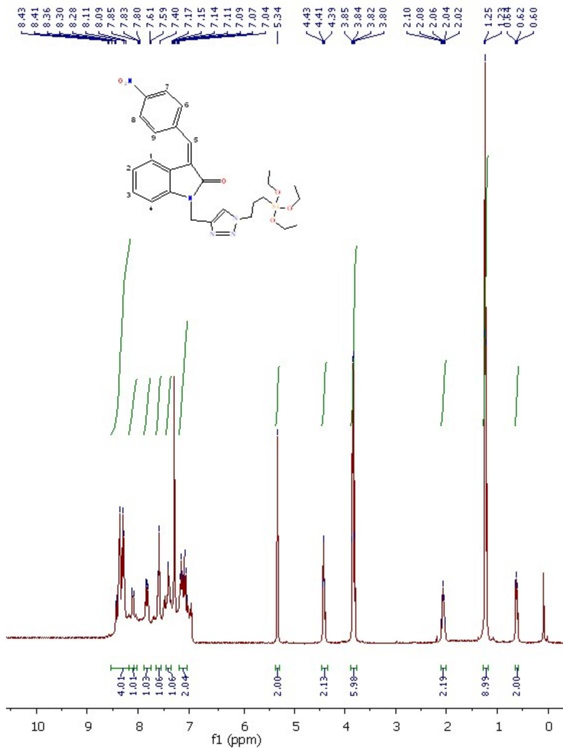
**Fig. S17. <sup>1</sup>H NMR Spectra of Compound 5d.**
