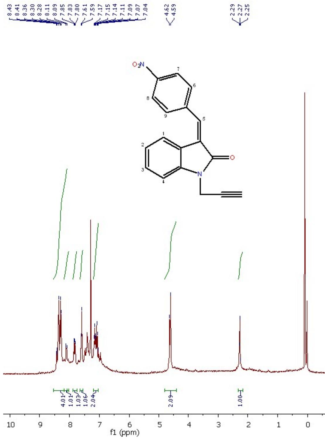
**Fig. S7. <sup>1</sup>H NMR Spectra of Compound 4d**
