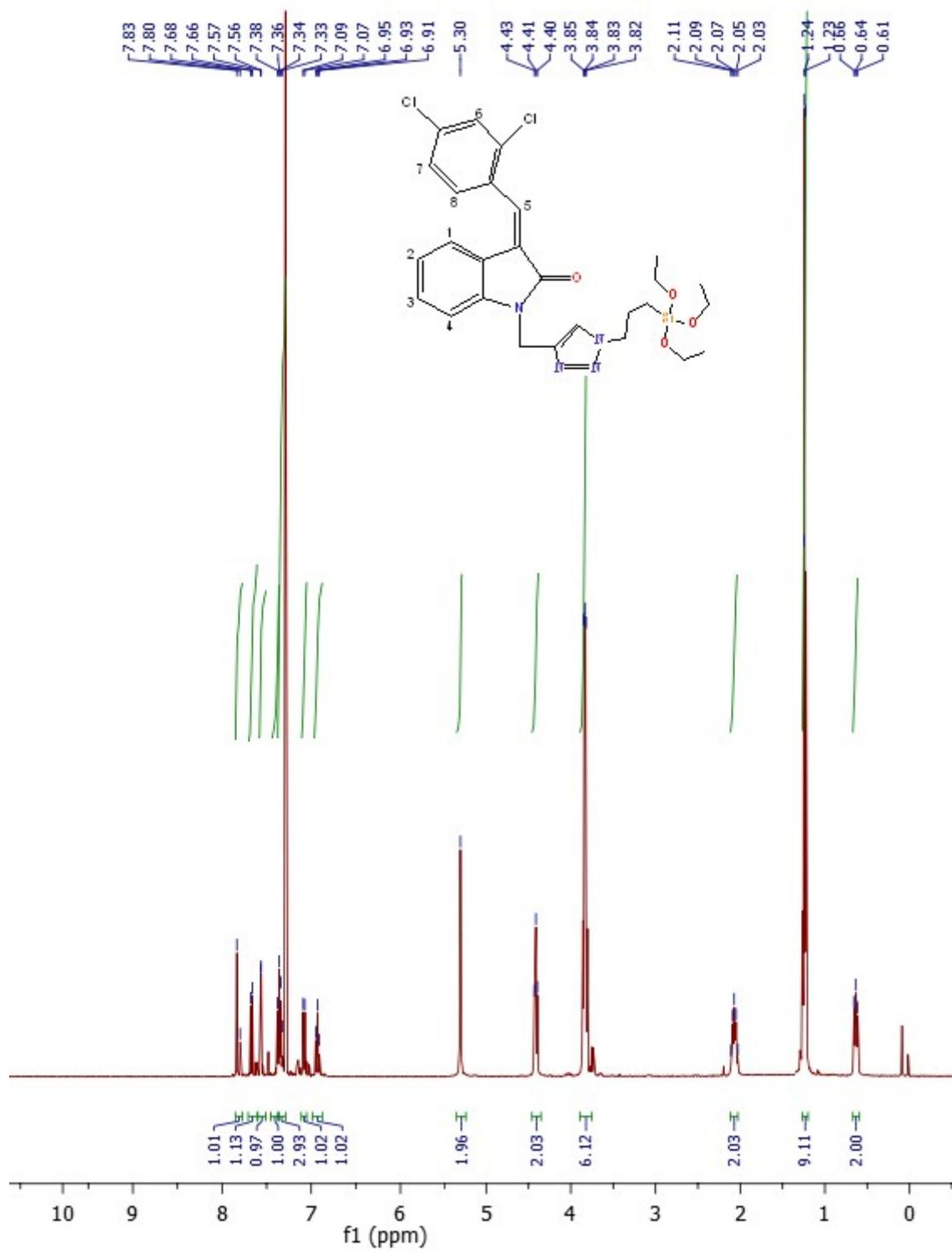
Fig. S13. <sup>1</sup>H NMR Spectra of Compound 5b.
