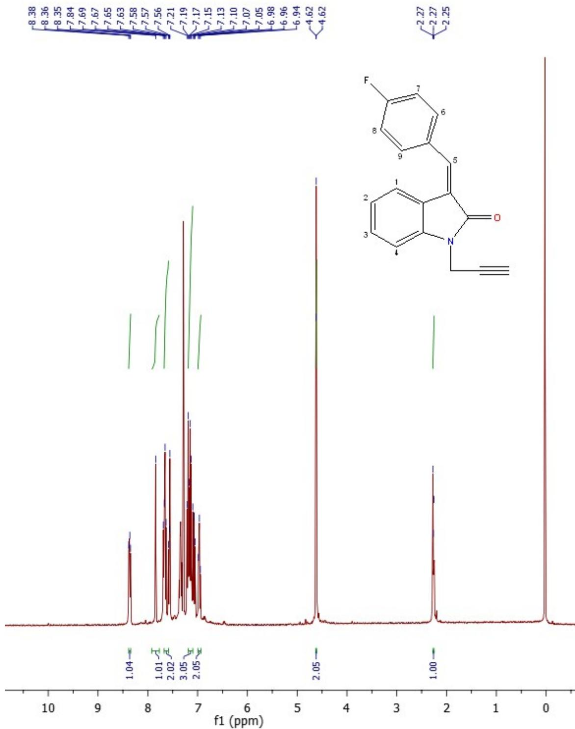
Fig. S1. <sup>1</sup>H NMR Spectra of Compound 4a
