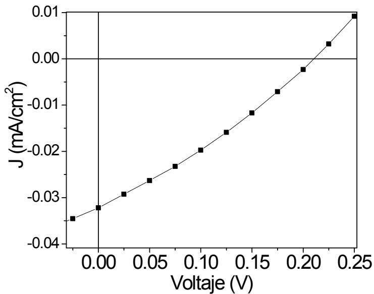
**Figure S36.** a) J-V curve of a solar cell in configuration: ITO/PEDOT/P3HT+**2**/TiO<sub>2</sub>/FM
