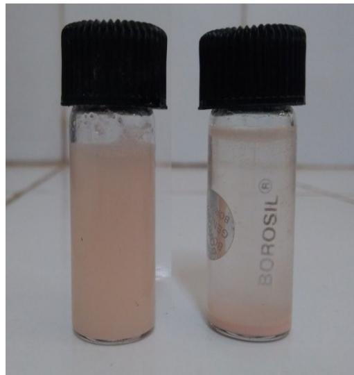
**Figure S1.** The phenomenon of the multicomponent reaction between Isatin, Malononitrile and Dimedone. (A) The reaction mixture at the completion of the reaction. (B) The product precipitated after allowed the reaction to stand.
