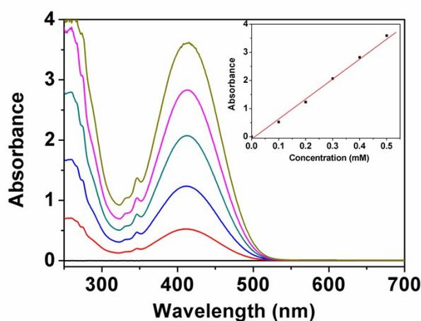
**Fig. S1** Solubility evaluation of **Nap-Se** in pure water by absorption spectra. Inset: Plots of absorption intensity at 410 nm vs probe concentrations (0-0.5mM).
