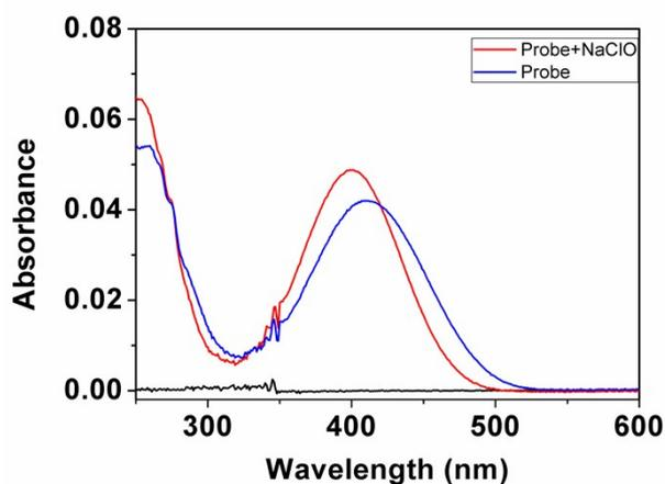
**Fig.S2** Absorption spectra changes of Nap-Se ( $5 \mu\text{M}$ ) upon addition of 1 equiv NaClO in PBS buffer (20 mM, pH 7.4).
