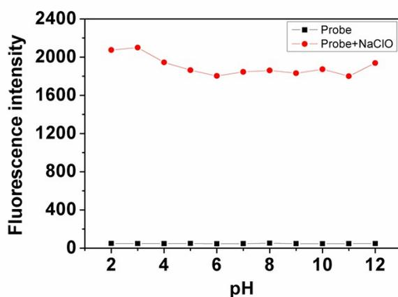
**Fig. S4** pH-dependent experiments of Nap-Se ( $5 \mu\text{M}$ ) with NaClO (10  $\mu\text{M}$ ) at different pH values.
