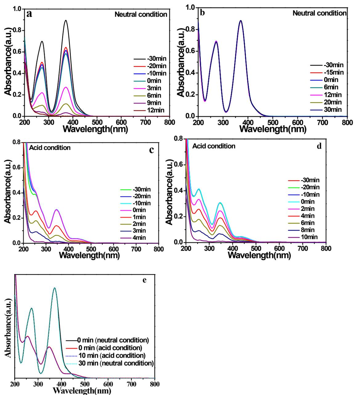
Fig. S4 the UV-Vis absorption spectra of Cr(VI) in presence of BiOCl-110 (a,c), BiOCl-001 (b,d), and in absence of photocatalysts (e) under solar light irradiation.
