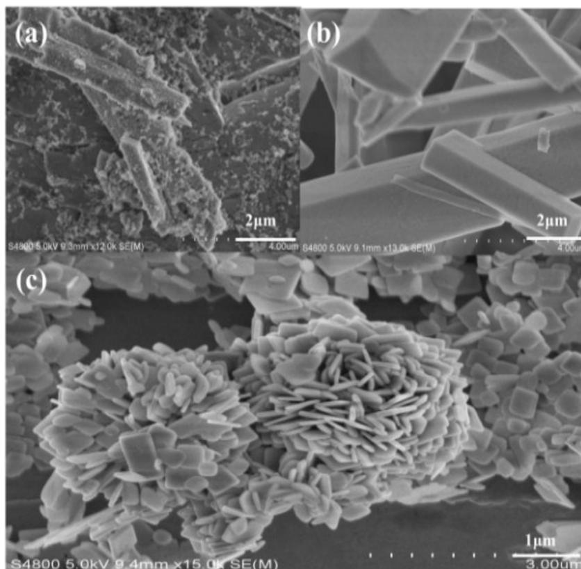
**Fig. S2** SEM images of BiOCl-110 obtained under the different concentrations of reactants (a) 0.5 mmol, (b) 1 mmol, (c) 2 mmol.
