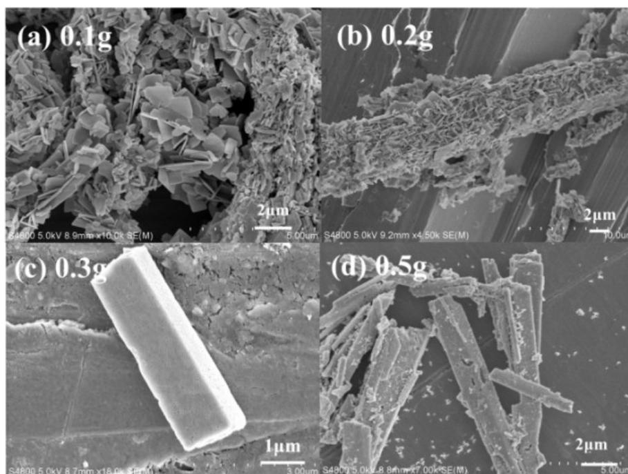
**Fig. S3** SEM images of BiOCl obtained under the different concentrations of sodium citrate, (a) 0.1 g, (b) 0.2 g, (c) 0.3 g and (d) 0.5 g.
