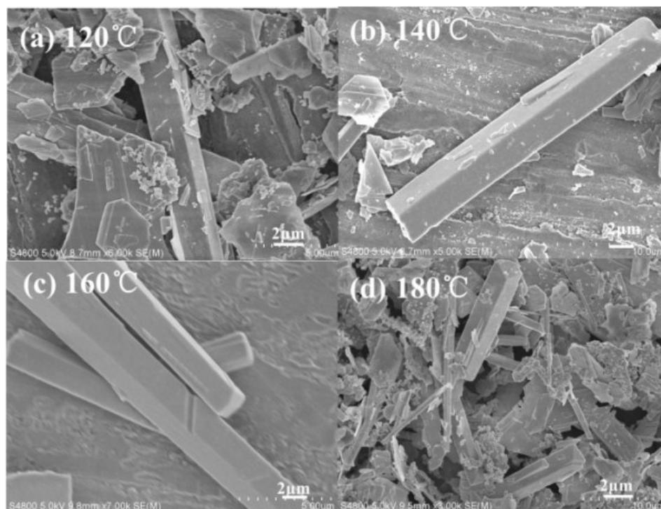
**Fig. S1** SEM images of BiOCl-110 obtained at different reaction temperature (a) 120 °C, (b) 140 °C, (c) 160 °C, (d) 180 °C.
