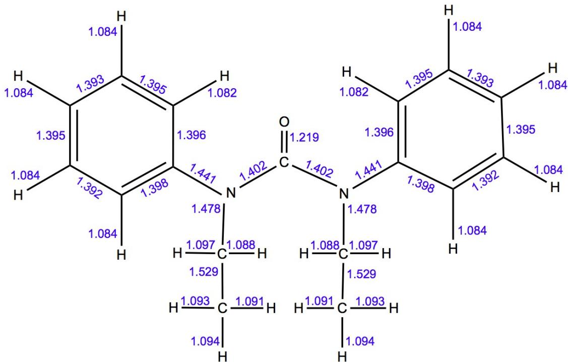
**Figure S9** – The QM bond lengths for EC
