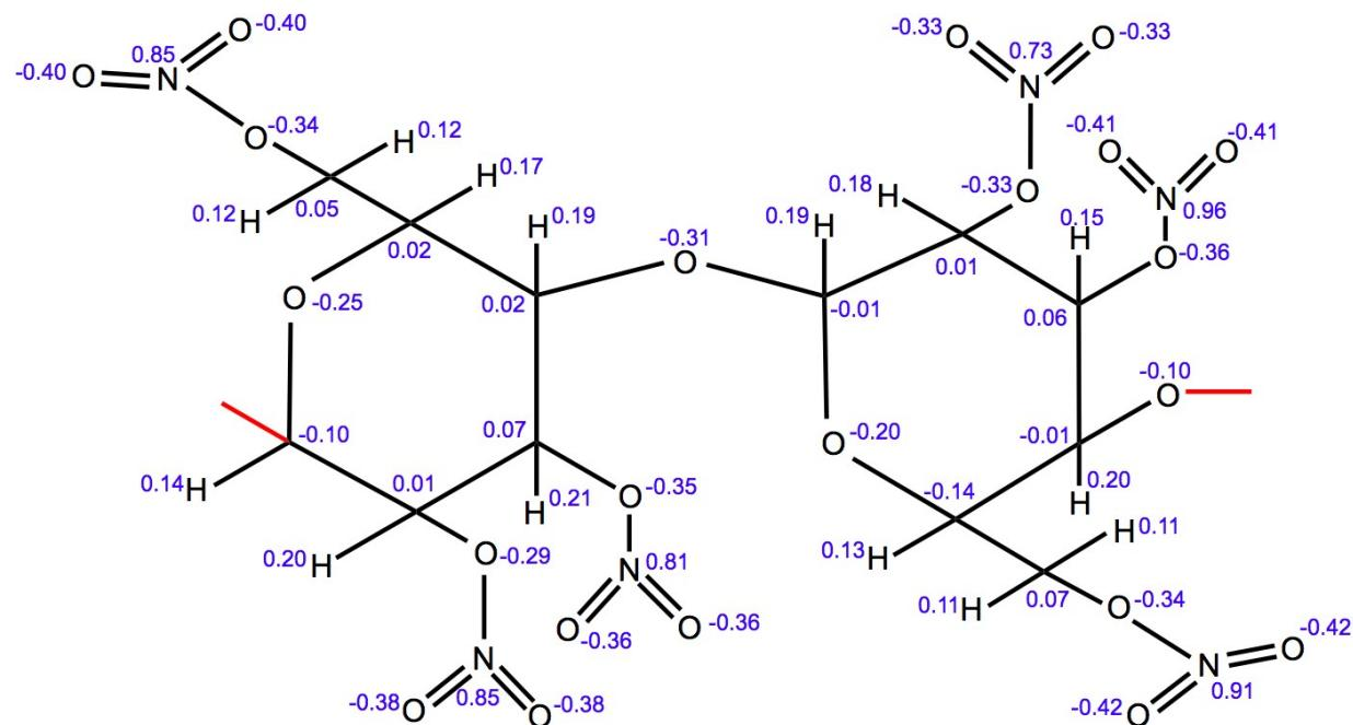
**Figure S3** – The QM derived partial charges for NC
