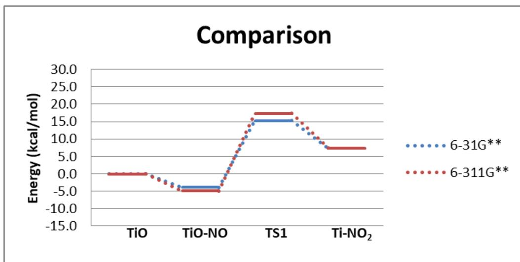
**Table S3.** Activation energies for NO decomposition along the reaction pathways of the low- and high-spin states TiO-por catalyst and the imaginary frequencies.
