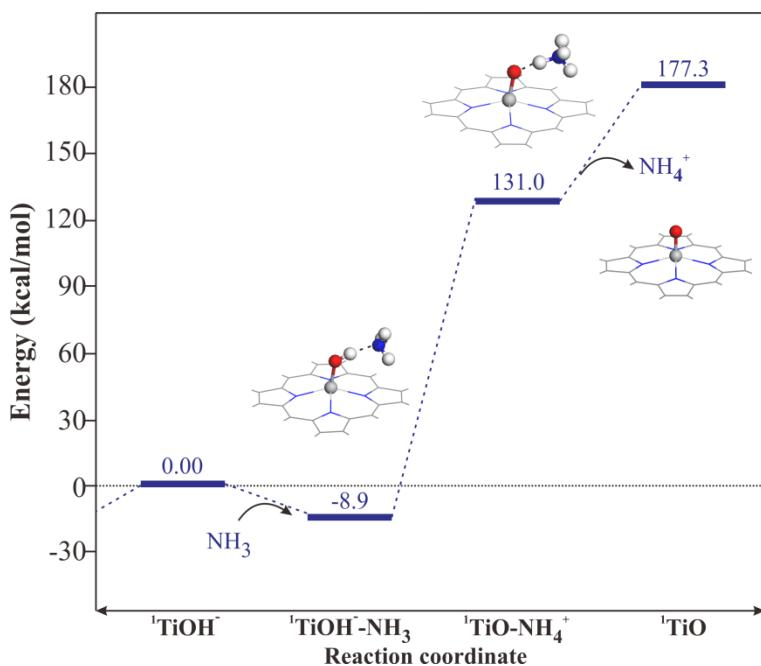
**Figure S2.** Catalyst regeneration by NH<sub>3</sub> reducing agent over the Brønsted site of TiOH intermediate calculated at the low-spin state.
