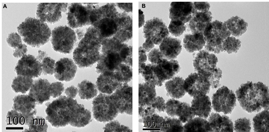
**Fig. S3.** TEM images of Cu-CuFe<sub>2</sub>O<sub>4</sub> NPs: (A) before reaction and (B) after reused six times.
