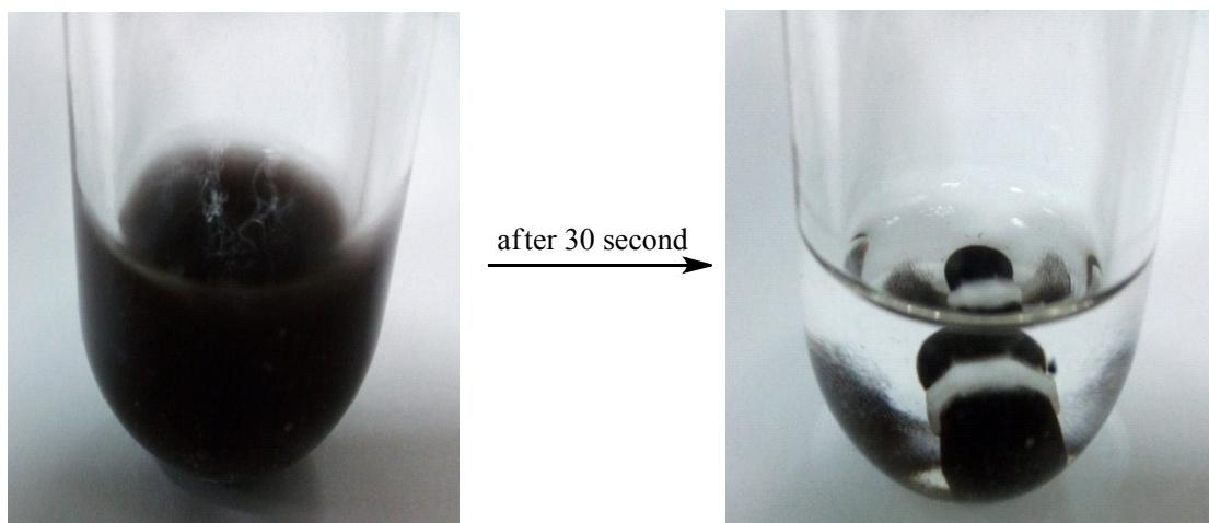
**Fig. S4.** The reusability of Cu-CuFe<sub>2</sub>O<sub>4</sub> catalyst in the hydroboration of alkynes
