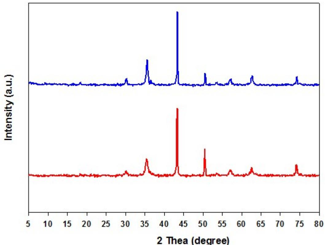
**Fig. S5.** X-ray powder diffractogram of the synthesized Cu-CuFe<sub>2</sub>O<sub>4</sub> nanoparticles (red line) and after reused six times (blue line).
