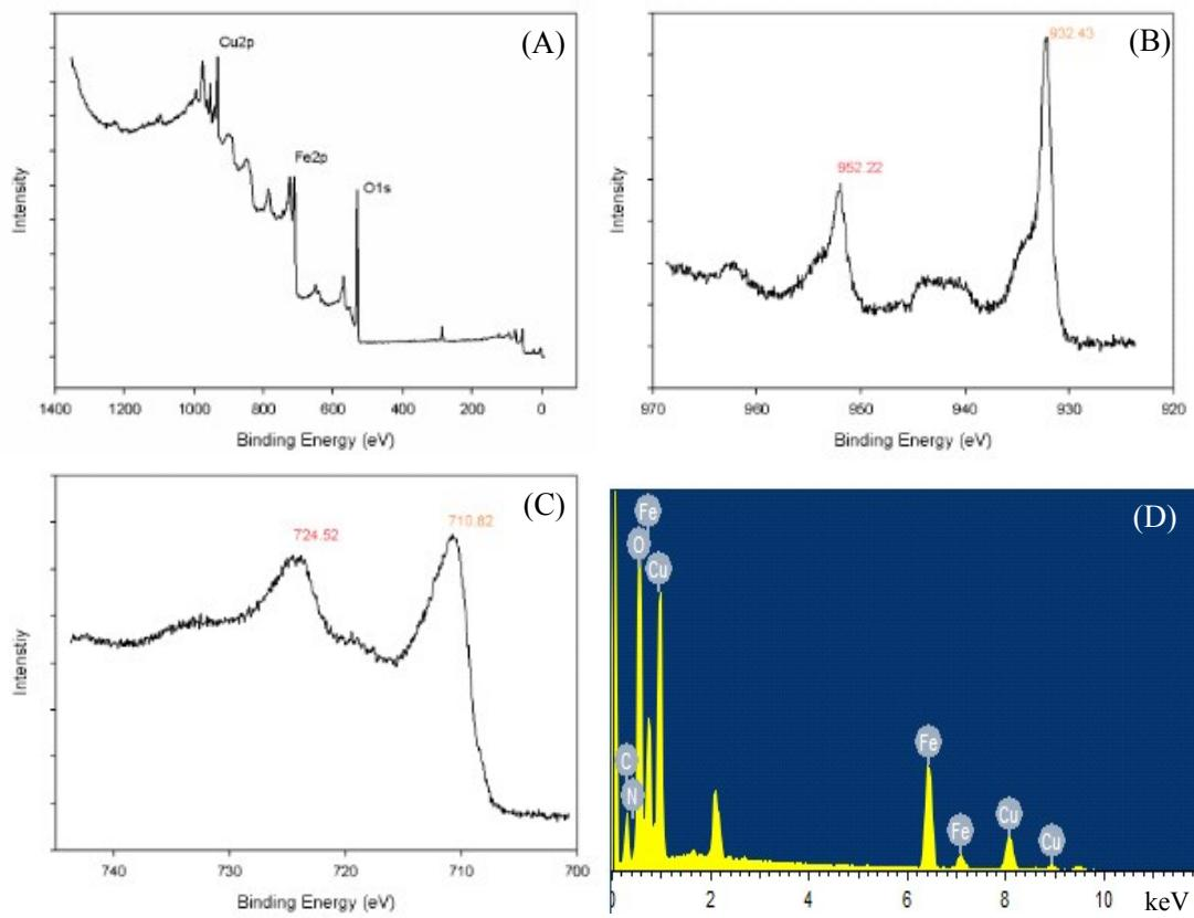
**Fig. S1.** The XPS spectrum of Cu-CuFe<sub>2</sub>O<sub>4</sub> MNPs: (A) survey, (B) Cu 2p, (C) Fe 2p and SEM-EDS of Cu-CuFe<sub>2</sub>O<sub>4</sub> MNPs (D).
