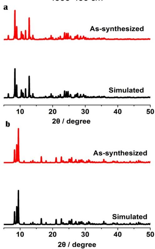
Fig. S3 (a) Powder X-ray diffraction patterns of simulated **1** and as-synthesized; (b) Powder X-ray diffraction patterns of simulated **2** and as-synthesized.
