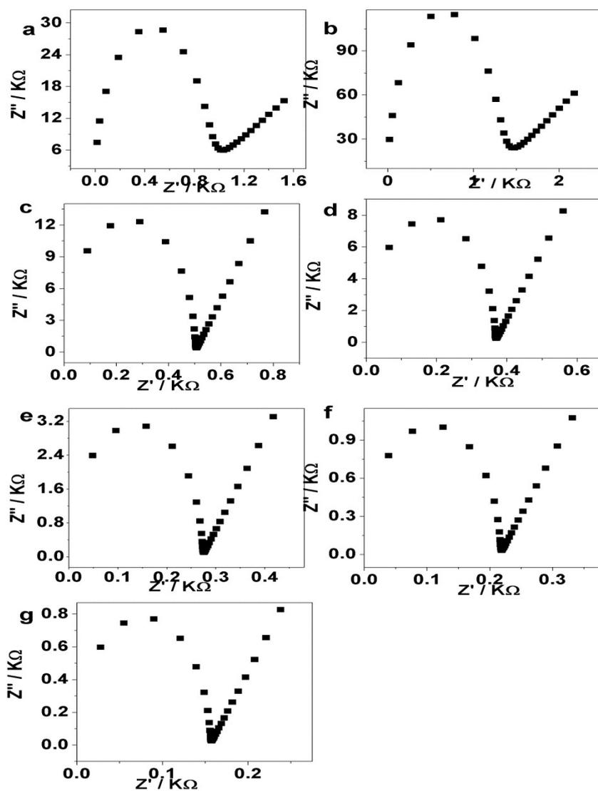
Fig. S7 Nyquist plots of **1** at 97% RH with various temperatures (a) 25 °C, (b) 35°C, (c) 45 °C, (d) 55°C, (e) 65 °C, (f) 75 °C, (g) 85°C
