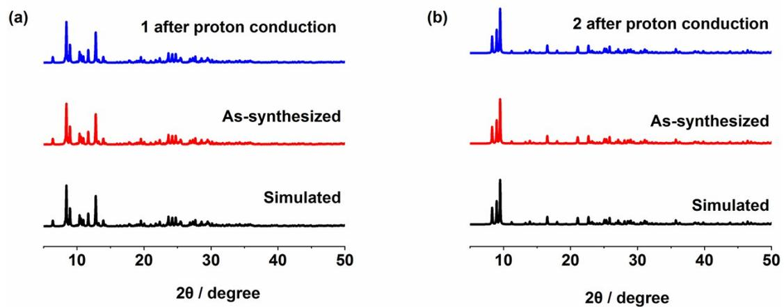
Fig. S11 (a) Powder X-ray diffraction patterns of **1** after proton conduction test; (b) Powder X-ray diffraction patterns of **2** after proton conduction test.
