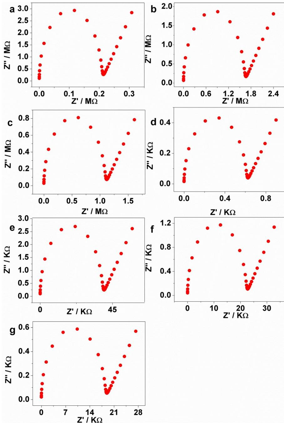
Fig. S10 Nyquist plots of **2** at 25 °C RH with various RH (a) 45%, (b) 55%, (c) 65%, (d) 75%, (e) 85%, (f) 95%, (g) 97%.
