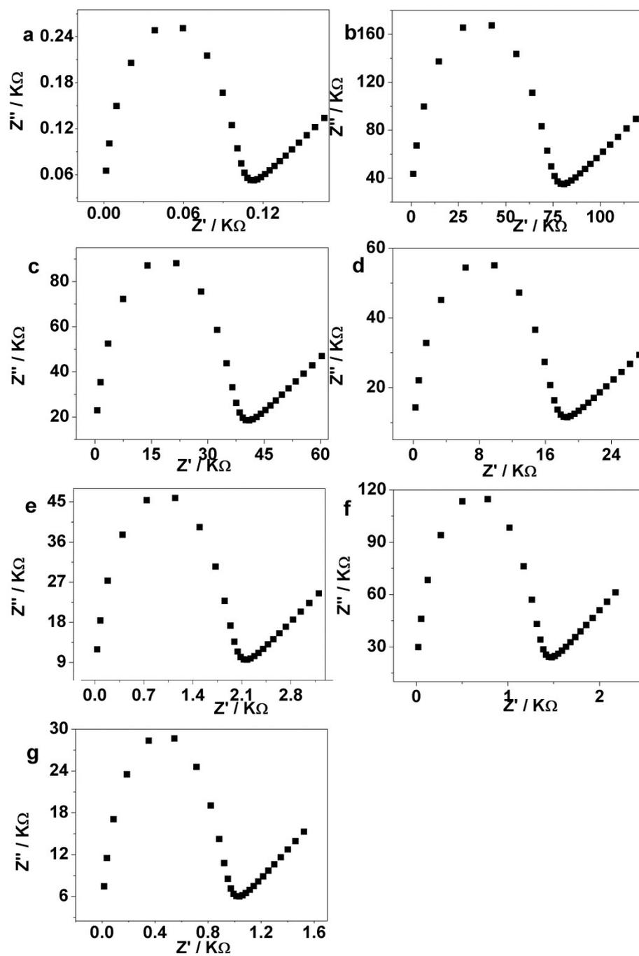
Fig. S8 Nyquist plots of **1** at 25 °C RH with various RH (a) 45%, (b) 55%, (c) 65%, (d) 75%, (e) 85%, (f) 95%, (g) 97%.
