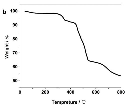
Fig. S5 (a) The thermogravimetric (TG) curves of **1**; (b) The thermogravimetric (TG) curves of **2** measured from 30 to 800 °C under N<sub>2</sub> atmosphere with the heating rate of 10 °C/min.
