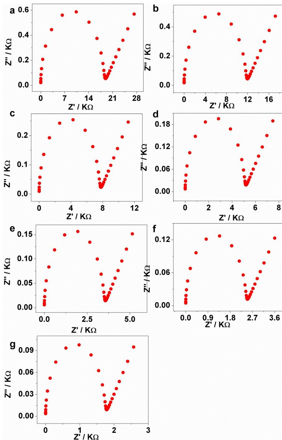
Fig. S9 Nyquist plots of **2** at 97% RH with various temperatures (a) 25 °C, (b) 35°C, (c) 45 °C, (d) 55°C, (e) 65 °C, (f) 75 °C, (g) 85°C
