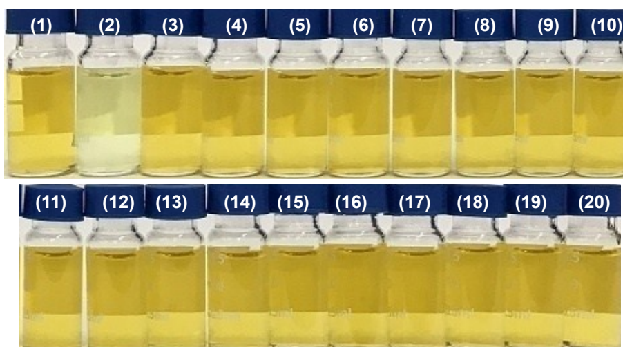
Fig. S11 Colour responses of L-Cu^{2+} ( 10 \mu M ) in HEPES aqueous buffer ( CH_3CN : HEPES = 7:3, 20 mM, pH = 7.4) upon addition of various biothiols and amino acids ( 30 \mu M ): (1) free L-Cu^{2+} , (2) Cys, (3) Ala, (4) Asp, (5) Gln, (6) Gly, (7) Hcy, (8) Lys, (9) Phe, (10) Pro, (11) Ser, (12) Thr, (13) Try, (14) Val, (15) Leu, (16) His, (17) Arg, (18) Asn, (19) GSH, (20) Glu.
