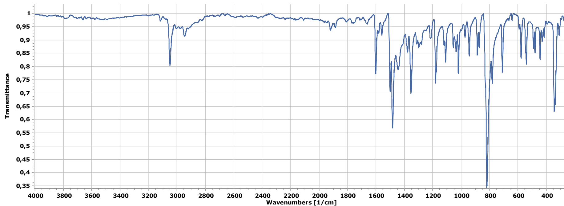
Figure S5. Solid-state IR spectrum (250-4000 \text{cm}^{-1} ) of [\text{PtCl}_2\{\kappa^2N\text{-(HCN(4-C}_6\text{H}_4\text{CH}_3)_2)\}_2] , 3 .
