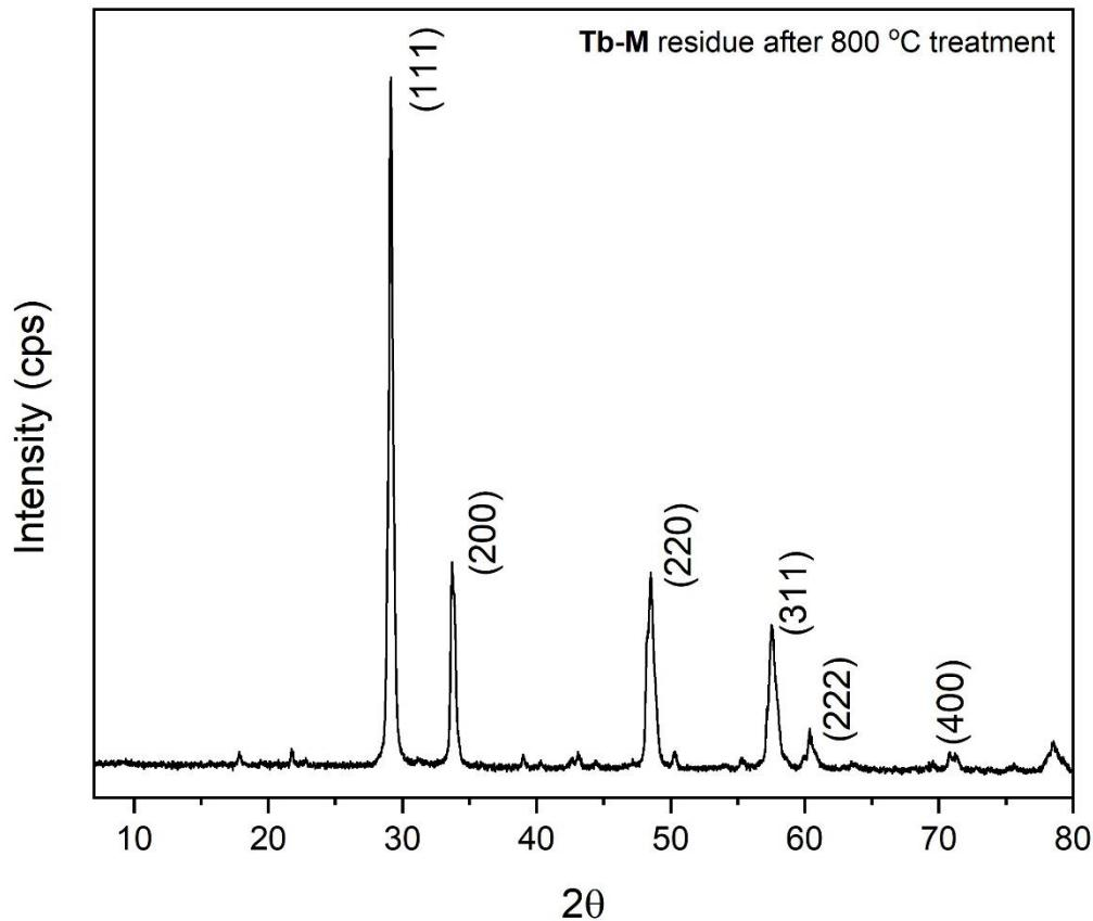
**Fig. S10.** XRD pattern of **Tb-M** residue after 800 °C treatment showing  $\text{Tb}_4\text{O}_7$  characteristic peaks.
