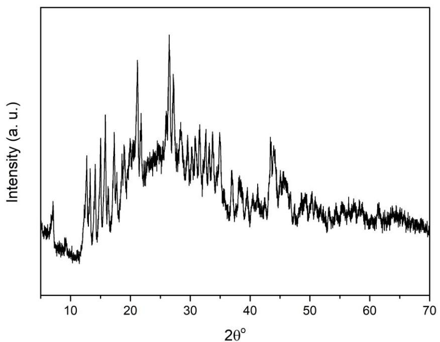
**Fig. S6.** Powder X-ray diffraction pattern of **Tb-MHT** synthesized with pH = 4.0 by hydrothermal technique, 72 h at 150 °C and 36 h of cooling to room temperature.
