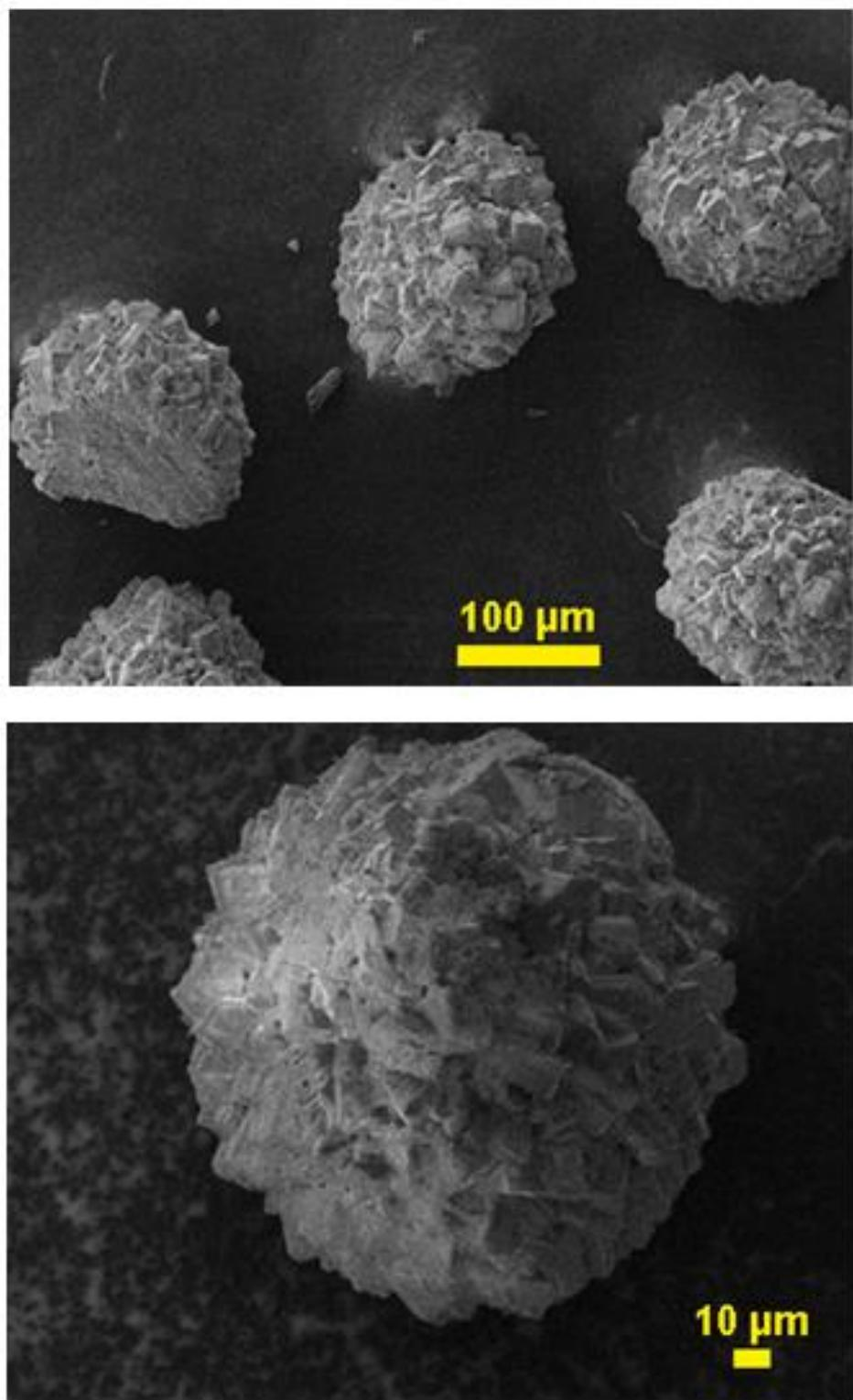
**Fig. S5.** FEG-SEM images of **Tb-MHT** synthesized with  $\text{pH} = 4.0$  by hydrothermal technique, with 72 h at  $150^\circ\text{C}$  and 36 h of cooling to room temperature.
