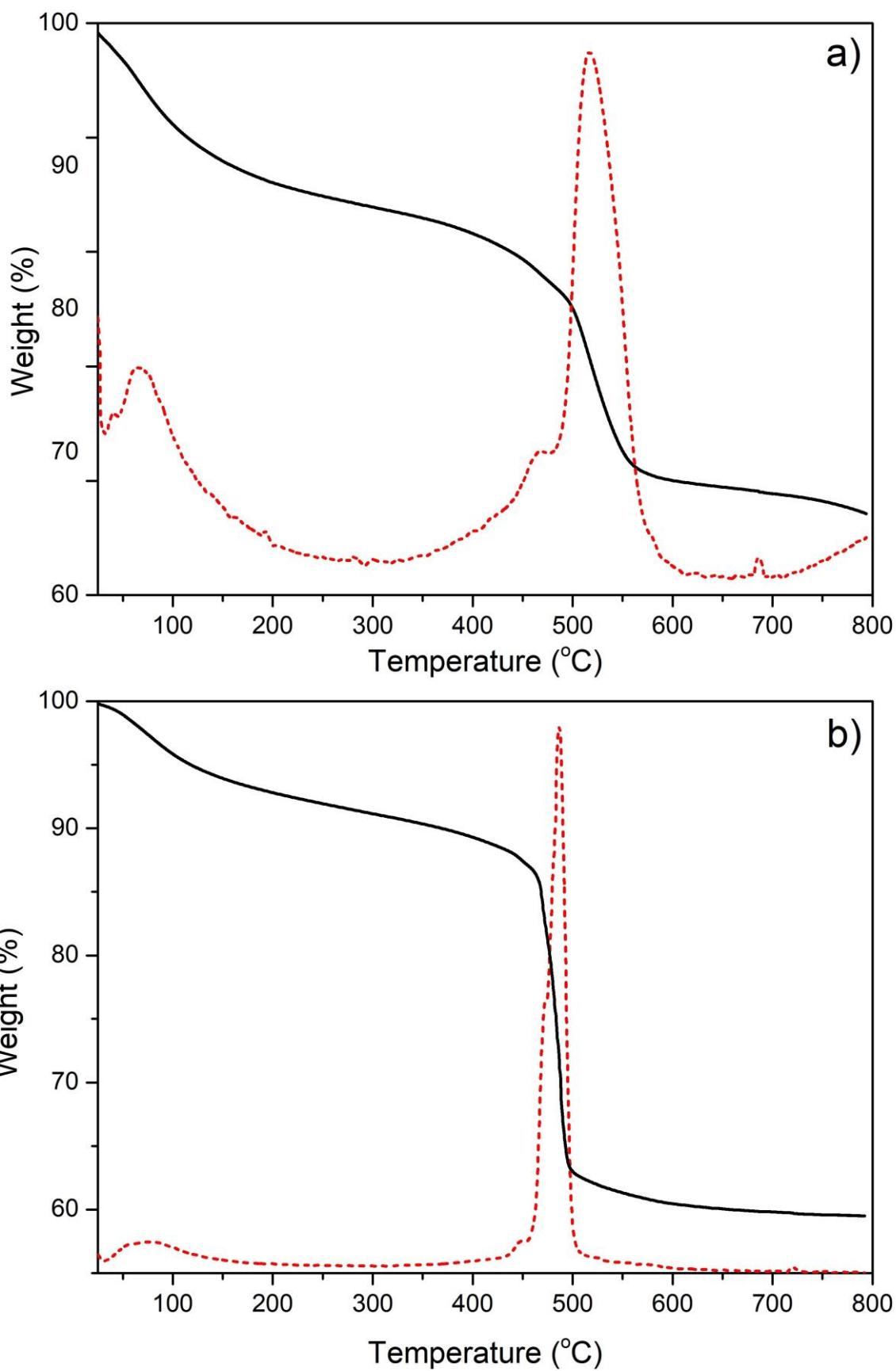
**Fig. S9.** TG/DTG curves of as-synthesized **Tb-M** (a) and after activation (b).
