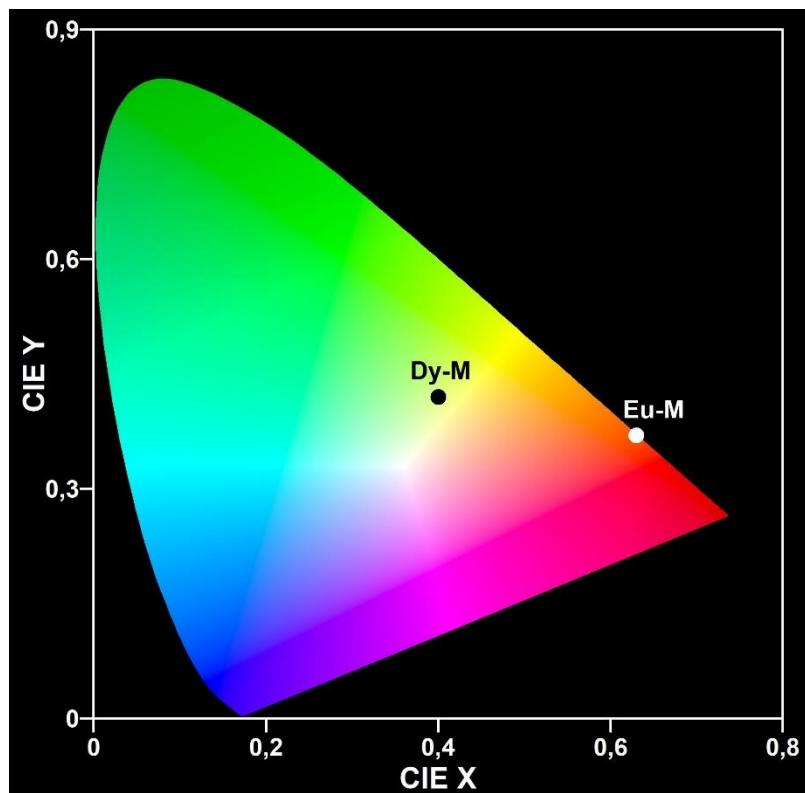
**Fig. S12.** CIE chromaticity diagram for **Eu-M** (0.63, 0.37) and **Dy-M** (0.40, 0.42) samples.
