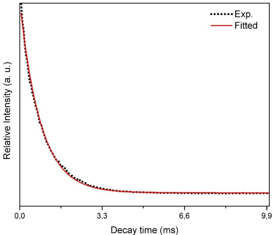
**Fig. S11.** Decay time curves of **Tb-M**.
