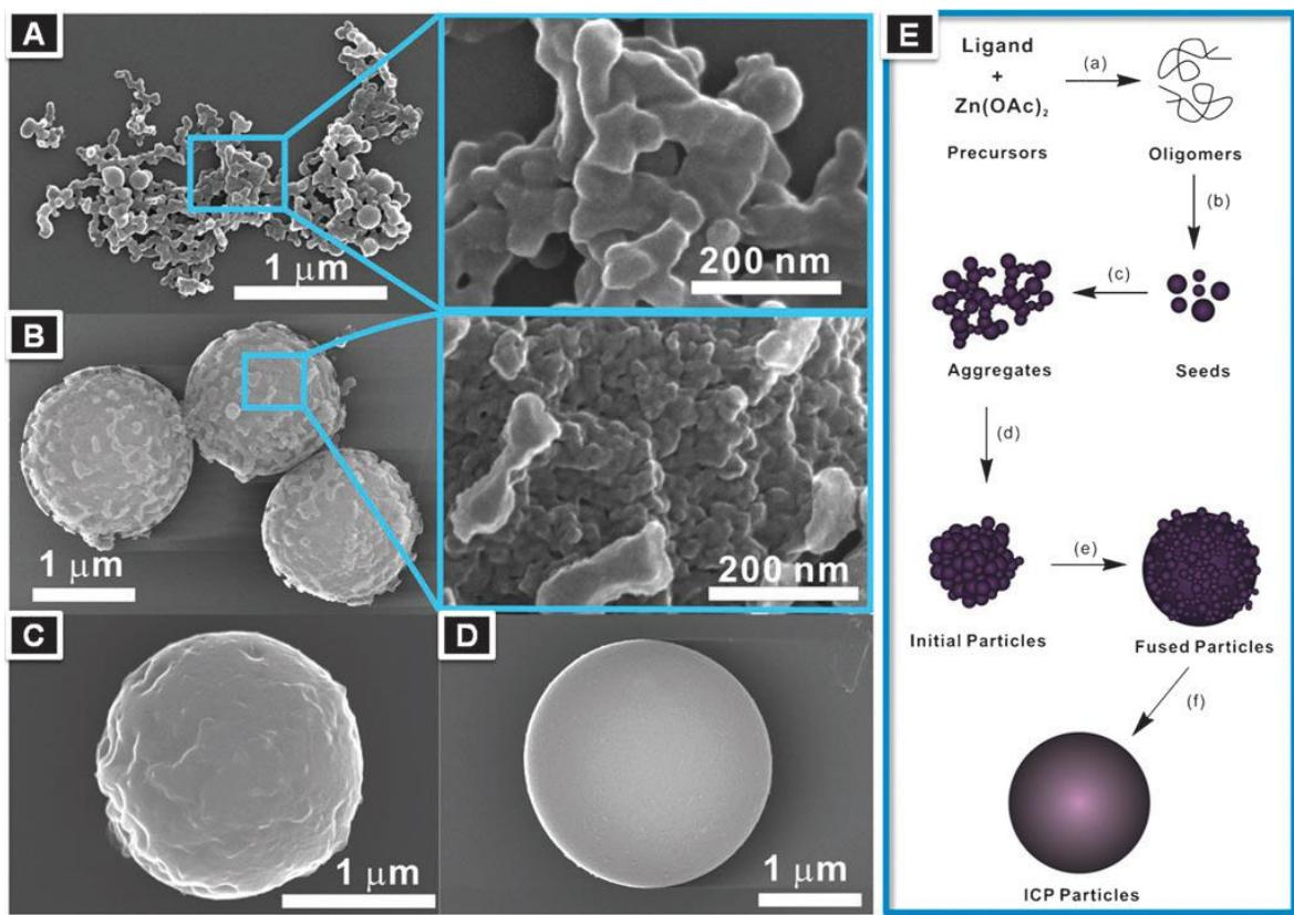
**Fig. S4.** Proposed mechanism of the formation of the spherical particles for an analogous Zn-based ICP. Reproduced from Ref. 1 with permission from The Royal Society of Chemistry.
