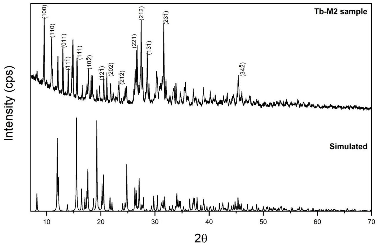
**Fig. S2.** Powder XRD of **Tb-M2** (top) and simulated data (bottom) (P<sub>2</sub>1/c, CCDC Deposition Number 614527).
