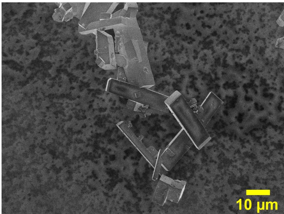
**Fig. S1.** FEG-SEM image of **Tb-M2** synthesized with pH = 2.
