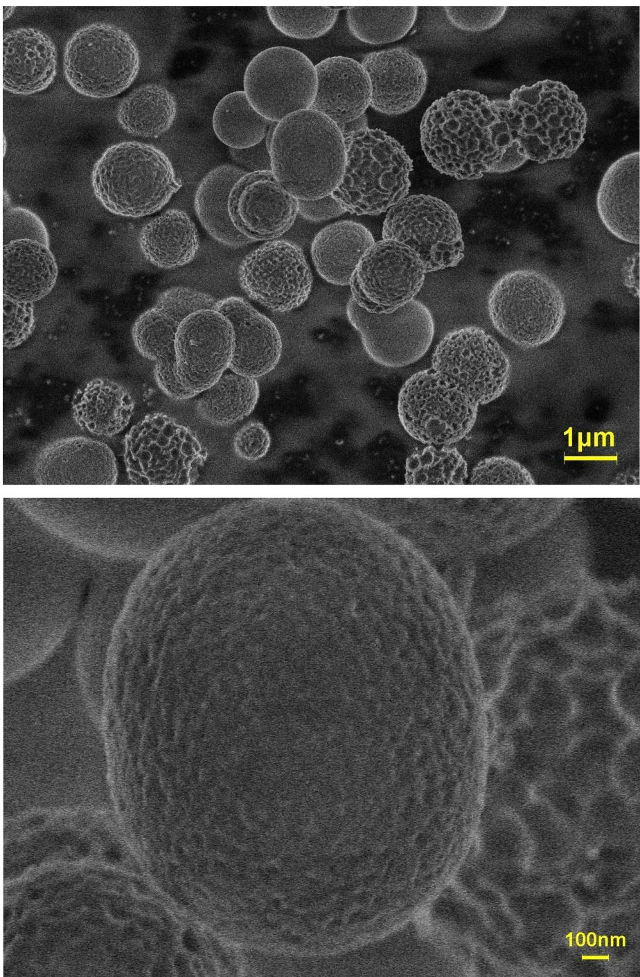
**Fig. S3.** FEG-SEM images of **Tb-M5** synthesized with pH = 5.
