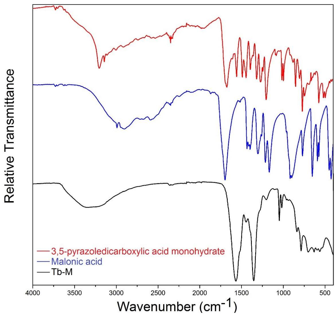
**Fig. S8.** Infrared spectra of the ligands and **Tb-M**.
