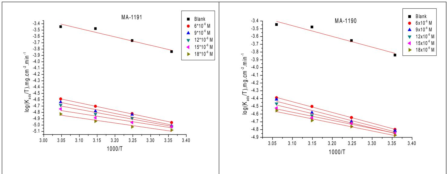
**Fig. 3.** Transition state plots ( $\log k_{corr}$  vs  $1/T$ ) for carbon steel in 1.0 M HCl in absence and presence of different concentration of (MA-1191, MA-1190).
