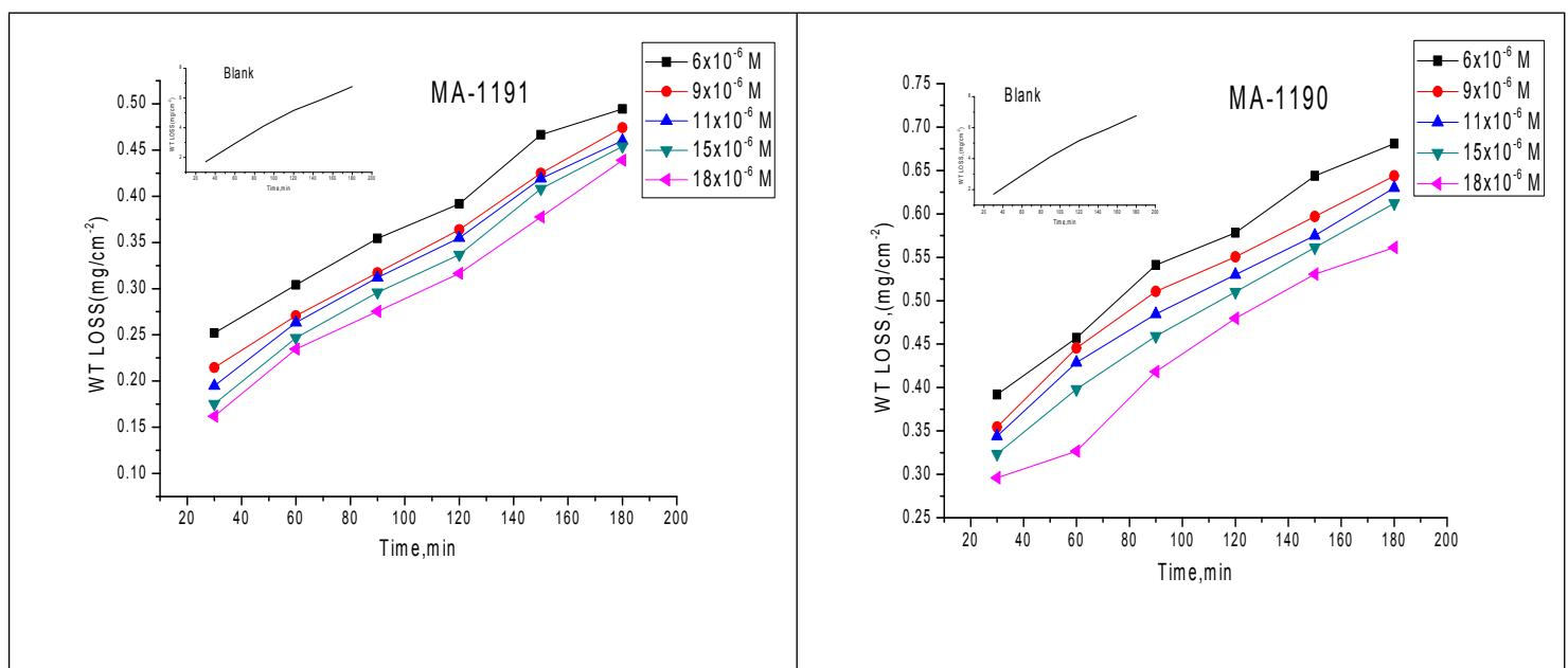
**Fig. S1.** WL-time curves for the dissolution of CS in 1.0 M HCl without and with various concentrations of MA-1191 (left) and MA-1190 (right) at 25°C.
