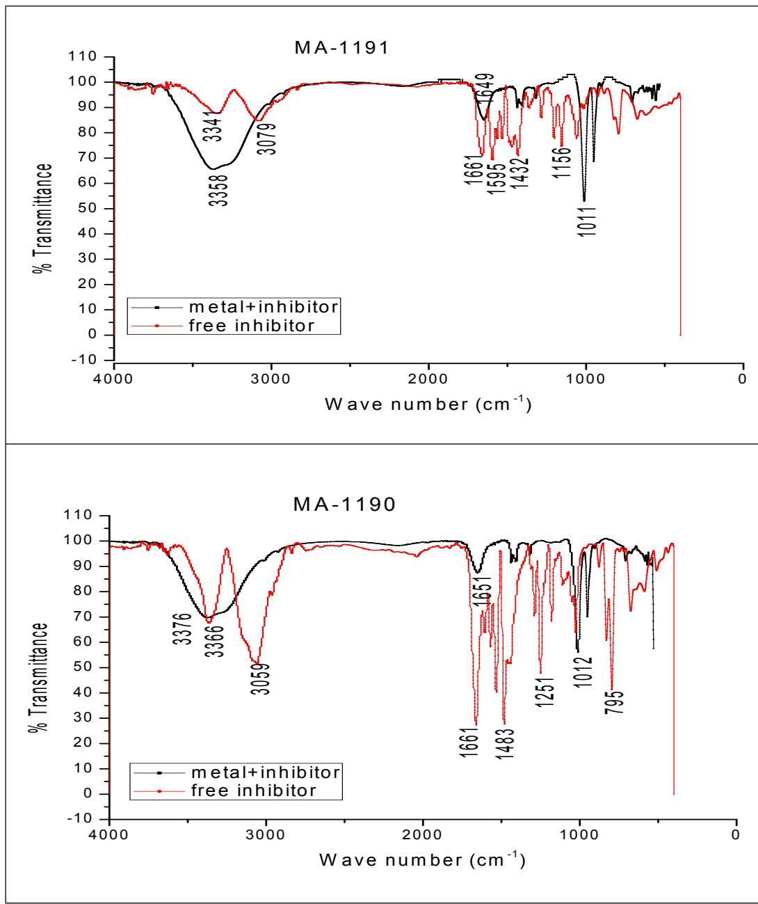
**Fig. S8.** shows FT-IR spectra for free inhibitors and inhibitors with metal for (MA-1191, MA-1190) inhibitors.
