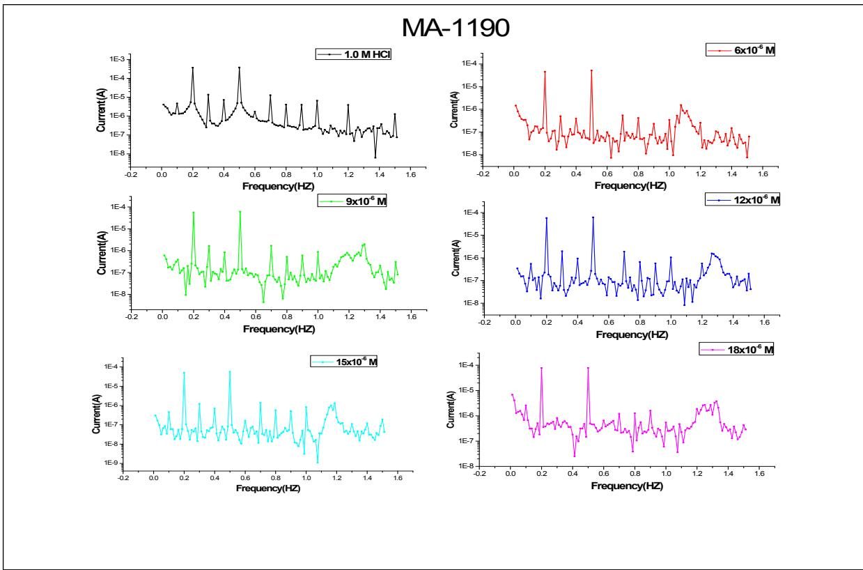
**Fig. S6.** EFM spectra for corrosion of CS in 1.0 M HCl with out and with various concentrations of MA-1191 and MA-1190 at 25°C.
