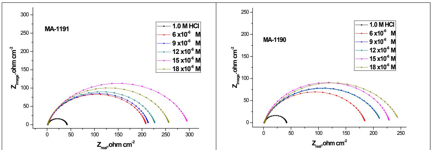
**Fig. 4.** Nyquist plots for CS in 1.0 M HCl in without and with different concentrations of (MA-1191, MA-1190) at 25°C.
