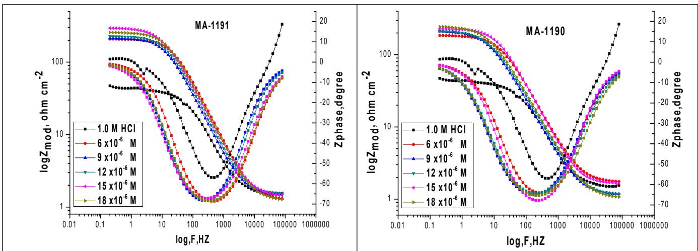
**Fig. S5.** Bode plots for CS in 1.0 M HCl in without and with different concentrations of (MA-1191, MA-1190) at 25°C.
