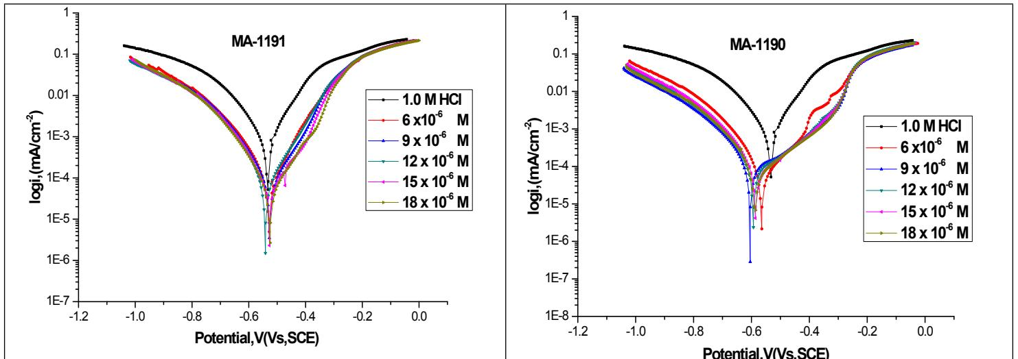
**Fig. S7.** Polarization curves for CS in 1.0 M HCl without and with various concentrations of (MA-1191, MA-1190) at 25°C.
