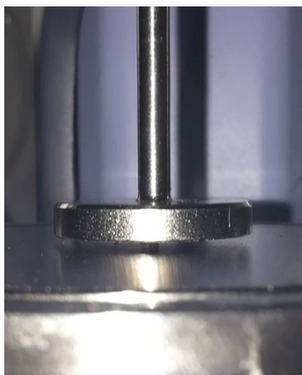
Figure S1. The experimental instrument of measuring mechanical strength of fertilizers.
