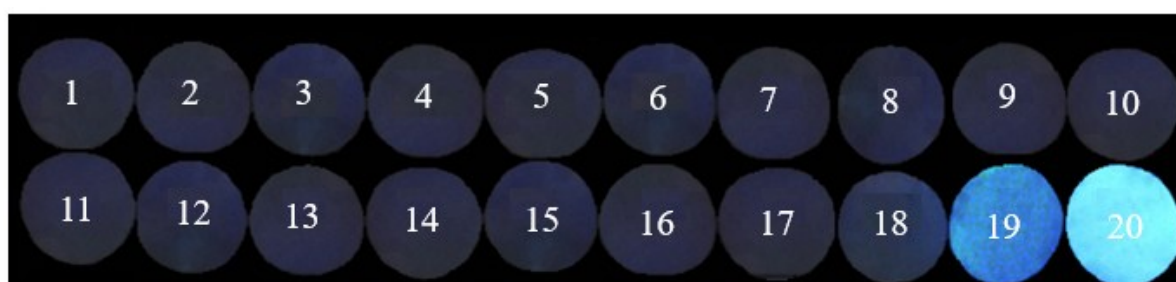
Figure S13. Fluorescence changes in test paper (under a 365 nm UV lamp) with probe BTNA upon addition of some representative analytes (1. none, 2. Ala, 3. Arg, 4. Asn, 5. Asp, 6. Gln, 7. Glu, 8. His, 9. HIE, 10. Leu, 11. Lys, 12. Met, 13. Phe, 14. Pro, 15. Ser, 16. Trp, 17. Tyr, 18. GSH, 19. Hcy, 20. Cys. Except GSH were used 1mM, others were used 200 \mu\text{M} for the test).
