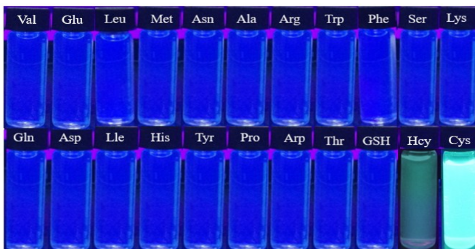
Figure S8. Emission color changes of probe BTNA with various analytes.
