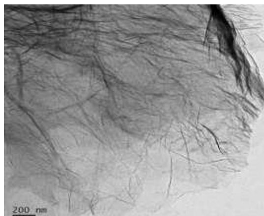
Figure S2. TEM image of reduced graphene oxide
