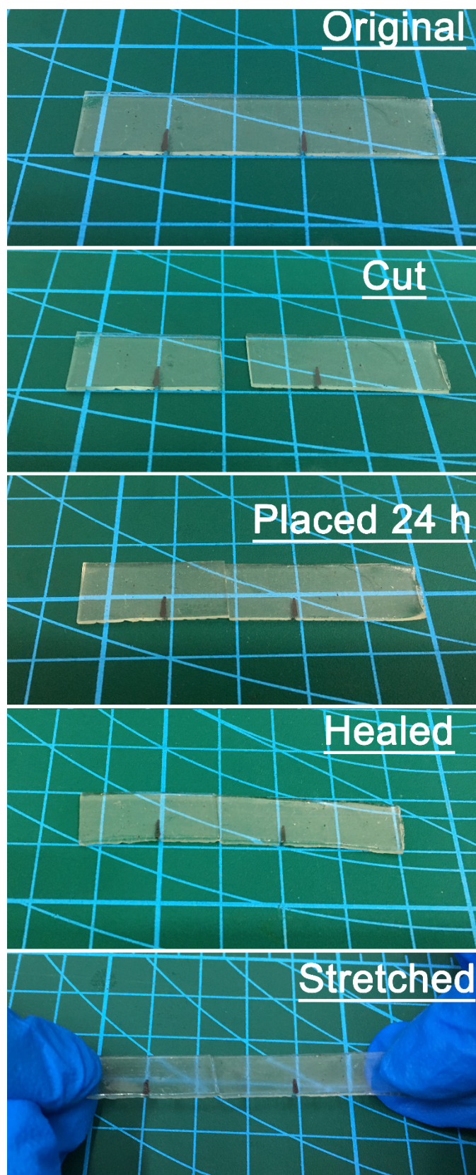
Figure S1. Digital photos shows the self-healing of Al(III)-CPDMS.
