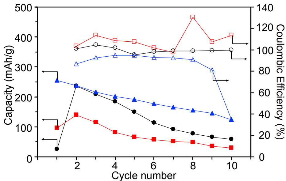
**Fig. S8** Cycle performance of the Q-TTF-Q/M (M = Li, Na and K) half cells.
