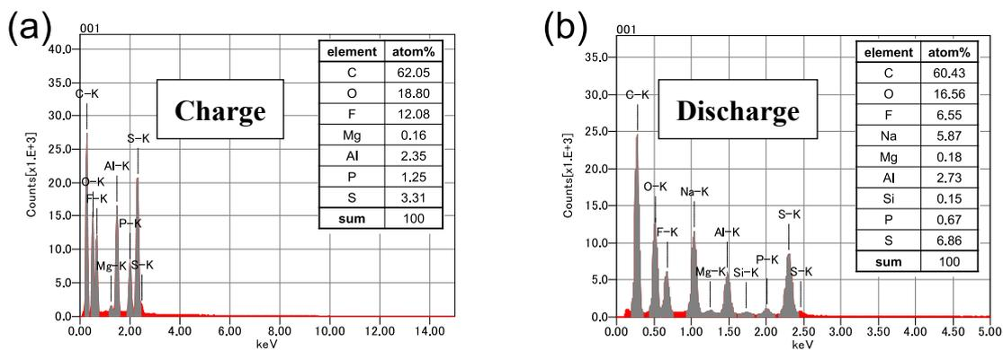
**Fig. S3** EDX analysis of the Q-TTF-Q/Na half cells.
