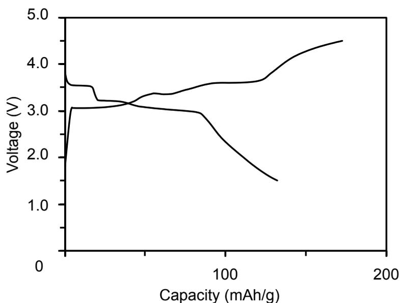
**Fig. S1** Charge and discharge curves of the TTF electrode in the 1.0 mol/L  $\text{LiPF}_6/(\text{EC}/\text{DEC}=1/5)$  solution.
