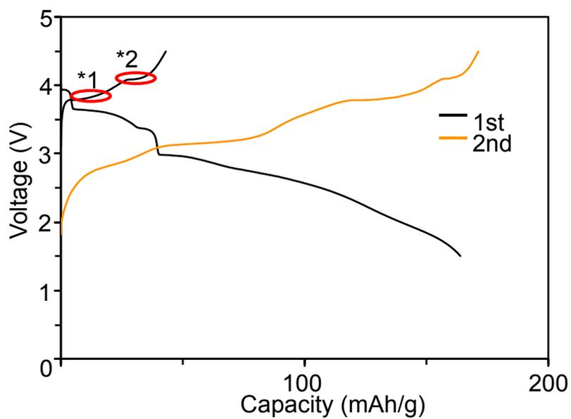
**Fig. S7** Initial charge/discharge curves of the QTTFQ/Li cell initiated by the charge process. The marked plateau potential values of 3.7(\*1) and 4.1(\*2) V vs.  $\text{Li}^+/\text{Li}$  agree with the reported values for TTF, suggesting the anion insertion reaction to the TTF moiety at these potentials.
