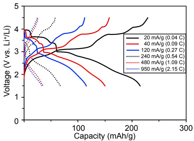
**Fig. S10** Rate performance of the Q-TTF-Q/Li half cells.
