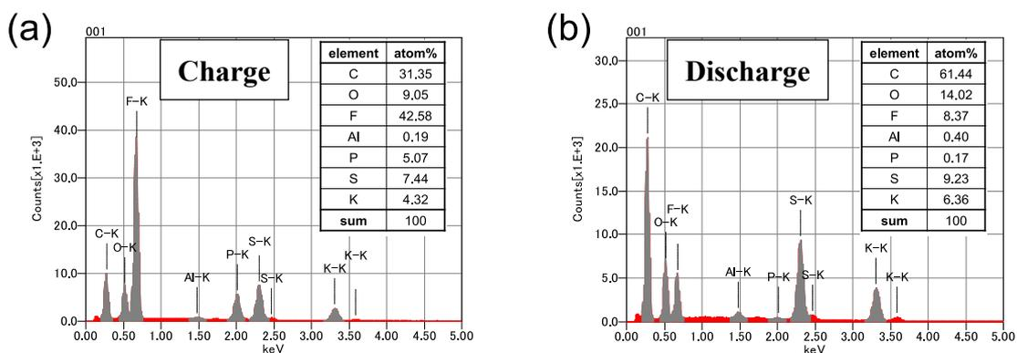
**Fig. S4** EDX analysis of the Q-TTF-Q/K half cells.
