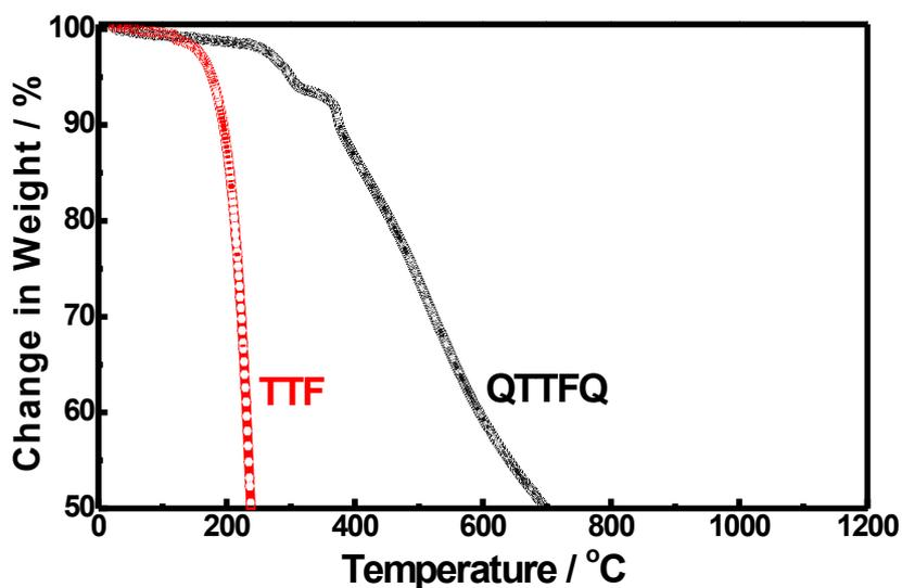
**Fig. S5** Thermogravimetric analysis (TGA) of Q-TTF-Q and TTF at 5°C/min under an Ar atmosphere.
