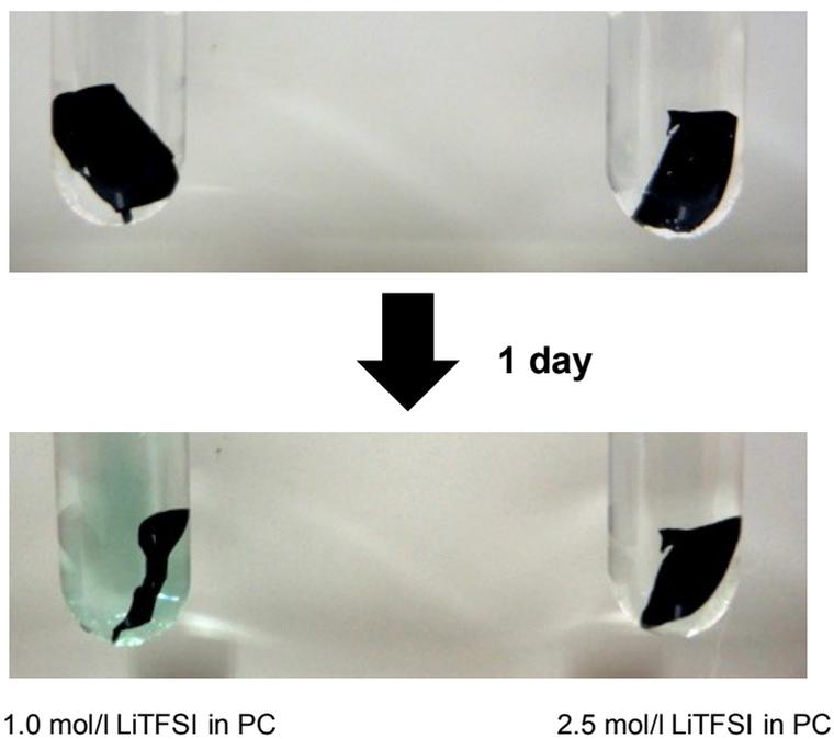
**Fig. S9** Dissolution test of the Q-TTF-Q electrodes. In this test, two types of the electrolyte solutions (1.0 mol/L LiTFSI in PC, 2.5 mol/L LiTFSI in PC) to examine the concentration effect of the electrolyte salt.
