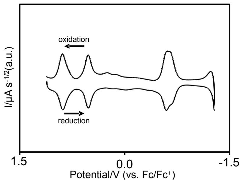
**Fig. S6** Deconvoluted cyclic voltammogram of Q-TTF-Q in the acetonitrile solution containing 0.1 mol/L  $\text{Bu}_4\text{NPF}_6$ ; scan rate is  $50 \text{ mV s}^{-1}$ .
