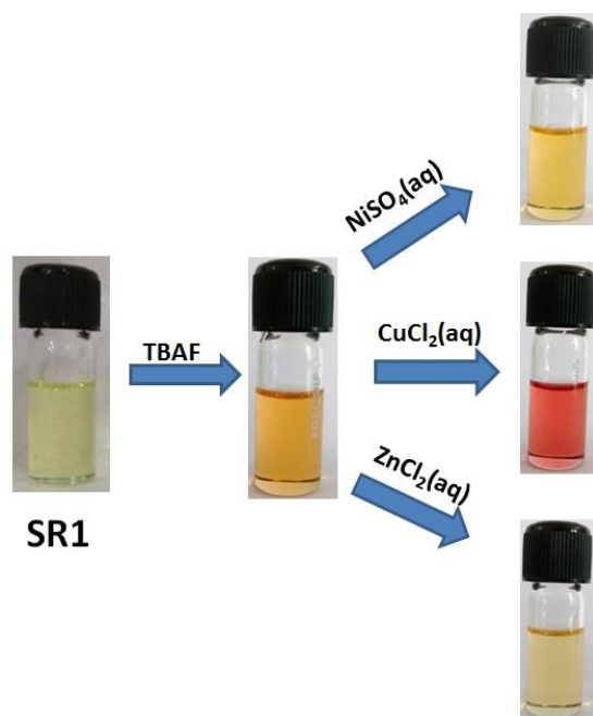
Figure S14: Schematic representation of the colorimetric change upon addition of aqueous solution of CuCl 2 , ZnCl 2 and NiSO 4 .6H 2 O of same concentration 15.4 \times 10^{-5} \text{ M} to the SR1 .F - complex in DMSO.
